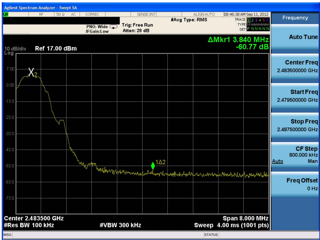
Plot 6-8. Band Edge Plot (Bluetooth (LE) – Ch. 39)
