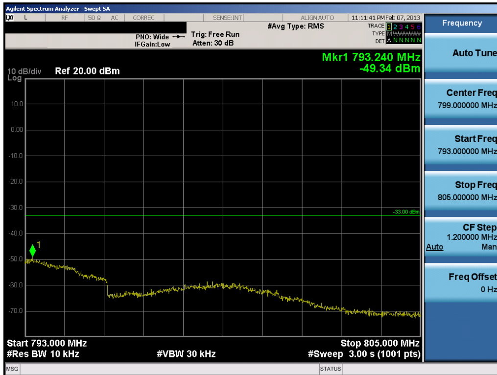
Plot 7-8. Upper Emission Mask Plot (10.0MHz QPSK – RB Size 50)
