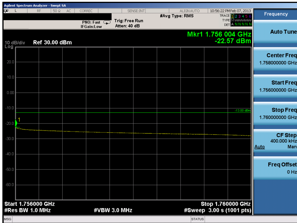
Plot 8-26. Upper Extended Band Edge Plot (10.0MHz QPSK – RB Size 50)
