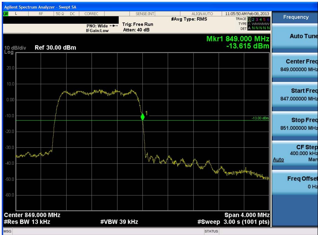
Plot 7-32. Band Edge Plot (Cellular CDMA Mode – Ch. 777)
