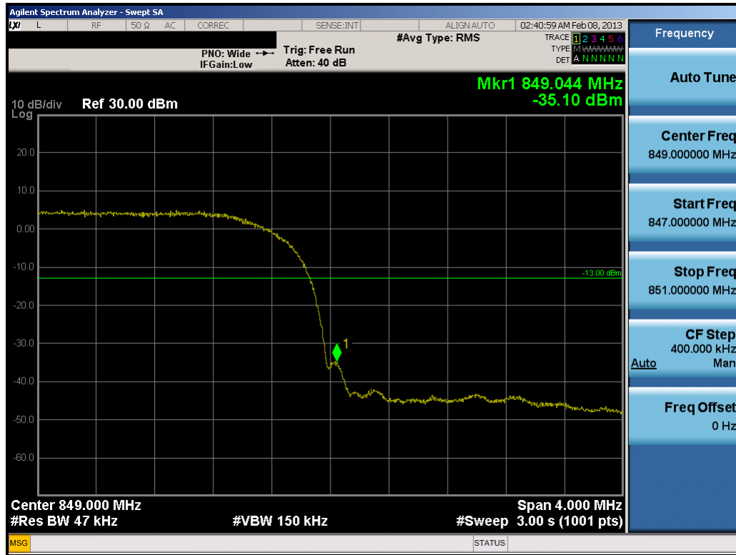
Plot 7-55. Band Edge Plot (Cellular WCDMA Mode – Ch. 4233)
