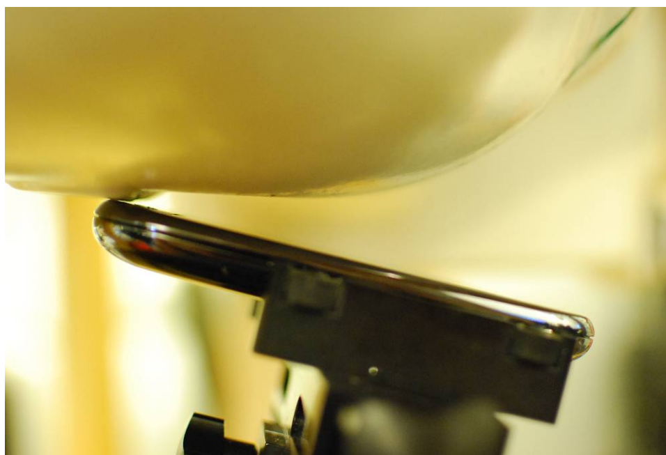
SAR Test Setup Photo 2 – Right Tilt
