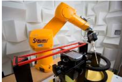
Figure 5-5 SPEAG Robotic System
