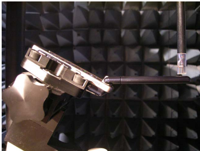
Figure 13-2 Test Setup for Wireless Device
