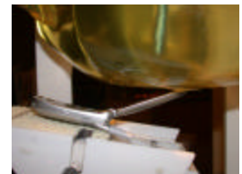
Figure A.4 Left Head SAR Test Setup -- Ear / 15° Tilt Position --
