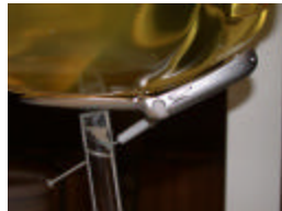
Figure A.9 Right Head SAR Test Setup -- Cheek / Touch Position --
