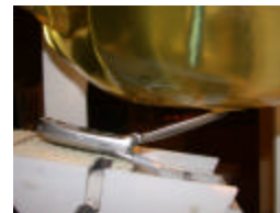
Figure A.8 Left Head SAR Test Setup -- Ear / 15° Tilt Position --
