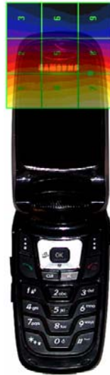
Figure 28 Sample H-field Scan Overlay
