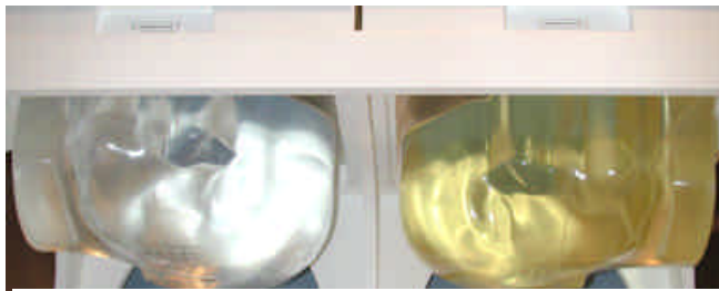
Figure 7.1 Left and Right SAM Phantom shells
