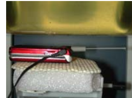
Figure 14.5 Body SAR Test Setup -- w/o Holster --
