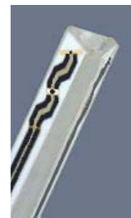
Figure 3.2 Probe Thick-Film Technique
