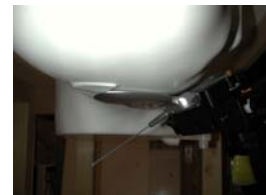
Figure 14.4 Right Head SAR Test Setup -- Cheek / Touch Position --
