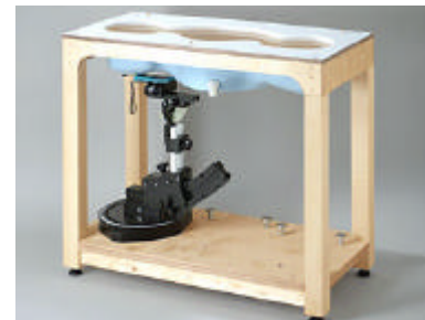
Fig. 8 Generic Twin Phantom
