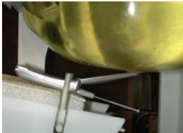
Figure 14.6 Left Head SAR Test Setup -- Ear / 15° Tilt Position --
