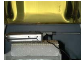
Figure 14.13 Body SAR Test Setup -- w/o Holster --
