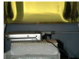
Figure 14.11 Body SAR Test Setup -- w/o Holster --
