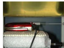
Figure 14.7 Body SAR Test Setup -- w/o Holster --
