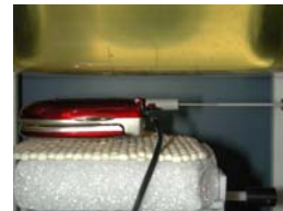
Figure 14.8 Body SAR Test Setup -- w/o Holster --
