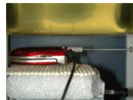
Figure 14.5 Body SAR Test Setup -- w/o Holster --
