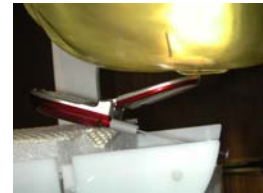
Figure 14.3 Left Head SAR Test Setup -- Ear / 15° Tilt Position --
