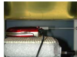
Figure 14.9 Body SAR Test Setup -- w/o Holster --
