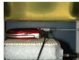
Figure 14.8 Body SAR Test Setup -- w/o Holster --
