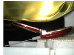
Figure 14.2 Right Head SAR Test Setup -- Ear / 15° Tilt Position --
