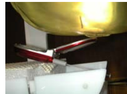
Figure 14.7 Left Head SAR Test Setup -- Ear / Tilt Position --
