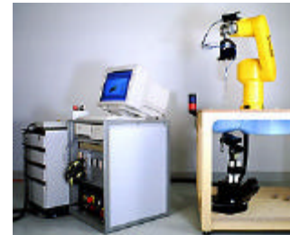
Fig. 1 SAR Test Setup
