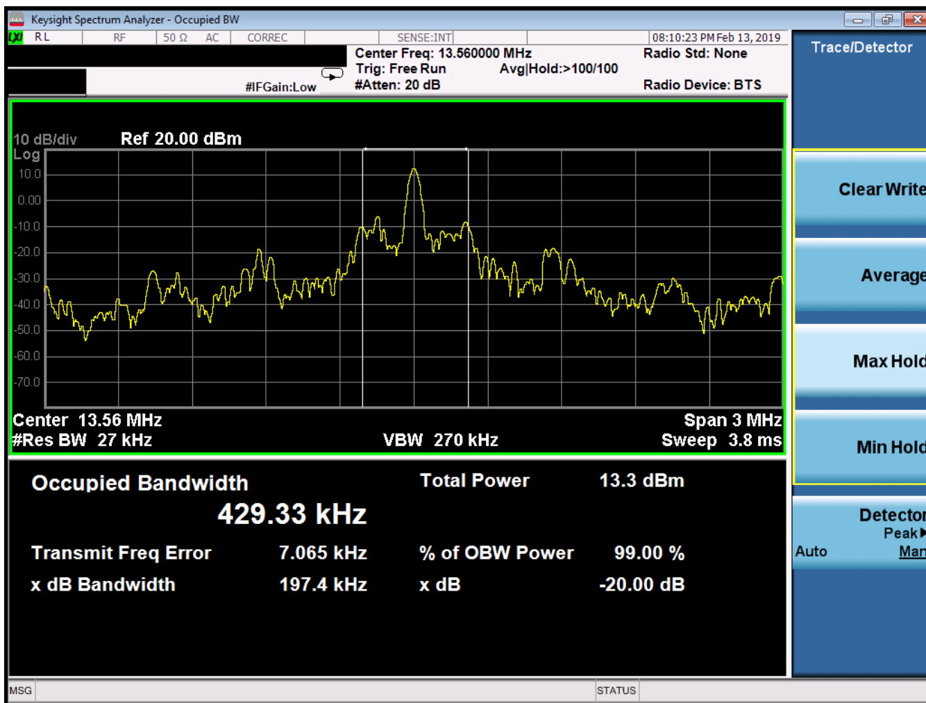
Figure 7-2. Occupied Bandwidth Plot
