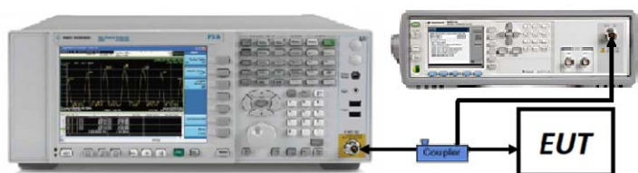
Figure 7-5. Test Instrument & Measurement Setup
