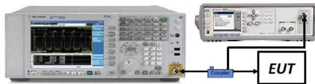
Figure 7-2. Test Instrument & Measurement Setup
