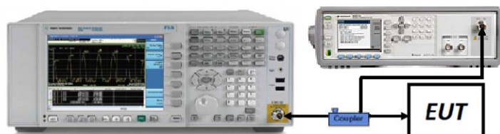
Figure 7-3. Test Instrument & Measurement Setup
