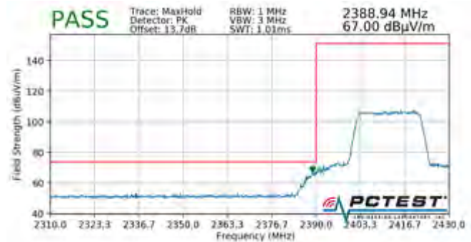
Plot 7-198. Radiated Restricted Lower Band Edge Measurement MIMO (Peak – 242 Tones)
