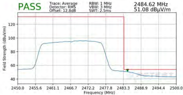
Plot 7-183. Radiated Restricted Upper Band Edge Measurement SISO ANT1 (Average – 242 Tones)
