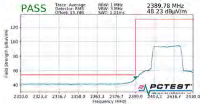
Plot 7-179. Radiated Restricted Lower Band Edge Measurement SISO ANT2 (Average – 242 Tones)
