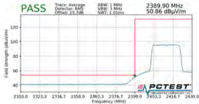
Plot 7-197. Radiated Restricted Lower Band Edge Measurement MIMO (Average – 242 Tones)
