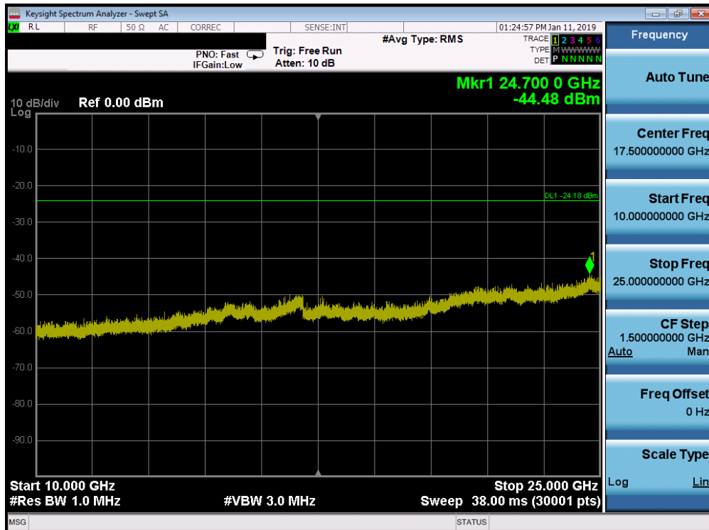
Plot 7-104. Conducted Spurious Plot SISO ANT1 (802.11ax OFDMA- 242 Tones – Ch. 11)
