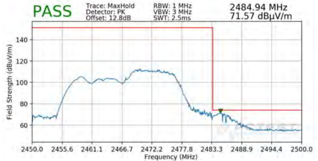
Plot 7-194. Radiated Restricted Upper Band Edge Measurement MIMO (Peak – 106 Tones)
