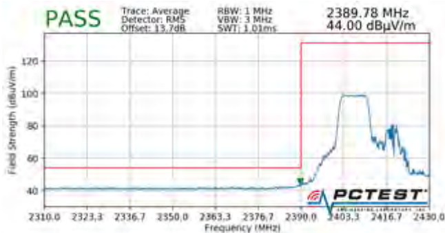
Plot 7-171. Radiated Restricted Lower Band Edge Measurement SISO ANT2 (Average – 106 Tones)
