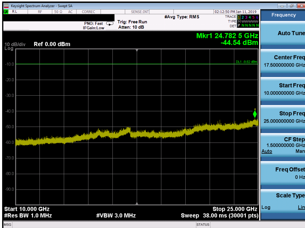
Plot 7-120. Conducted Spurious Plot SISO ANT2 (802.11ax OFDMA- 106 Tones - Ch. 6)
