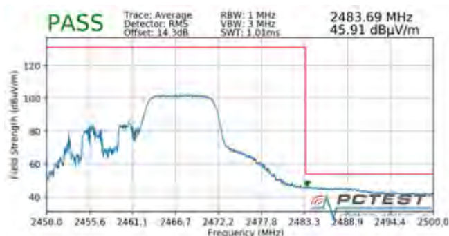
Plot 7-155. Radiated Restricted Upper Band Edge Measurement SISO ANT1 (Average – 106 Tones)
