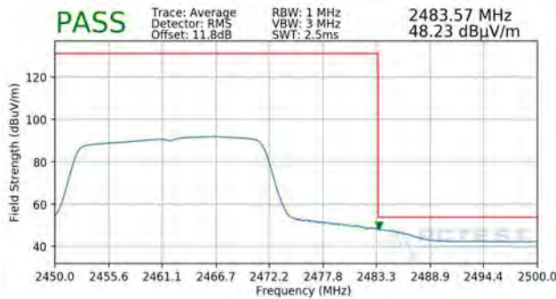
Plot 7-187. Radiated Restricted Band Edge Measurement SISO ANT2 with WCP (Average – 242 Tones)
