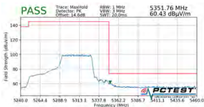
Plot 7-744. Radiated Upper Band Edge Plot SISO ANT2 (Peak – UNII Band 2A – 484 Tones)
