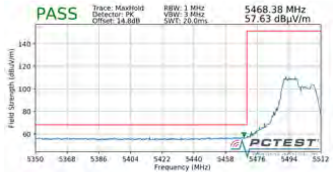
Plot 7-666. Radiated Lower Band Edge Plot SISO ANT1 (Peak - UNII Band 2C - 106 Tones)
