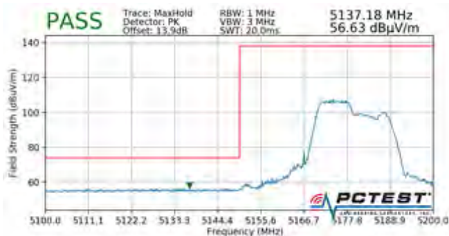
Plot 7-710. Radiated Lower Band Edge Plot SISO ANT2 (Peak – UNII Band 1 – 106 Tones)
