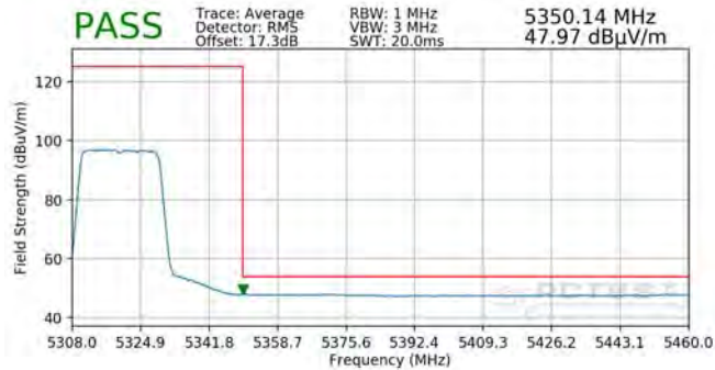
Plot 7-771. Radiated Band Edge Plot MIMO (Average – WCP – 242 Tones)
