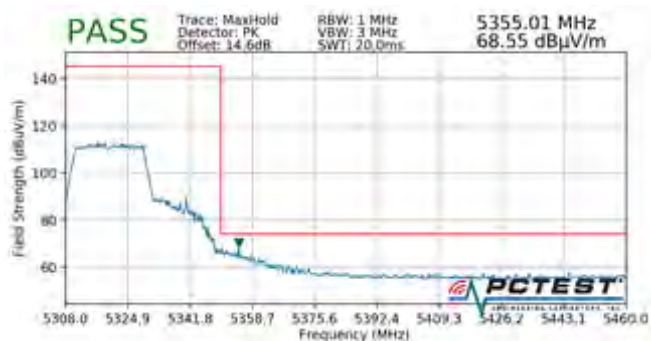
Plot 7-671. Radiated Upper Band Edge Plot SISO ANT1 (Peak – UNII Band 2A – 242 Tones)
