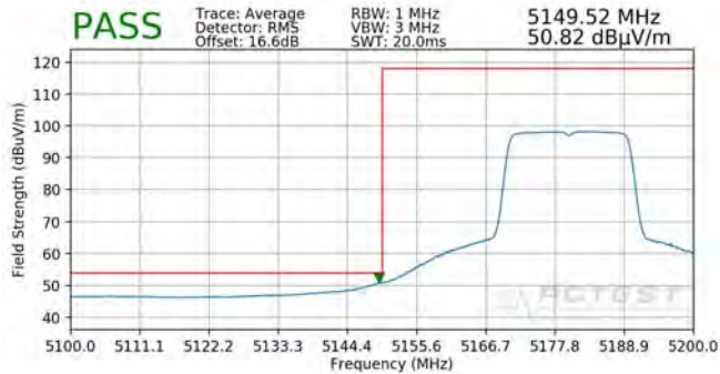
Plot 7-675. Radiated Band Edge Plot SISO ANT1 (Average – WCP – 242 Tones)
