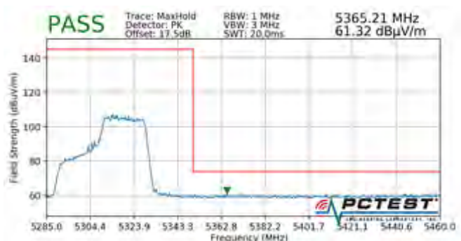
Plot 7-776. Radiated Upper Band Edge Plot MIMO (Peak – UNII Band 2A – 242 Tones)
