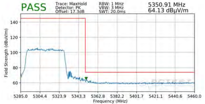
Plot 7-692. Radiated Band Edge Plot SISO ANT1 (Peak – WCP – 484 Tones)
