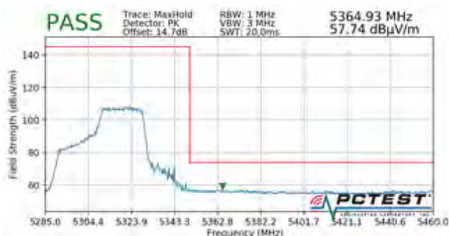
Plot 7-680. Radiated Upper Band Edge Plot SISO ANT1 (Peak – UNII Band 2A – 242 Tones)
