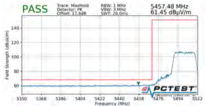
Plot 7-769. Radiated Lower Band Edge Plot MIMO (Peak – UNII Band 2C – 242 Tones)
