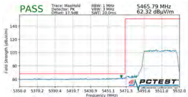
Plot 7-737. Radiated Lower Band Edge Plot SISO ANT2 (Peak – UNII Band 2C – 484 Tones)
