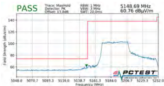
Plot 7-694. Radiated Lower Band Edge Plot SISO ANT1 (Peak – UNII Band 1 – 484 Tones)
