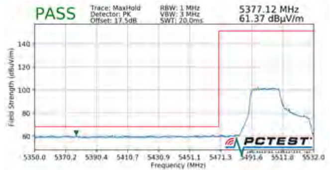
Plot 7-778. Radiated Lower Band Edge Plot MIMO (Peak – UNII Band 2C – 242 Tones)
