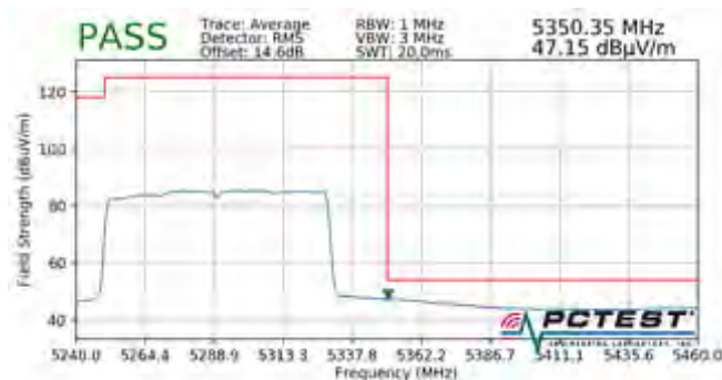
Plot 7-750. Radiated Upper Band Edge Plot SISO ANT2 (Average – UNII Band 2A – 996 Tones)
