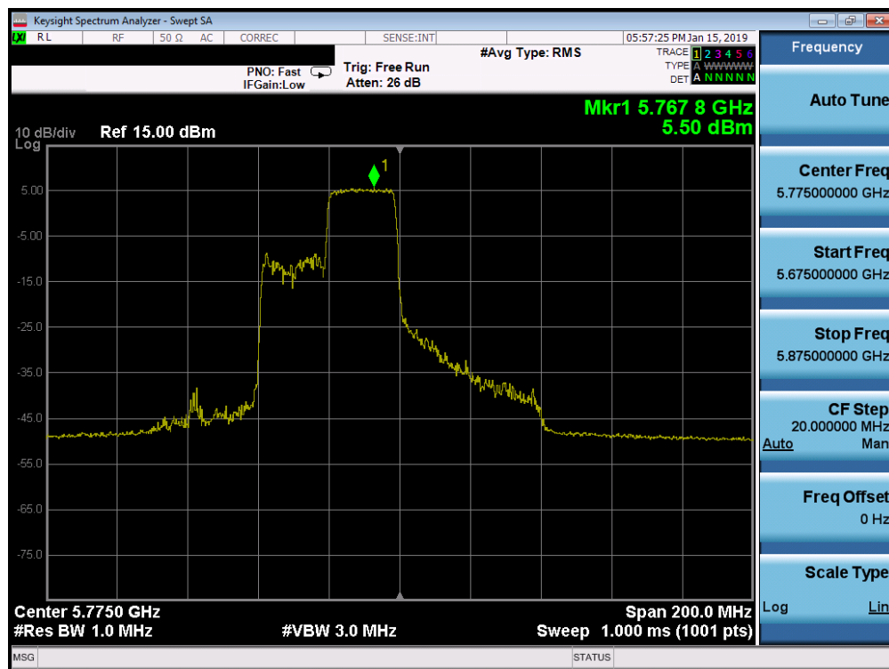
Plot 7-603. Power Spectral Density Plot MIMO ANT2 (80MHz BW 802.11ax – 242 Tones (UNII Band 3) – Ch. 155)
