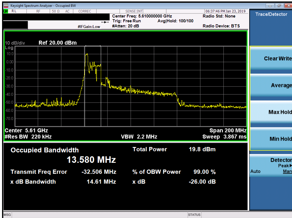
Plot 7-20. 26dB Bandwidth Plot SISO ANT1 (80MHz BW 802.11ax – 26 Tones (UNII Band 2C) – Ch. 122)
