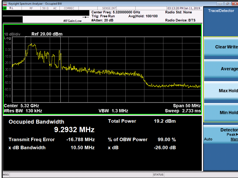
Plot 7-51. 26dB Bandwidth Plot SISO ANT2 (20MHz BW 802.11ax – 26 Tones (UNII Band 2A) – Ch. 64)
