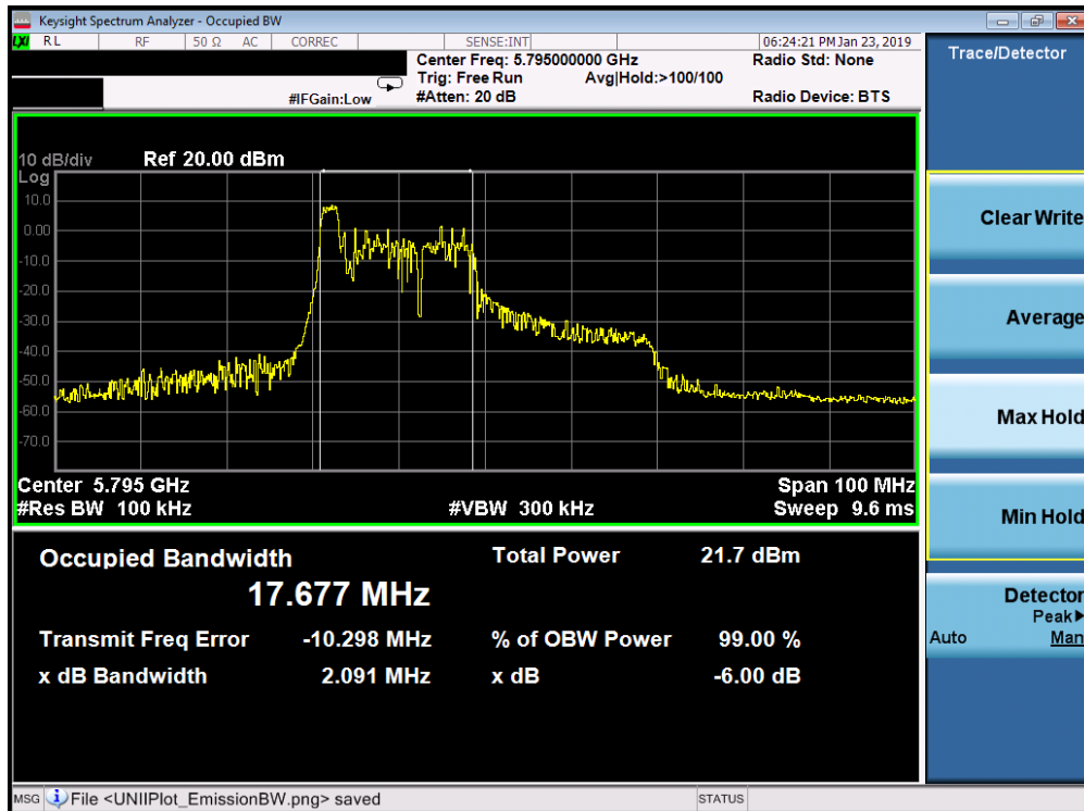
Plot 7-89. 6dB Bandwidth Plot SISO ANT1 (40MHz BW 802.11ax – 26 Tones (UNII Band 3) – Ch. 159)
