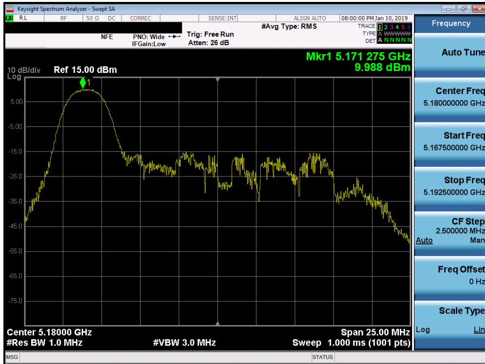
Plot 7-109. Power Spectral Density Plot SISO ANT1 (20MHz BW 802.11ax – 26 Tones (UNII Band 1) – Ch. 36)
