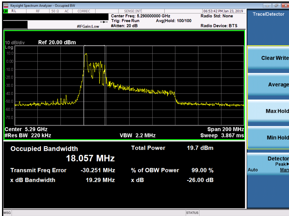
Plot 7-54. 26dB Bandwidth Plot SISO ANT2 (80MHz BW 802.11ax – 26 Tones (UNII Band 2A) – Ch. 58)
