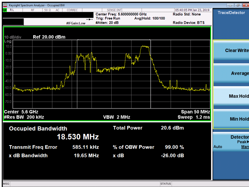
Plot 7-29. 26dB Bandwidth Plot SISO ANT1 (20MHz BW 802.11ax – 242 Tones (UNII Band 2C) – Ch. 120)
