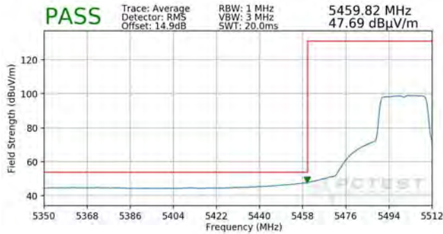
Plot 7-344. Radiated Lower Band Edge Plot MIMO (Average – UNII Band 2C)
