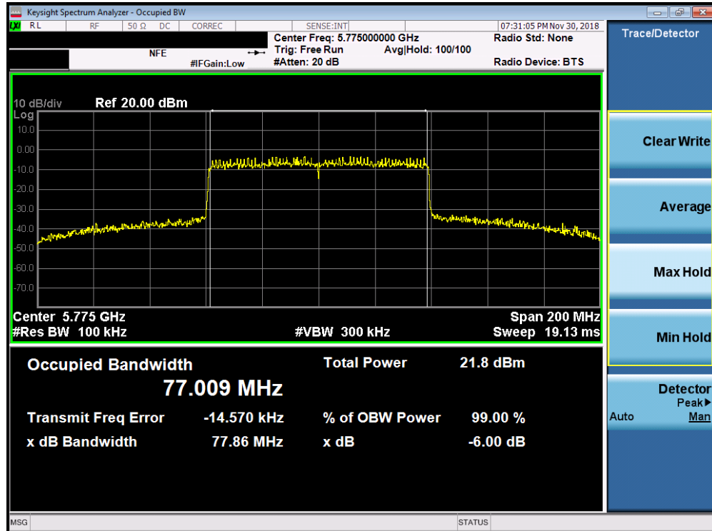
Plot 7-117. 6dB Bandwidth Plot SISO ANT1 (80MHz BW 802.11ax (UNII Band 3) – Ch. 155)
