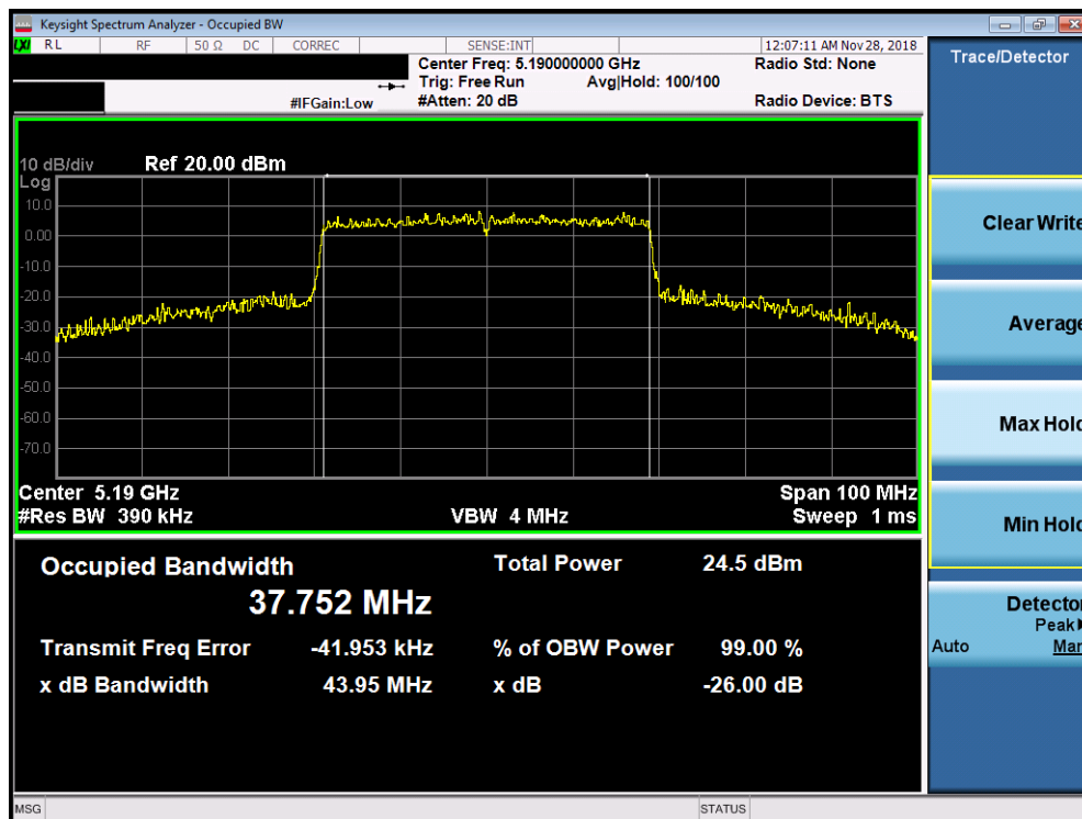
Plot 7-63. 26dB Bandwidth Plot SISO ANT2 (40MHz BW 802.11ax (UNII Band 1) – Ch. 38)
