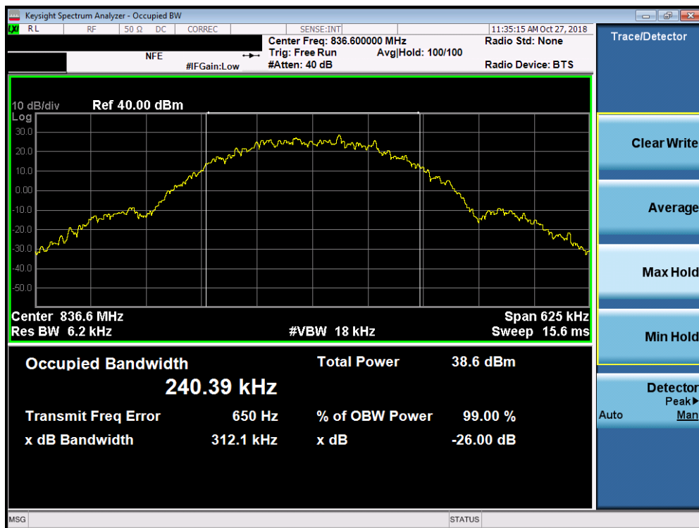
Plot 7-1. Occupied Bandwidth Plot (Cellular GPRS Mode)
