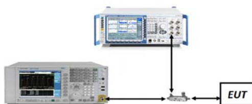
Figure 7-1. Test Instrument & Measurement Setup
