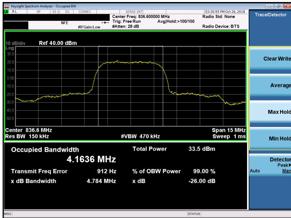
Plot 7-5. Occupied Bandwidth Plot (Cellular WCDMA Mode)
