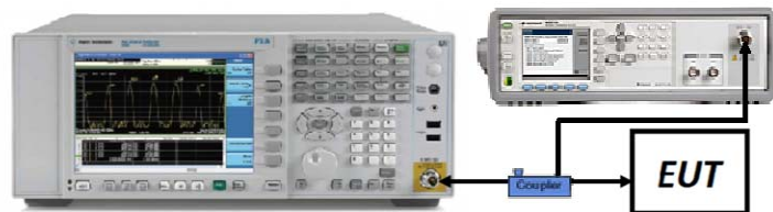
Figure 7-7. Test Instrument & Measurement Setup
