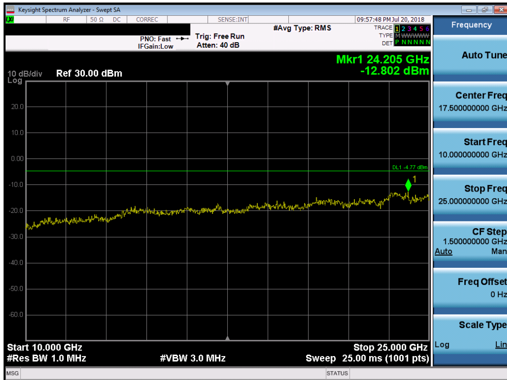
Plot 7-41. Conducted Spurious Plot (Bluetooth, 1Mbps – Ch. 78)
