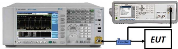
Figure 7-4. Test Instrument & Measurement Setup
