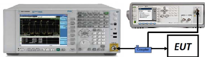
Figure 7-1. Test Instrument & Measurement Setup
