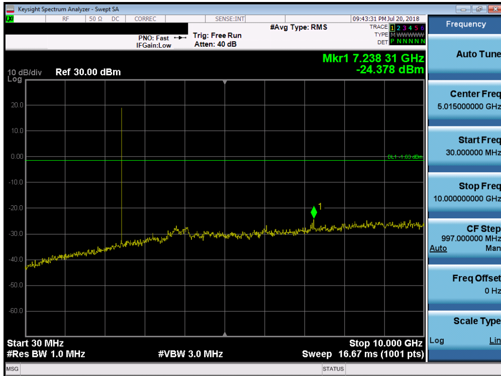
Plot 7-38. Conducted Spurious Plot (Bluetooth, 1Mbps – Ch. 39)
