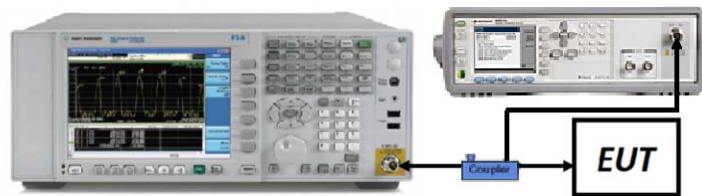
Figure 7-6. Test Instrument & Measurement Setup
