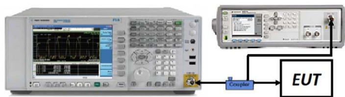
Figure 7-5. Test Instrument & Measurement Setup
