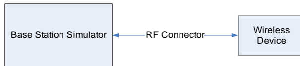
Figure 9-1 Power Measurement Setup
