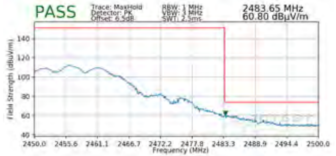
Plot 7-114. Radiated Restricted Upper Band Edge Measurement CDD (Peak)
