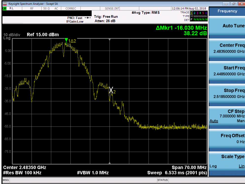
Plot 7-51. Band Edge Plot SISO ANT2 (802.11b – Ch. 12)
