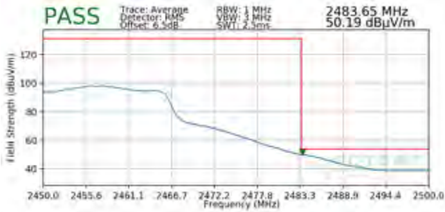
Plot 7-99. Radiated Restricted Upper Band Edge Measurement SISO ANT2 (Average)
