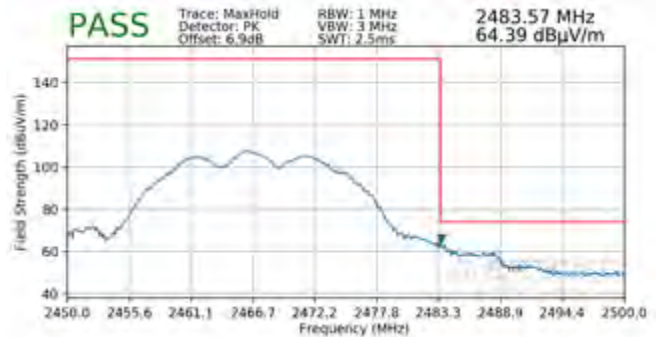
Plot 7-118. Radiated Restricted Upper Band Edge Measurement CDD (Peak)
