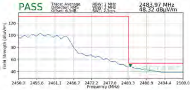
Plot 7-127. Radiated Restricted Upper Band Edge Measurement MIMO (Average)
