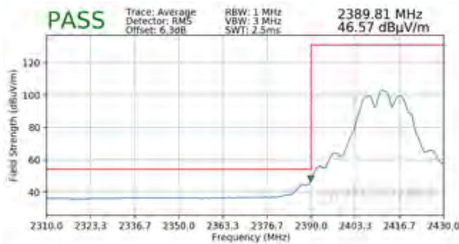
Plot 7-109. Radiated Restricted Lower Band Edge Measurement CDD (Average)
