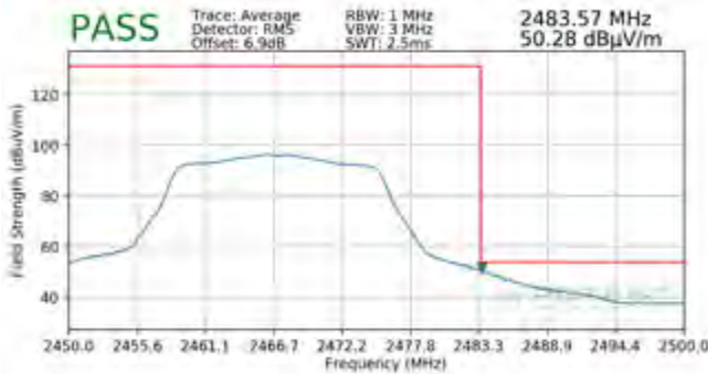
Plot 7-89. Radiated Restricted Upper Band Edge Measurement SISO ANT1 (Average)
