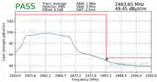
Plot 7-87. Radiated Restricted Upper Band Edge Measurement SISO ANT1 (Average)
