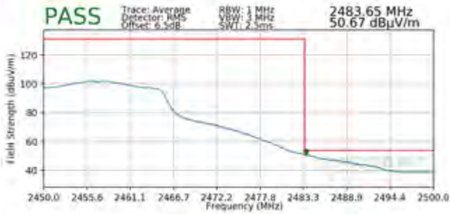
Plot 7-85. Radiated Restricted Upper Band Edge Measurement SISO ANT1 (Average)
