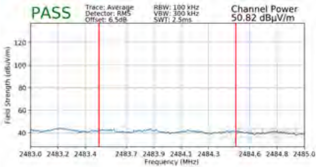
Plot 7-129. Radiated Restricted Upper Band Edge Measurement MIMO (Average)
