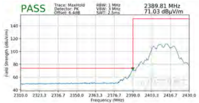
Plot 7-110. Radiated Restricted Lower Band Edge Measurement CDD (Peak)
