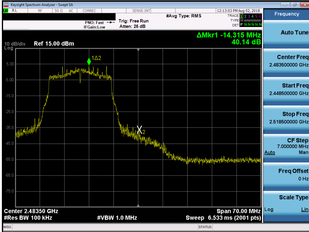
Plot 7-59. Band Edge Plot SISO ANT2 (802.11n (2.4GHz) – Ch. 12)
