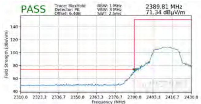
Plot 7-96. Radiated Restricted Lower Band Edge Measurement SISO ANT2 (Peak)
