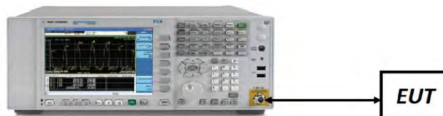
Figure 7-1. Test Instrument & Measurement Setup
