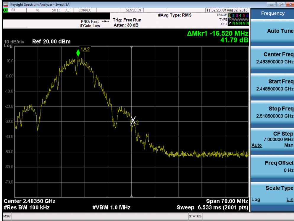
Plot 7-39. Band Edge Plot SISO ANT1 (802.11b – Ch. 12)
