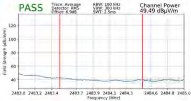
Plot 7-115. Radiated Restricted Upper Band Edge Measurement CDD (Average)
