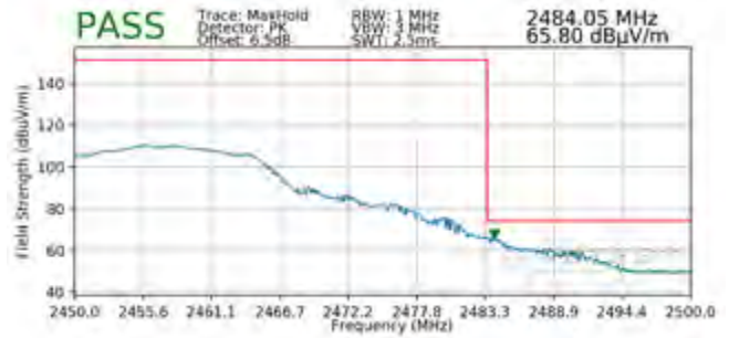
Plot 7-86. Radiated Restricted Upper Band Edge Measurement SISO ANT1 (Peak)
