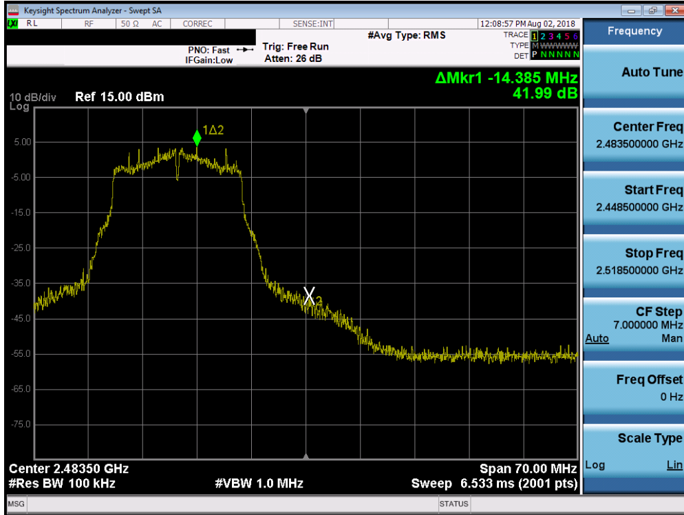
Plot 7-55. Band Edge Plot SISO ANT2 (802.11g – Ch. 12)
