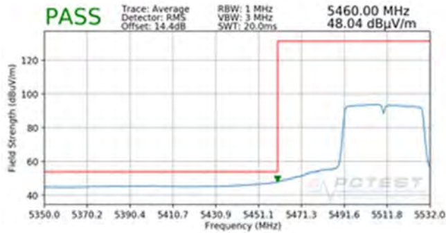
Plot 7-200. Radiated Lower Band Edge Plot SISO ANT1 (Average – UNII Band 2C)
