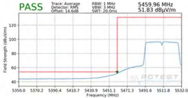
Plot 7-227. Radiated Lower Band Edge Plot SISO ANT2 (Average – UNII Band 2C)
