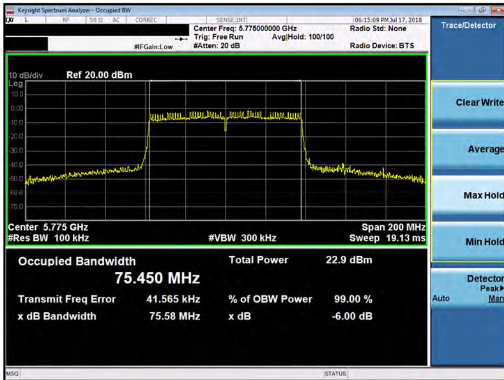
Plot 7-69. 6dB Bandwidth Plot SISO ANT1 (80MHz BW 802.11ac (UNII Band 3) – Ch. 155)
