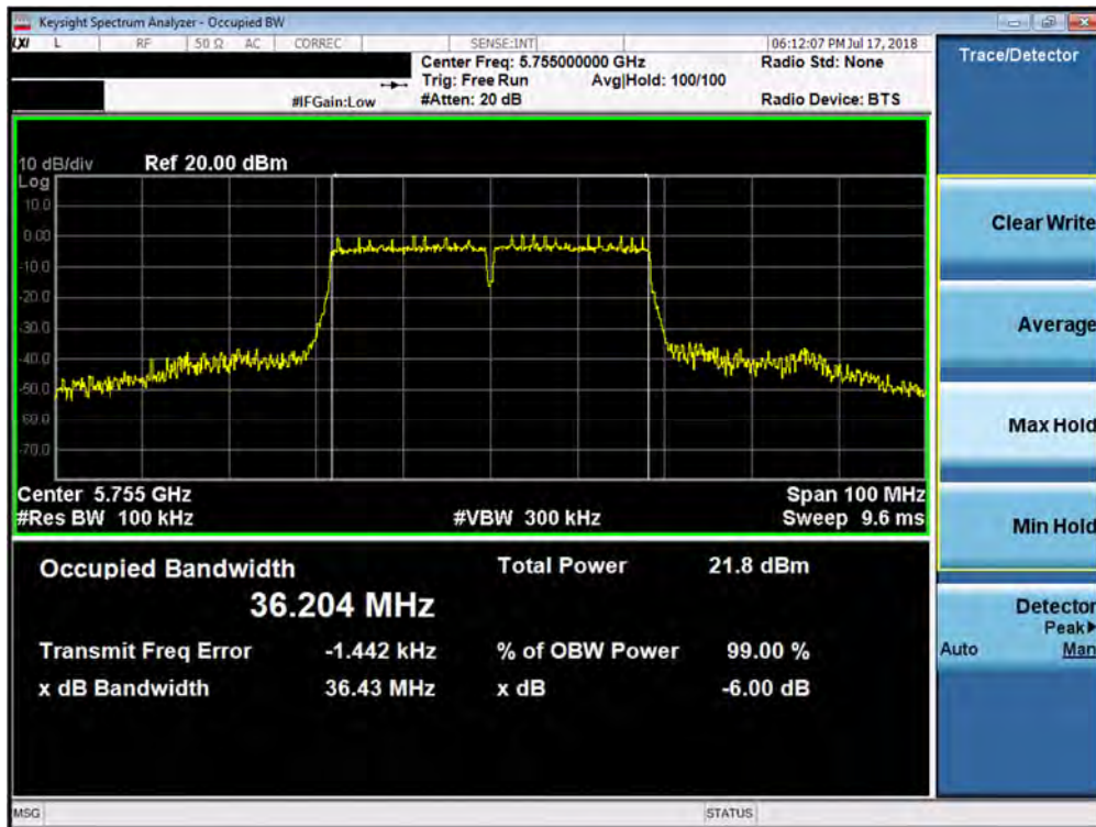
Plot 7-67. 6dB Bandwidth Plot SISO ANT1 (40MHz BW 802.11n (UNII Band 3) – Ch. 151)
