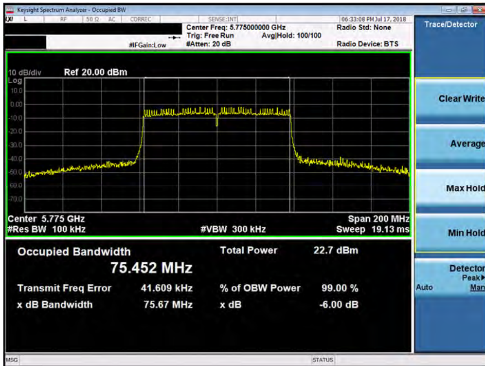
Plot 7-78. 6dB Bandwidth Plot SISO ANT2 (80MHz BW 802.11ac (UNII Band 3) – Ch. 155)
