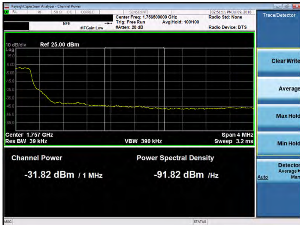
Plot 7-140. Upper Extended Band Edge Plot (Band 4 - 5.0MHz QPSK - Full RB Configuration)
