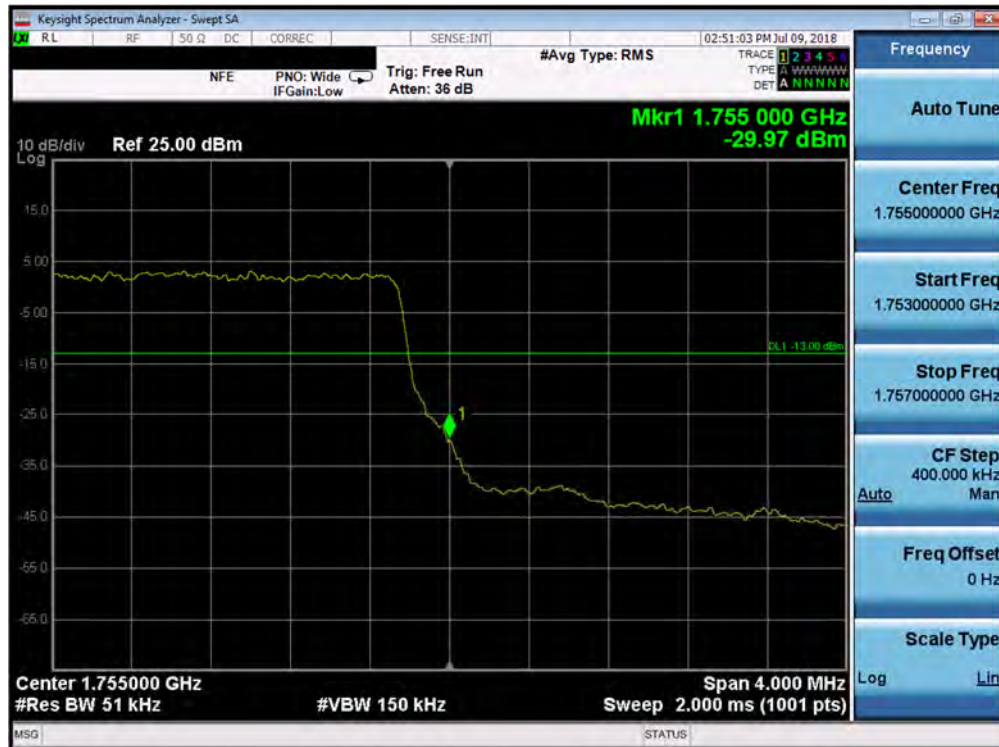
Plot 7-139. Upper Band Edge Plot (Band 4 - 5.0MHz QPSK - Full RB Configuration)
