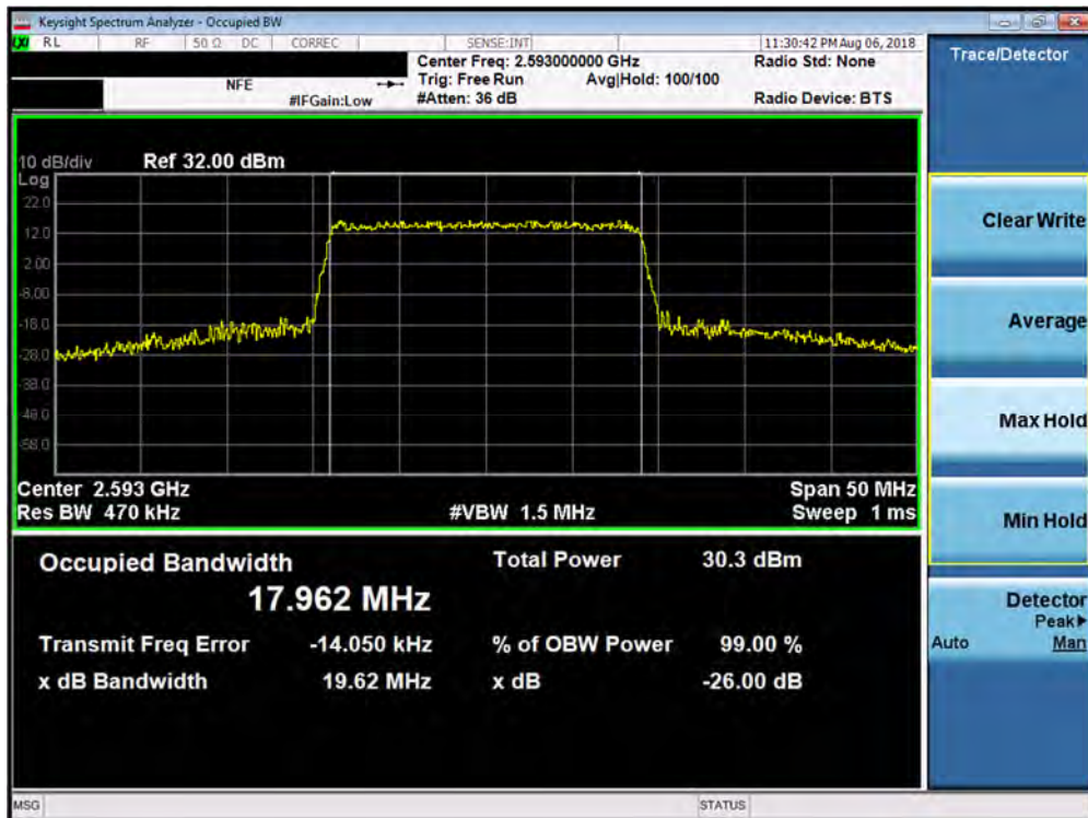
Plot 7-60. Occupied Bandwidth Plot (Band 41 - 20.0MHz 64-QAM - Full RB Configuration)
