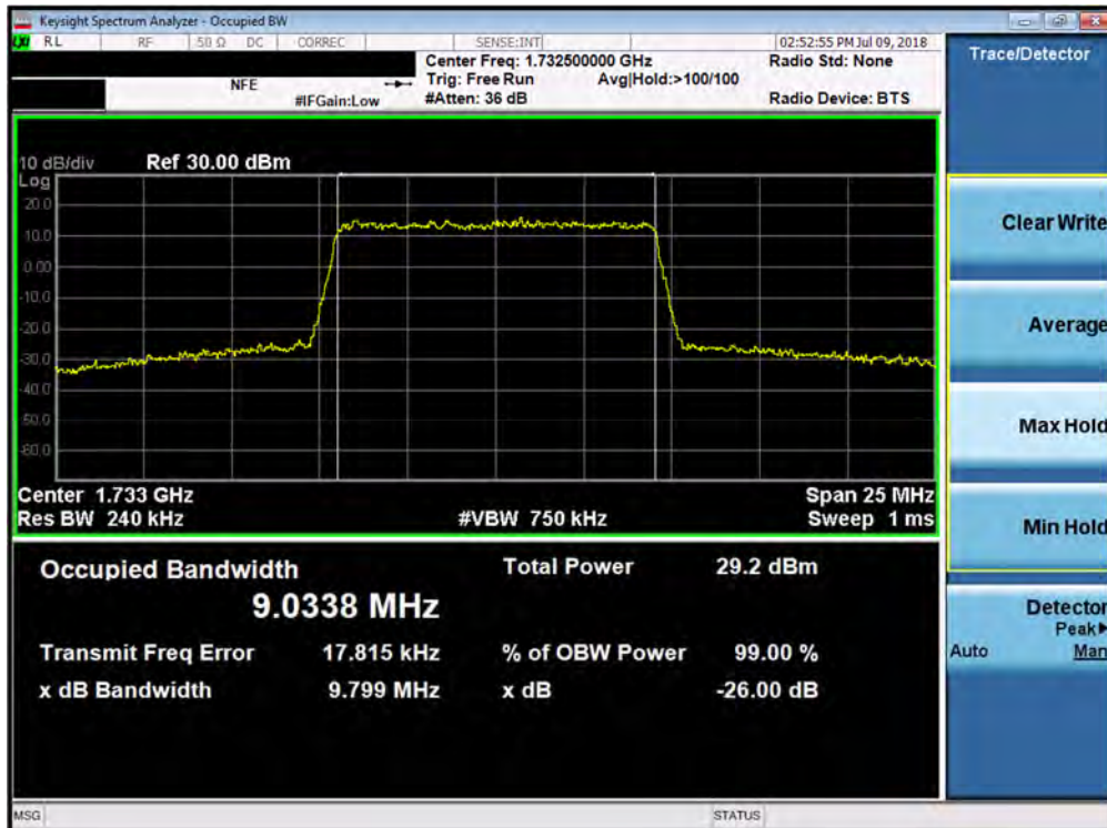
Plot 7-42. Occupied Bandwidth Plot (Band 4 - 10.0MHz 64-QAM - Full RB Configuration)
