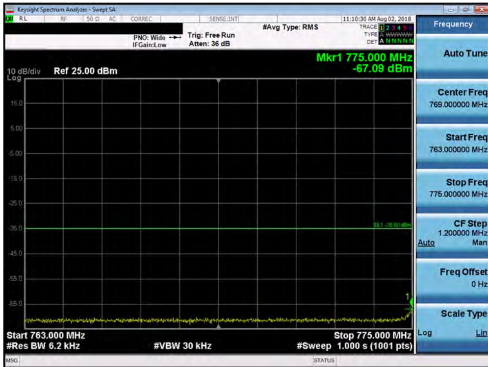
Plot 7-114. Lower Emission Mask Plot (Band 13 - 5.0MHz QPSK - Full RB Configuration)
