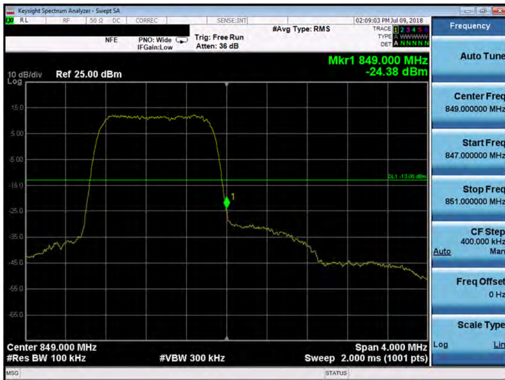
Plot 7-122. Upper Band Edge Plot (Band 5 - 1.4MHz QPSK - Full RB Configuration)
