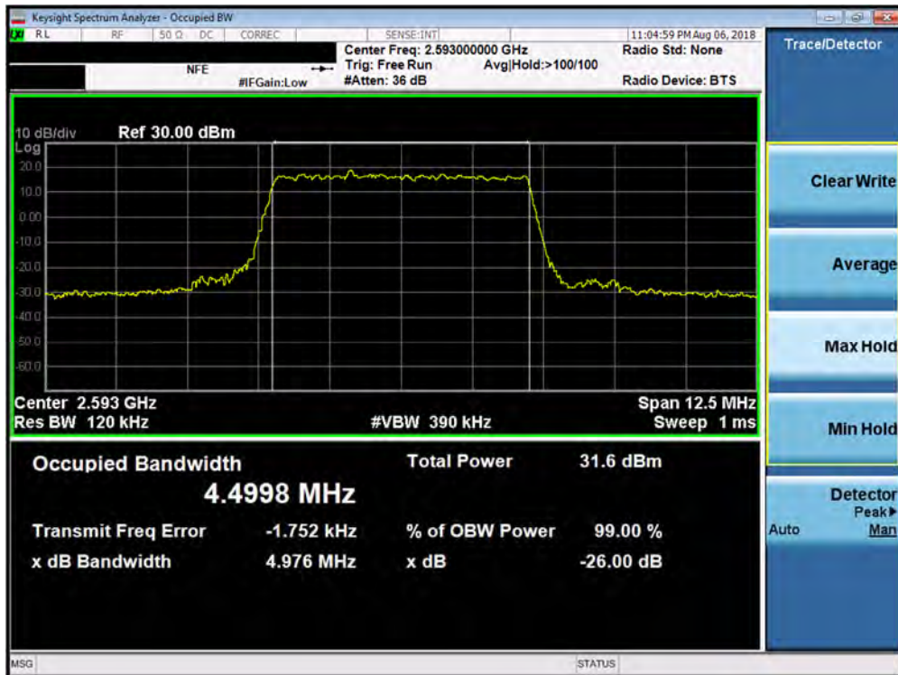
Plot 7-50. Occupied Bandwidth Plot (Band 41 - 5.0MHz 16-QAM - Full RB Configuration)
