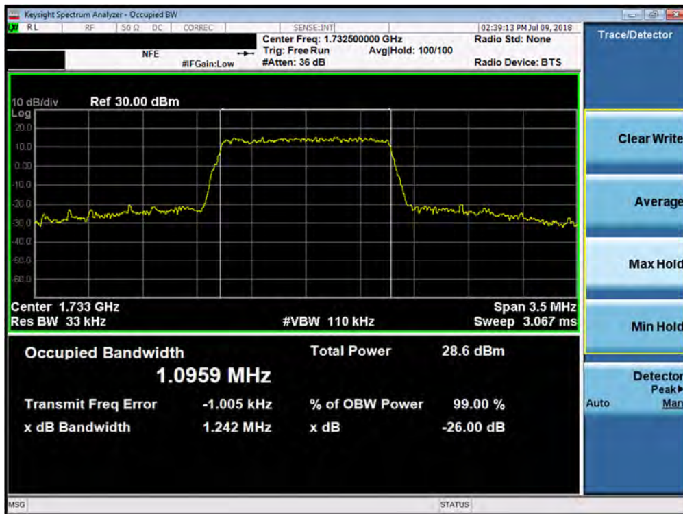
Plot 7-32. Occupied Bandwidth Plot (Band 4 - 1.4MHz 16-QAM - Full RB Configuration)
