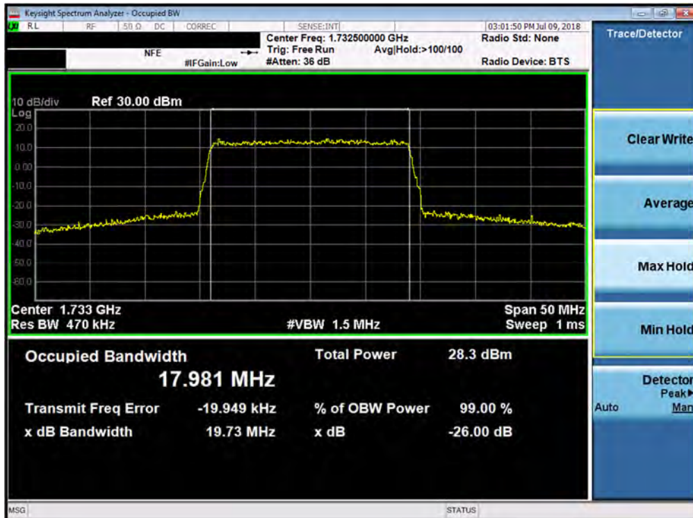
Plot 7-48. Occupied Bandwidth Plot (Band 4 - 20.0MHz 64-QAM - Full RB Configuration)
