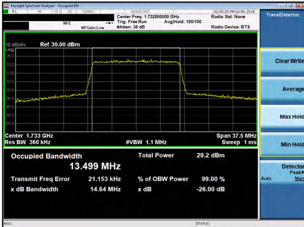
Plot 7-44. Occupied Bandwidth Plot (Band 4 - 15.0MHz 16-QAM - Full RB Configuration)
