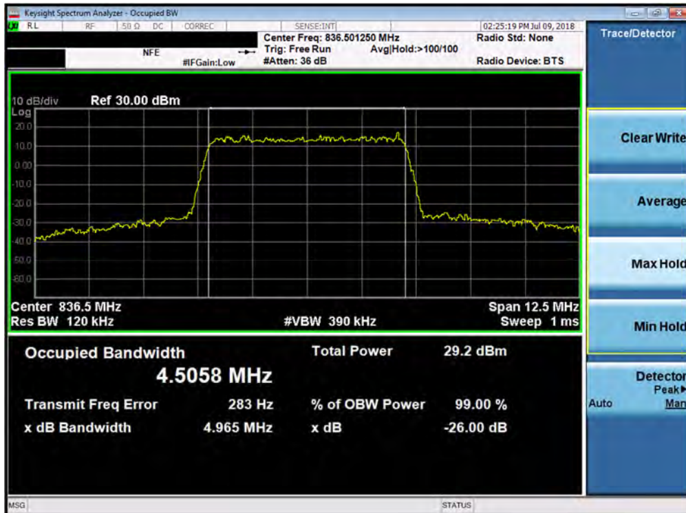
Plot 7-26. Occupied Bandwidth Plot (Band 5 - 5.0MHz 16-QAM - Full RB Configuration)
