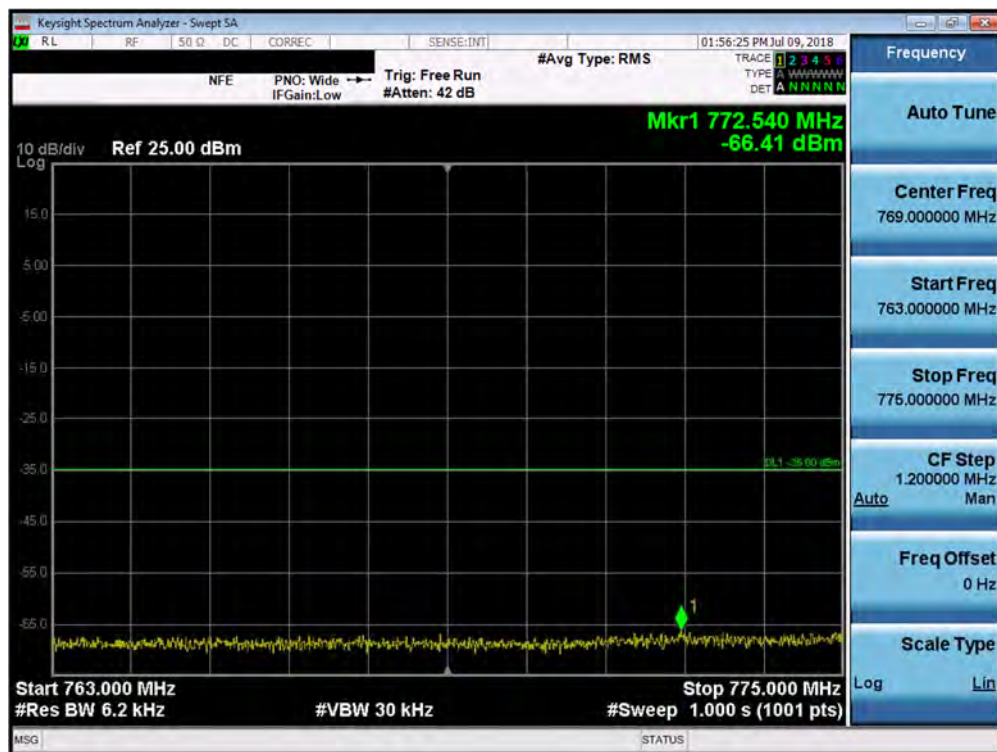
Plot 7-118. Lower Emission Mask Plot (Band 13 - 10.0MHz QPSK - Full RB Configuration)
