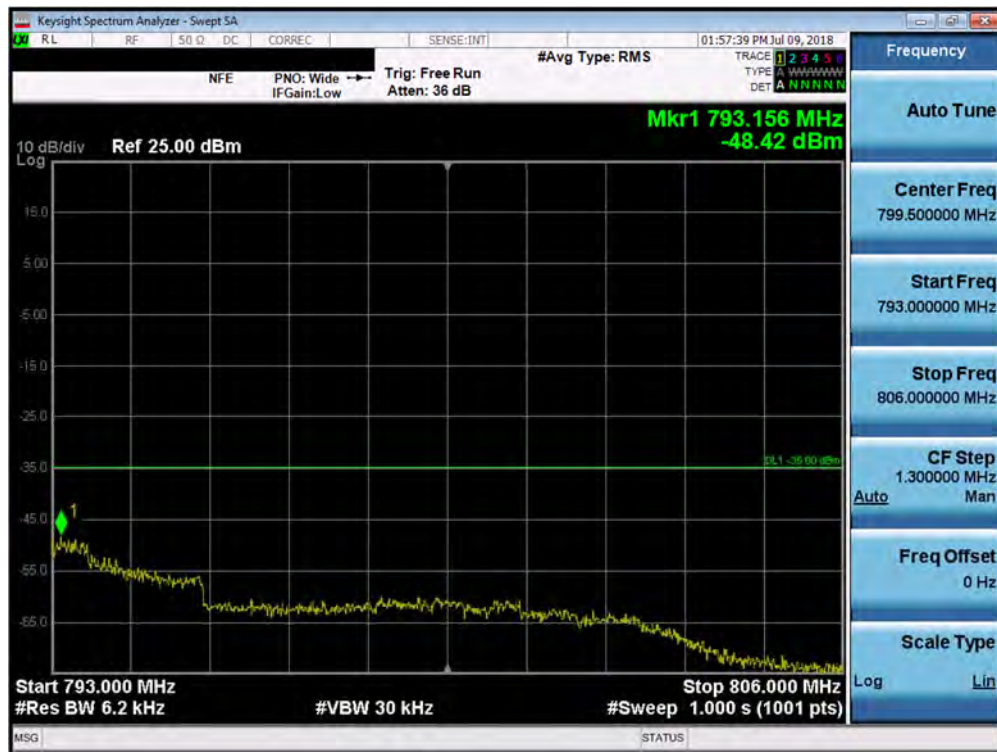
Plot 7-120. Upper Emission Mask Plot (Band 13 - 10.0MHz QPSK - Full RB Configuration)
