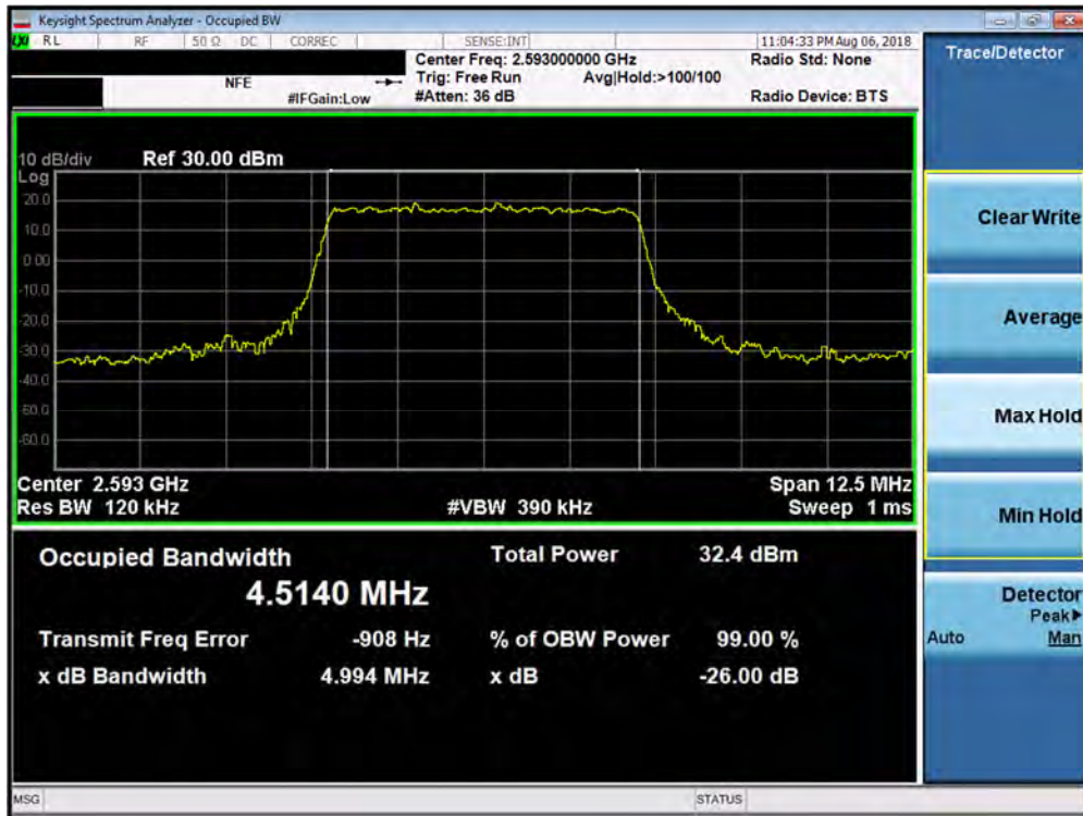
Plot 7-49. Occupied Bandwidth Plot (Band 41 - 5.0MHz QPSK - Full RB Configuration)
