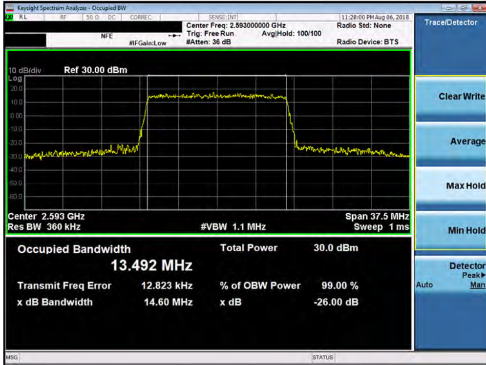
Plot 7-57. Occupied Bandwidth Plot (Band 41 - 15.0MHz 64-QAM - Full RB Configuration)
