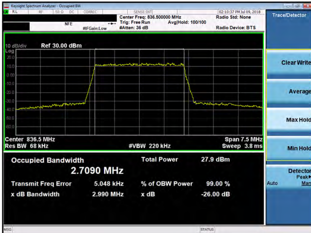
Plot 7-24. Occupied Bandwidth Plot (Band 5 - 3.0MHz 64-QAM - Full RB Configuration)
