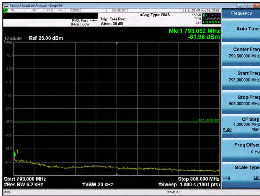
Plot 7-116. Upper Emission Mask Plot (Band 13 - 5.0MHz QPSK - Full RB Configuration)
