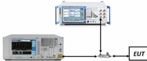
Figure 7-4. Test Instrument & Measurement Setup
