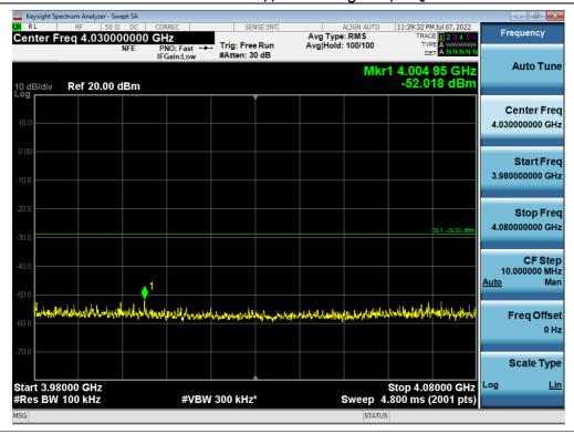
Antenna 2 / High Edge + 100 MHz ~ 10 GHz / 3.7 GHz Service 5G NR(20 MHz 1 Carrier + 20 MHz 1 Carrier) [2 Carrier] (3 700 MHz - 3 900 MHz) / Non-Contiguous / 64QAM
