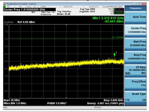
Antenna 0 / Low Edge - 100 MHz ~ Low Edge / 3.7 GHz Service 5G NR(20 MHz 1 Carrier + 20 MHz 1 Carrier) [2 Carrier] (3 700 MHz - 3 900 MHz) / Non-Contiguous / 256QAM
