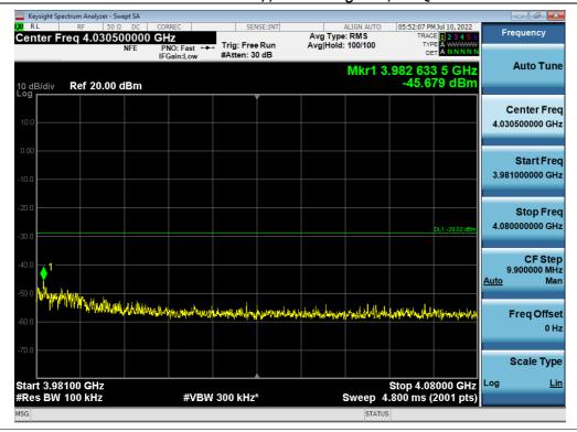
Antenna 1 / High Edge + 100 MHz ~ 10 GHz / 3.7 GHz Service 5G NR(20 MHz 1 Carrier + 20 MHz 1 Carrier) [2 Carrier] (3 780 MHz - 3 980 MHz) / Non-Contiguous / 64QAM
