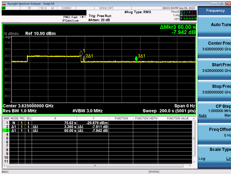
Plot 39. Conducted Measurement - RF transmission stops (WINNF.FT.C.RLQ.1) – LTE
