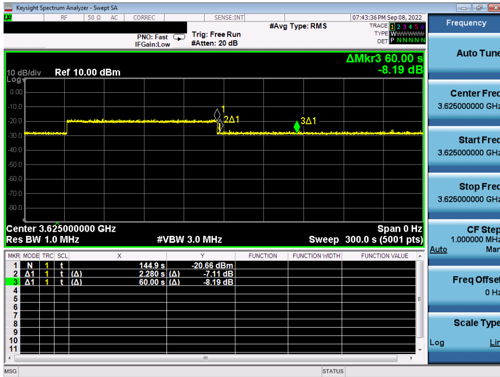
Plot 29. Conducted Measurement - RF transmission stops within 60s of SAS message. The SAS message is indicated by Marker 1 (X) (WINNF.FT.C.HBT.6) – LTE
