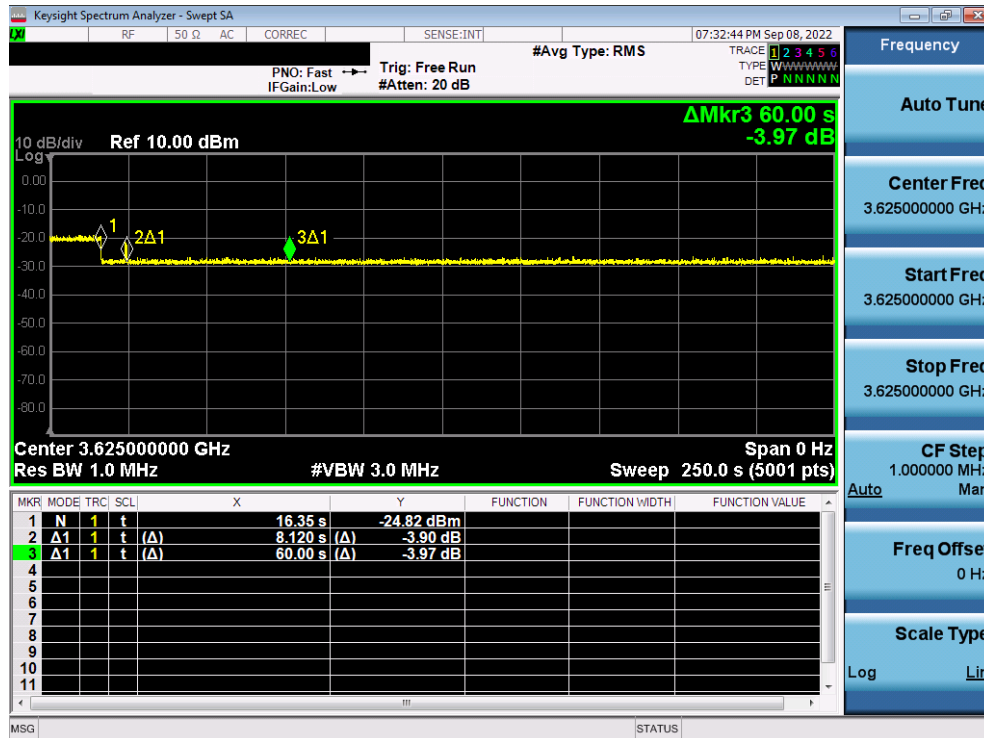
Plot 25. Conducted Measurement - RF transmission stops within 60s of SAS message indicated by Marker 1 (X) (WINNF.FT.C.HBT.4) – LTE
