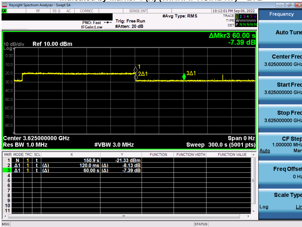
Plot 32. Conducted Measurement - RF transmission stops within 60s of SAS message. The SAS message is indicated by Marker 1 (X) (WINNF.FT.C.HBT.7) – NR
