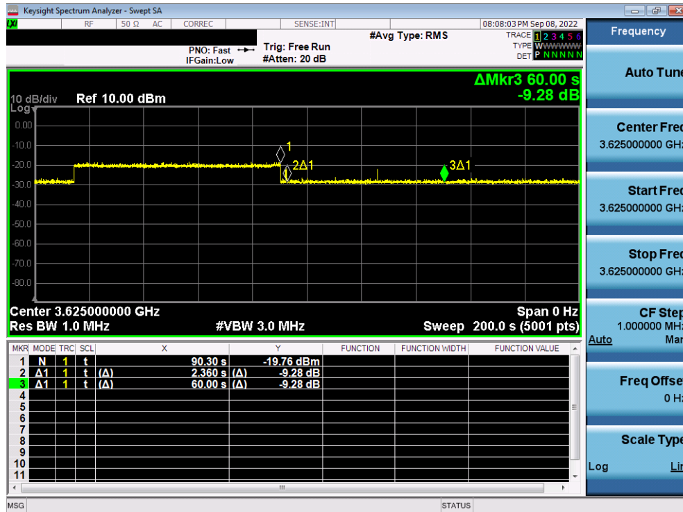
Plot 41. Conducted Measurement - RF transmission stops within 60s. The SAS message is indicated by Marker 1 (X) (WINNF.FT.C.DRG.1) – LTE
