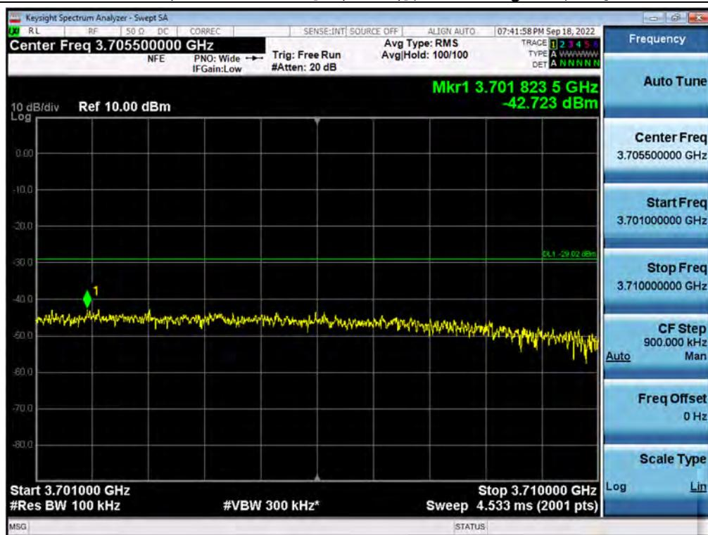
**Antenna 3 / 2<sup>nd</sup> High Edge + 10 MHz ~ 3720 MHz / CBRS (NR 40 MHz 1C + NR 20 MHz 1C + NR 20 MHz 1C + LTE 10 MHz 1C) + LTE 10 MHz 1C[5C(4C+1C)] / Non-Contiguous / QPSK**
