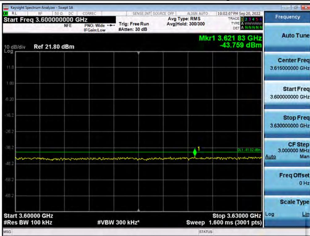
**Antenna 3 / 2<sup>nd</sup> High Edge - 10 MHz ~ 2<sup>nd</sup> High Edge - 1 MHz / CBRS NR 40 MHz 1C + (NR 20 MHz 1C + NR 20 MHz 1C + LTE 10 MHz 1C + LTE 10 MHz 1C)[5C(1C+4C)] / Non-Contiguous / QPSK**
