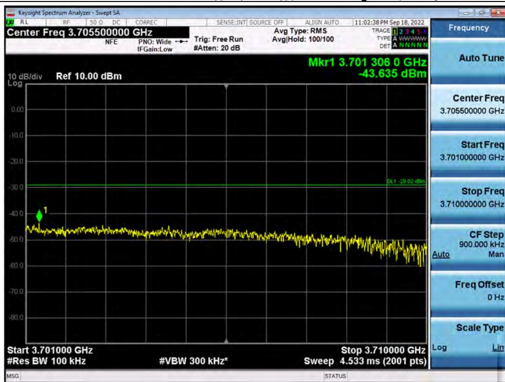
Antenna 3 / 2<sup>nd</sup> High Edge + 10 MHz ~ 3720 MHz / CBRS NR 40 MHz 1C + (NR 20 MHz 1C + NR 20 MHz 1C + LTE 10 MHz 1C + LTE 10 MHz 1C)[5C(1C+4C)] / Non-Contiguous / QPSK
