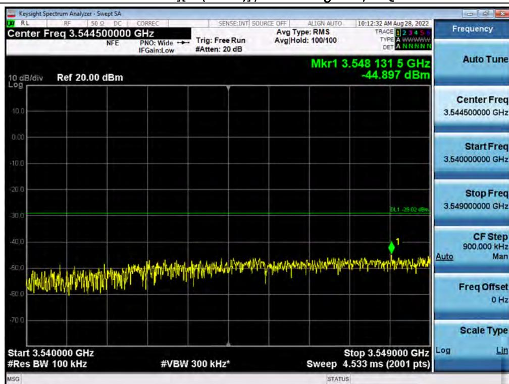
**Antenna 1 / 1<sup>st</sup> High Edge + 1 MHz ~ 1<sup>st</sup> High Edge + 10 MHz / CBRS LTE[(20 MHz 1C + 20 MHz 1C + 20 MHz 1C) + 20 MHz 1C][5C(4C+1C)] / Non-Contiguous / 256QAM**
