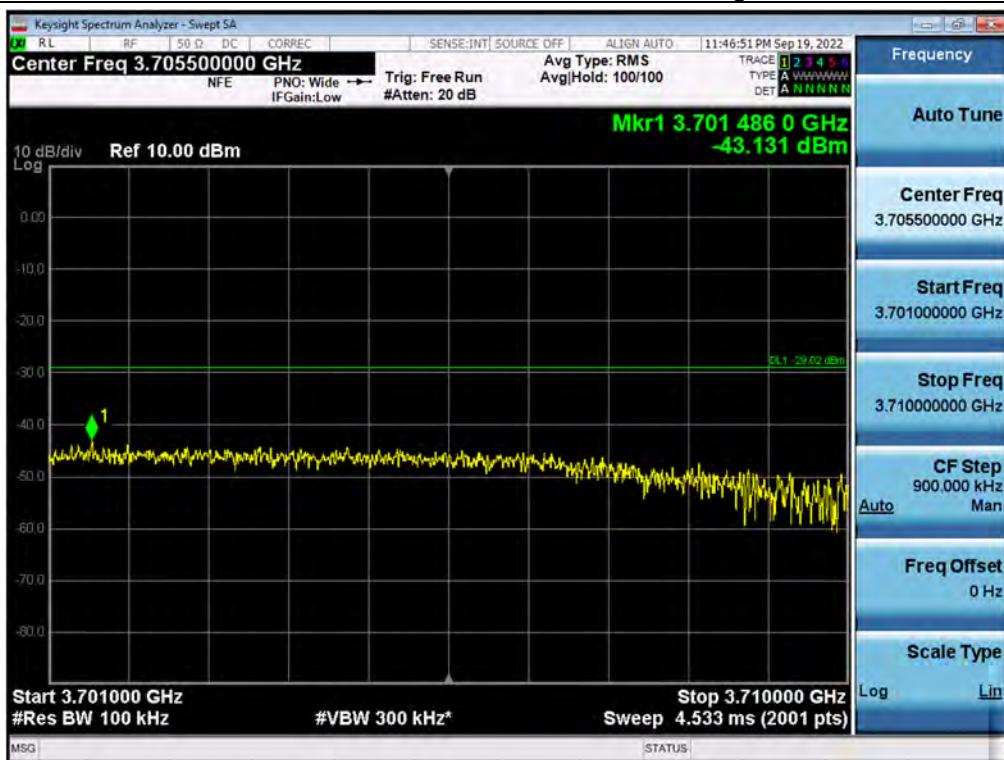
**Antenna 3 / 2<sup>nd</sup> High Edge + 10 MHz ~ 3720 MHz / CBRS NR 40 MHz 1C + (NR 10 MHz 1C + LTE 20 MHz 1C + LTE 5 MHz 1C + LTE 5 MHz 1C)[5C(1C+4C)] / Non-Contiguous / 64QAM**
