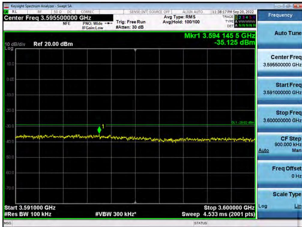
**Antenna 3 / 1<sup>st</sup> High Edge + 10 MHz ~ 2<sup>nd</sup> Low Edge - 10 MHz / CBRS NR 40 MHz 1C + (NR 10 MHz 1C + LTE 20 MHz 1C + LTE 5 MHz 1C + LTE 5 MHz 1C)[5C(1C+4C)] / Non-Contiguous / 64QAM**
