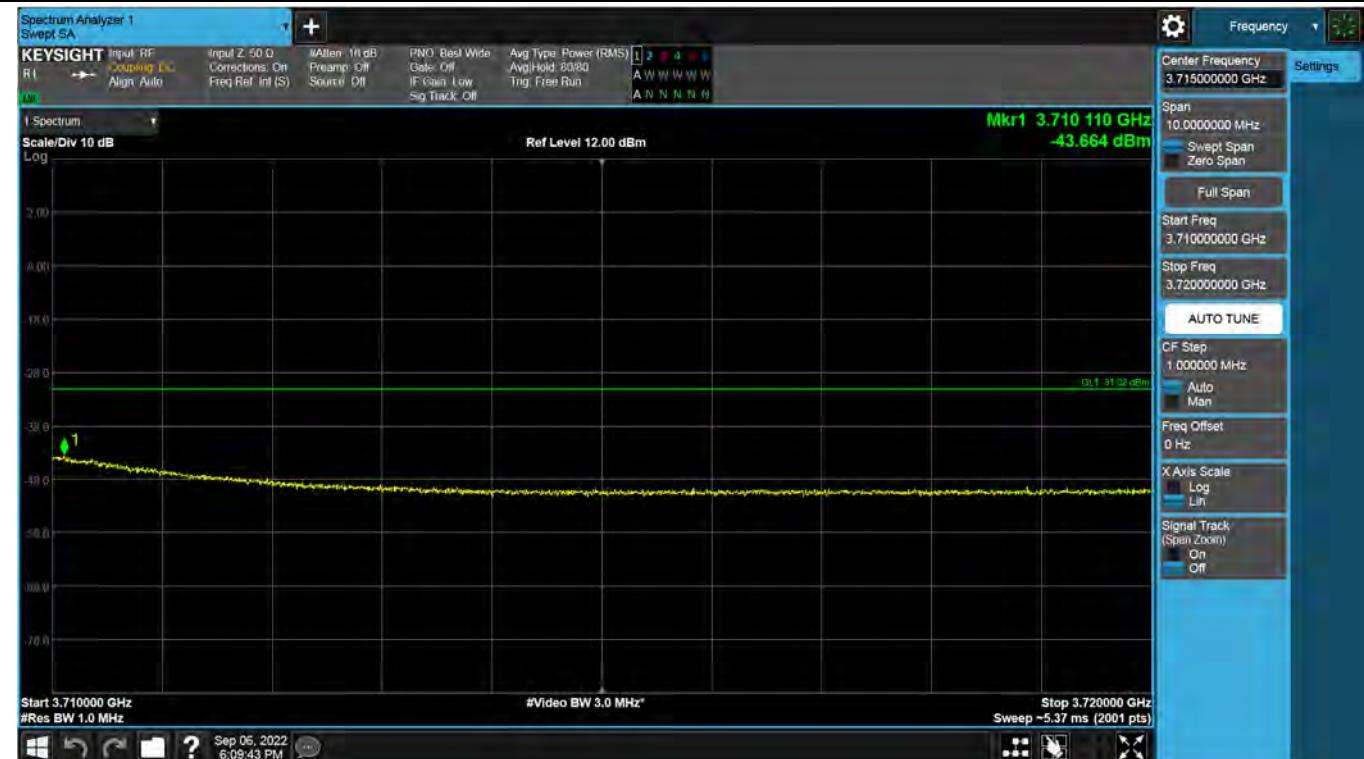
**Antenna 3 / 3720 MHz ~ 6 GHz / CBRS LTE[20 MHz 1C + (20 MHz 1C + 20 MHz 1C + 20 MHz 1C + 10 MHz 1C)][5C(1C+4C)] / Non-Contiguous / 64QAM**
