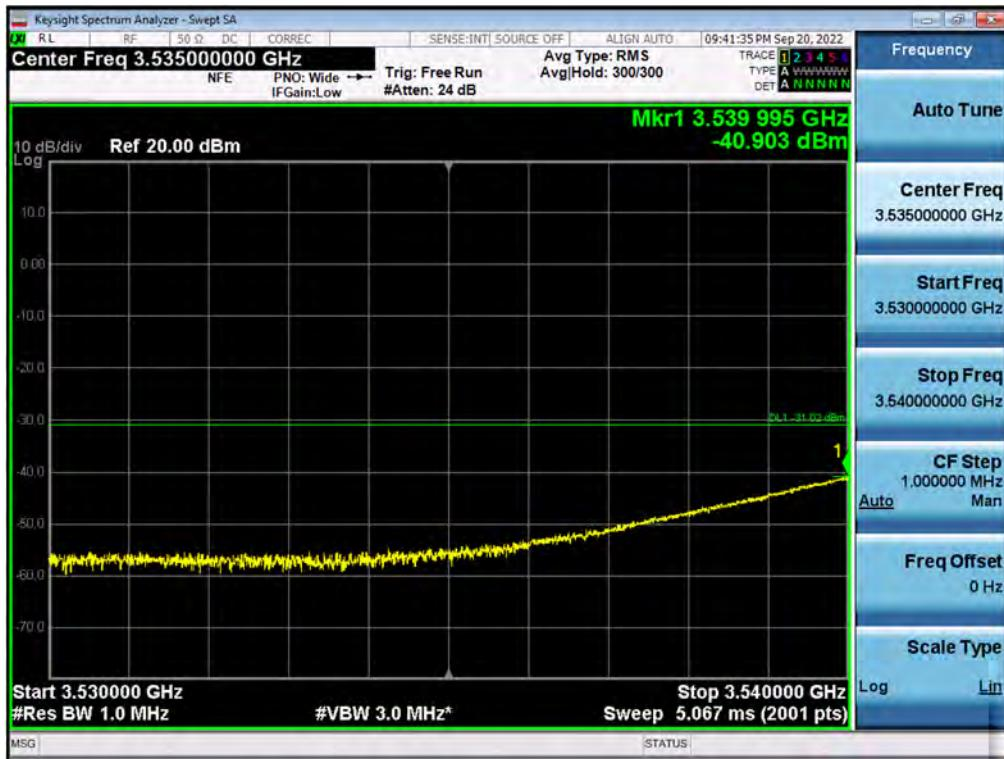
Antenna 3 / 1<sup>st</sup> Low Edge - 10 MHz ~ 1<sup>st</sup> Low Edge - 1 MHz / CBRS NR 40 MHz 1C + (NR 20 MHz 1C + NR 20 MHz 1C + LTE 10 MHz 1C + LTE 10 MHz 1C)[5C(1C+4C)] / Non-Contiguous / 256QAM
