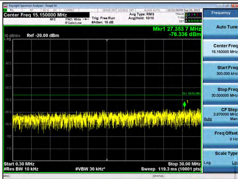
**Antenna 3 / 30 MHz ~ 3430 MHz / CBRS (NR 40 MHz 1C + NR 20 MHz 1C + NR 20 MHz 1C + LTE 10 MHz 1C) + LTE 10 MHz 1C[5C(4C+1C)] / Non-Contiguous / 64QAM**
