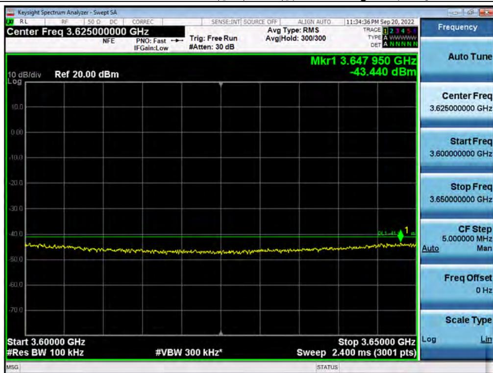
**Antenna 3 / 2<sup>nd</sup> High Edge - 10 MHz ~ 2<sup>nd</sup> High Edge - 1 MHz / CBRS NR 40 MHz 1C + (NR 10 MHz 1C + LTE 20 MHz 1C + LTE 5 MHz 1C + LTE 5 MHz 1C)[5C(1C+4C)] / Non-Contiguous / 64QAM**
