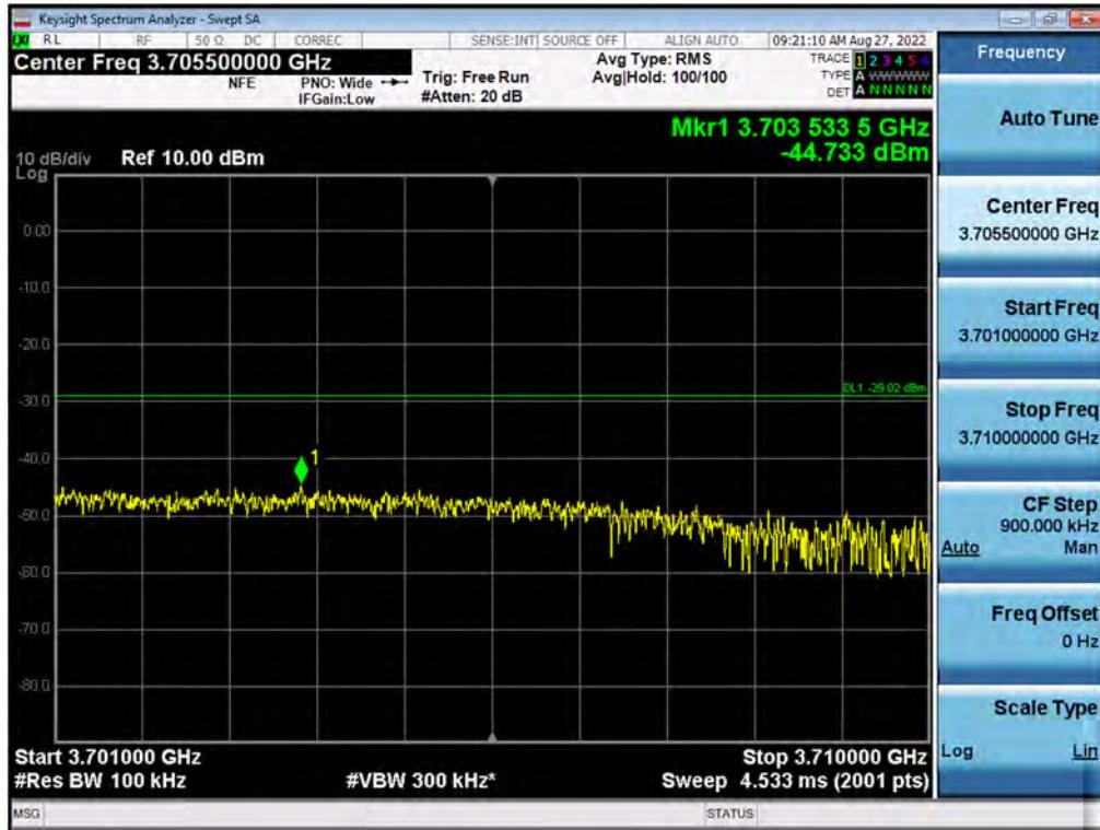
**Antenna 3 / 2<sup>nd</sup> High Edge + 10 MHz ~ 3720 MHz / CBRS LTE[20 MHz 1C + (20 MHz 1C + 20 MHz 1C + 20 MHz 1C + 10 MHz 1C)][5C(1C+4C)] / Non-Contiguous / QPSK**
