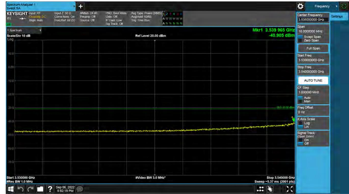
**Antenna 3 / 1<sup>st</sup> Low Edge - 10 MHz ~ 1<sup>st</sup> Low Edge - 1 MHz / CBRS LTE[(20 MHz 1C + 20 MHz 1C + 20 MHz 1C + 20 MHz 1C) + 10 MHz 1C][5C(4C+1C)] / Non-Contiguous / 64QAM**
