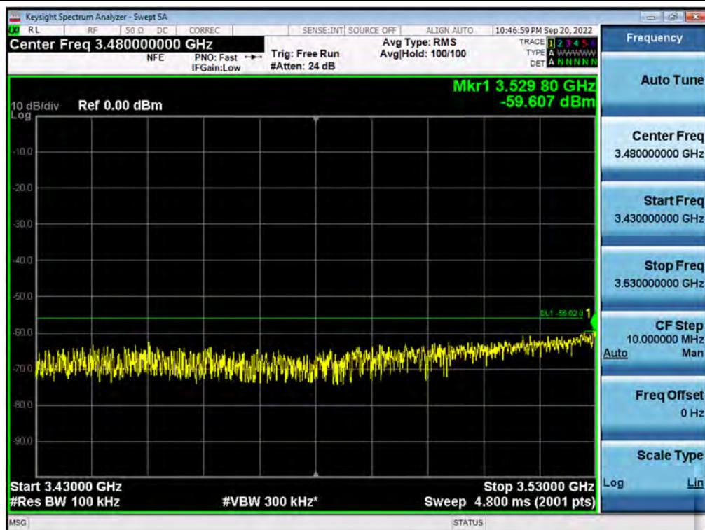
**Antenna 3 / 3530 MHz ~ 1<sup>st</sup> Low Edge - 10 MHz / CBRS (NR 40 MHz 1C + NR 20 MHz 1C + NR 20 MHz 1C + LTE 10 MHz 1C) + LTE 10 MHz 1C[5C(4C+1C)] / Non-Contiguous / QPSK**
