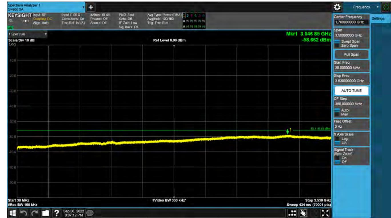
**Antenna 0 / 3530 MHz ~ 1<sup>st</sup> Low Edge - 10 MHz / CBRS LTE[20 MHz 1C + (20 MHz 1C + 20 MHz 1C + 20 MHz 1C + 20 MHz 1C)][5C(1C+4C)] / Non-Contiguous / QPSK**
