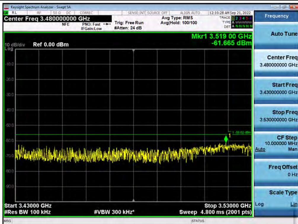
**Antenna 3 / 3530 MHz ~ 1<sup>st</sup> Low Edge - 10 MHz / CBRS (NR 40 MHz 1C + NR 10 MHz 1C + LTE 20 MHz 1C + LTE 5 MHz 1C[5C(4C+1C)] / Non-Contiguous / 64QAM**
