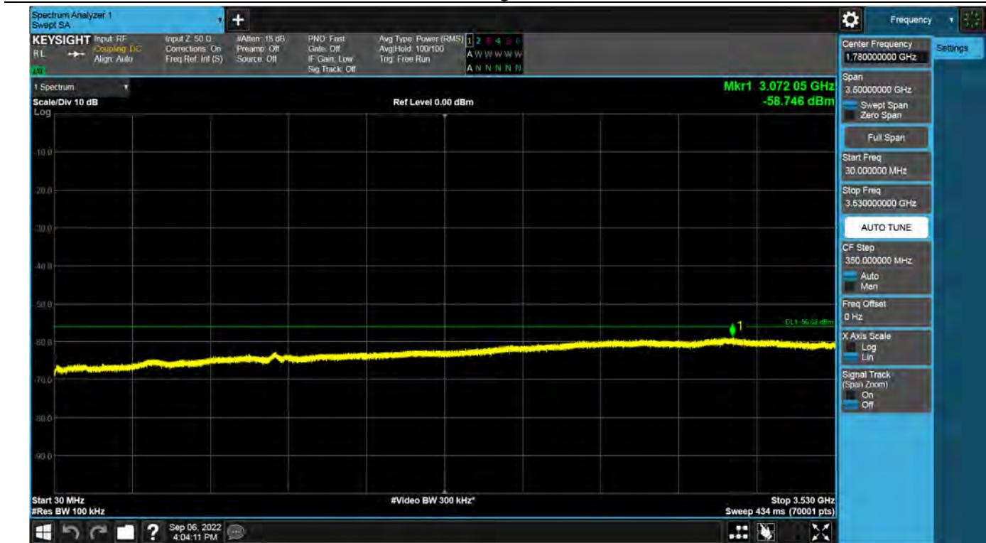
**Antenna 3 / 3530 MHz ~ 1<sup>st</sup> Low Edge - 10 MHz / CBRS LTE[(15 MHz 1C + 15 MHz 1C + 15 MHz 1C + 15 MHz 1C) + 10 MHz 1C][5C(4C+1C)] / Non-Contiguous / QPSK**
