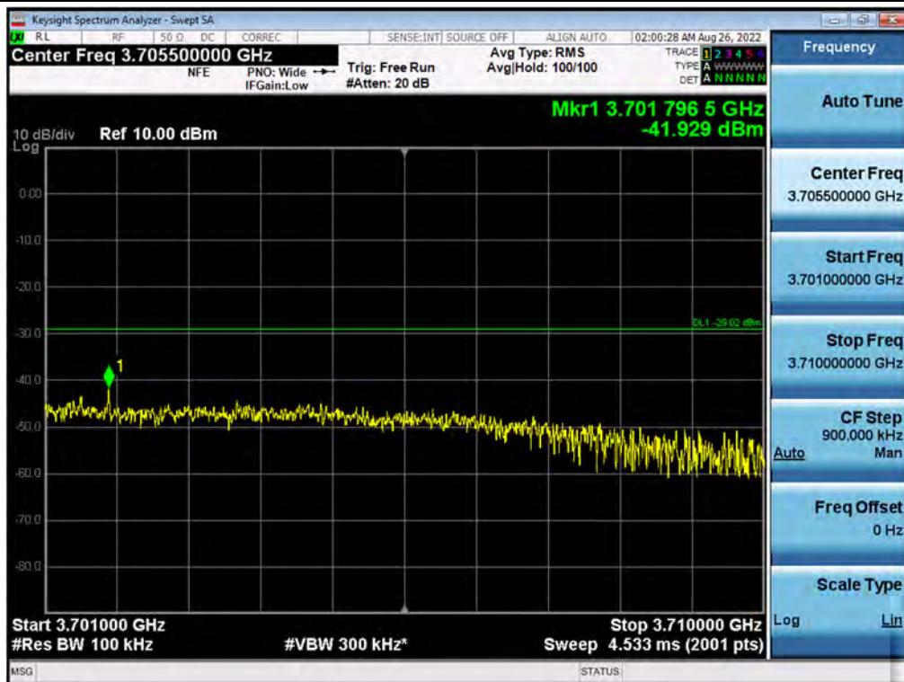
**Antenna 3 / 2<sup>nd</sup> High Edge + 10 MHz ~ 3720 MHz / CBRS LTE[(15 MHz 1C + 15 MHz 1C + 15 MHz 1C + 15 MHz 1C) + 10 MHz 1C][5C(4C+1C)] / Non-Contiguous / QPSK**
