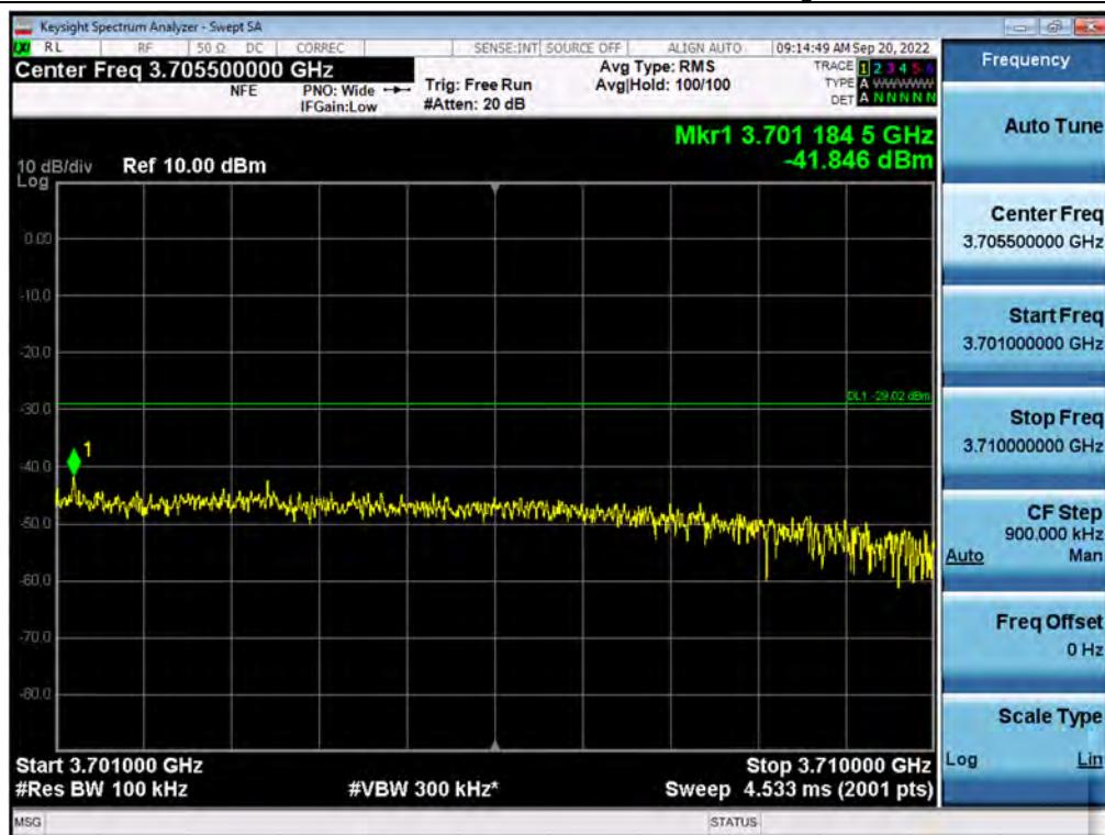
**Antenna 3 / 2<sup>nd</sup> High Edge + 10 MHz ~ 3720 MHz / CBRS (NR 40 MHz 1C + NR 10 MHz 1C + LTE 20 MHz 1C + LTE 5 MHz 1C + LTE 5 MHz 1C[5C(4C+1C)] / Non-Contiguous / 16QAM**
