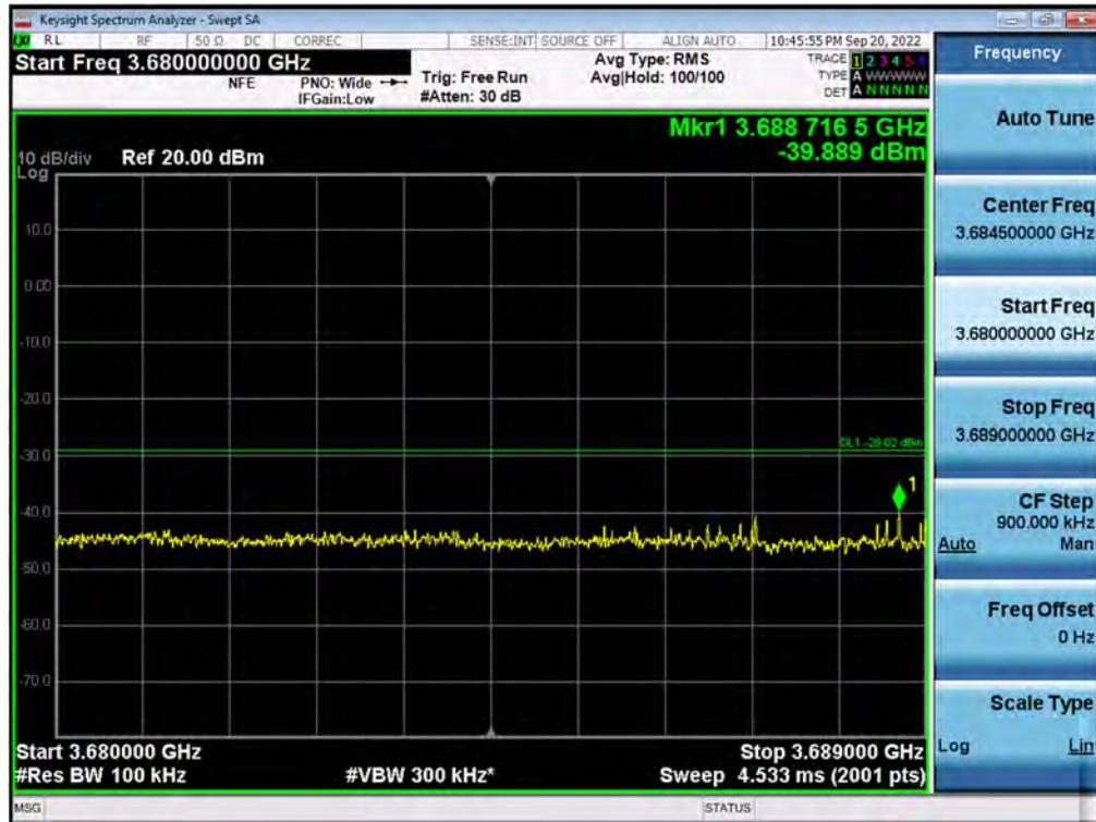
**Antenna 3 / 2<sup>nd</sup> High Edge + 1 MHz ~ 2<sup>nd</sup> High Edge + 10 MHz / CBRS (NR 40 MHz 1C + NR 20 MHz 1C + NR 20 MHz 1C + LTE 10 MHz 1C) + LTE 10 MHz 1C[5C(4C+1C)] / Non-Contiguous / 16QAM**
