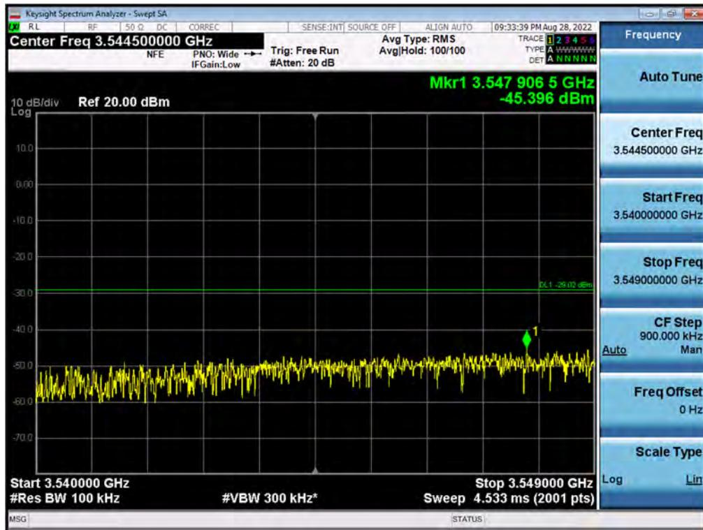
**Antenna 0 / 1<sup>st</sup> High Edge + 1 MHz ~ 1<sup>st</sup> High Edge + 10 MHz / CBRS LTE[20 MHz 1C + (20 MHz 1C + 20 MHz 1C + 20 MHz 1C + 20 MHz 1C)][5C(1C+4C)] / Non-Contiguous / 16QAM**
