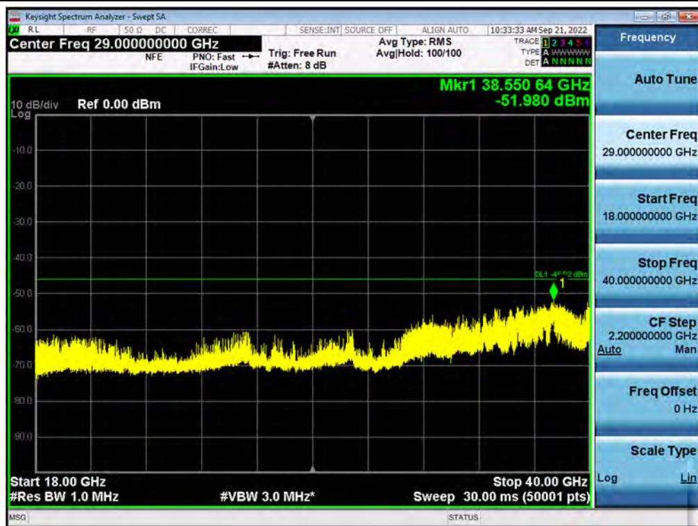
**Antenna 3 / 9 kHz ~ 300 kHz / CBRS (NR 40 MHz 1C + NR 10 MHz 1C + LTE 20 MHz 1C + LTE 5 MHz 1C) + LTE 5 MHz 1C[5C(4C+1C)] / Non-Contiguous / 16QAM**
