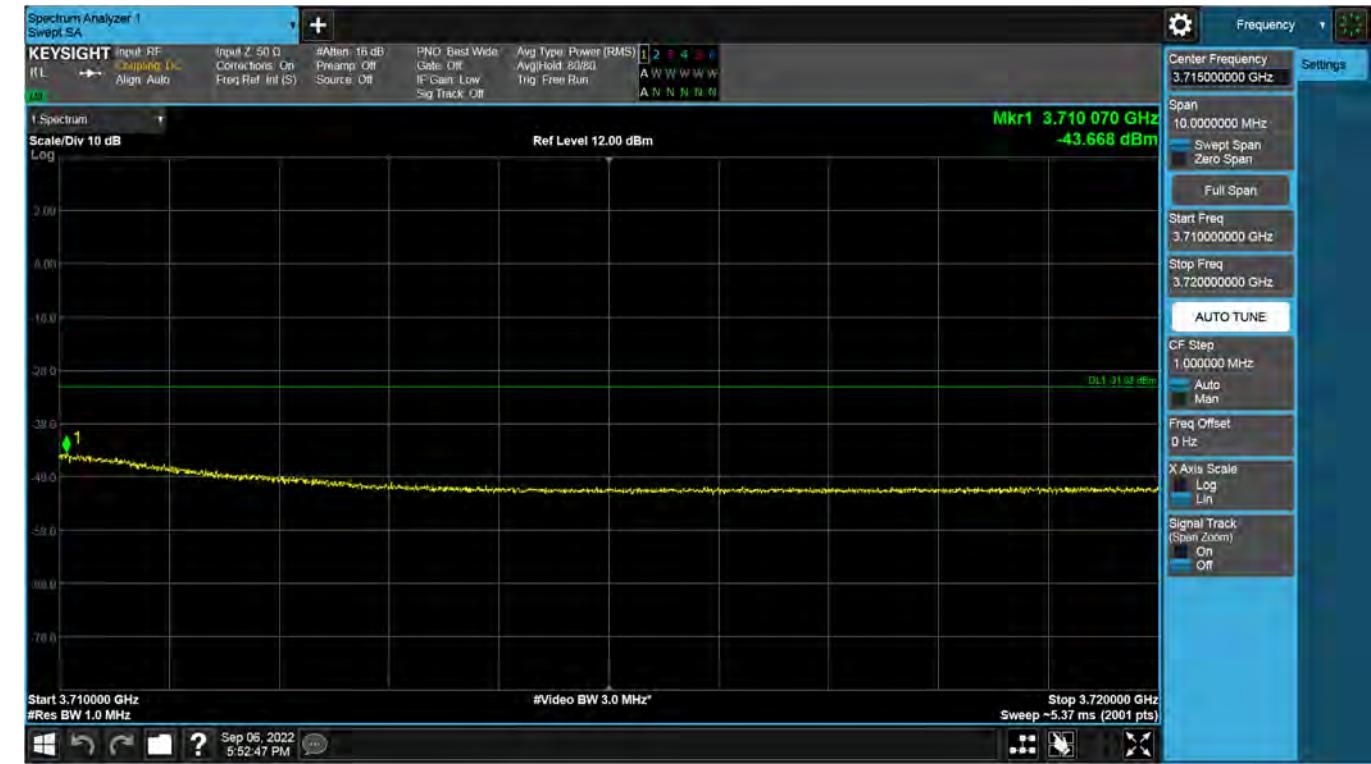
**Antenna 3 / 3720 MHz ~ 6 GHz / CBRS LTE[(20 MHz 1C + 20 MHz 1C + 20 MHz 1C + 20 MHz 1C) + 10 MHz 1C][5C(4C+1C)] / Non-Contiguous / 64QAM**
