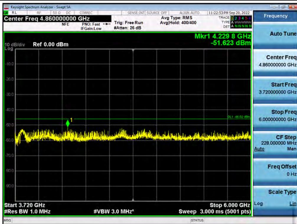
**Antenna 3 / 6 GHz ~ 18 GHz / CBRS NR 40 MHz 1C + (NR 10 MHz 1C + LTE 20 MHz 1C + LTE 5 MHz 1C + LTE 5 MHz 1C)[5C(1C+4C)] / Non-Contiguous / QPSK**
