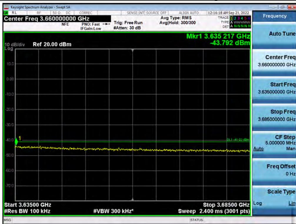
**Antenna 3 / 2<sup>nd</sup> High Edge - 10 MHz ~ 2<sup>nd</sup> High Edge - 1 MHz / CBRS (NR 40 MHz 1C + NR 10 MHz 1C + LTE 20 MHz 1C + LTE 5 MHz 1C) + LTE 5 MHz 1C[5C(4C+1C)] / Non-Contiguous / QPSK**
