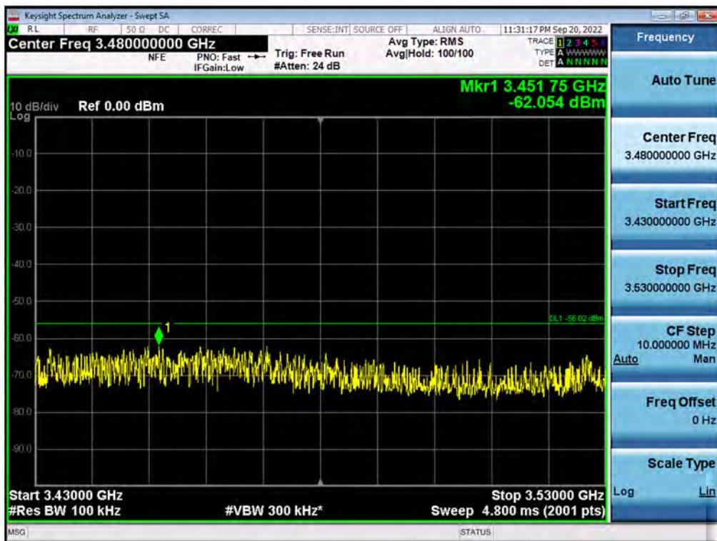
Antenna 3 / 3530 MHz ~ 1<sup>st</sup> Low Edge - 10 MHz / CBRS NR 40 MHz 1C + (NR 10 MHz 1C + LTE 20 MHz 1C + LTE 5 MHz 1C)[5C(1C+4C)] / Non-Contiguous / 16QAM
