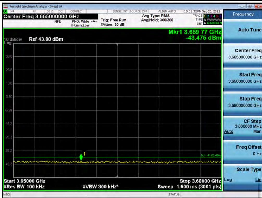
**Antenna 3 / 2<sup>nd</sup> High Edge - 10 MHz ~ 2<sup>nd</sup> High Edge - 1 MHz / CBRS (NR 40 MHz 1C + NR 20 MHz 1C + NR 20 MHz 1C + LTE 10 MHz 1C) + LTE 10 MHz 1C[5C(4C+1C)] / Non-Contiguous / QPSK**
