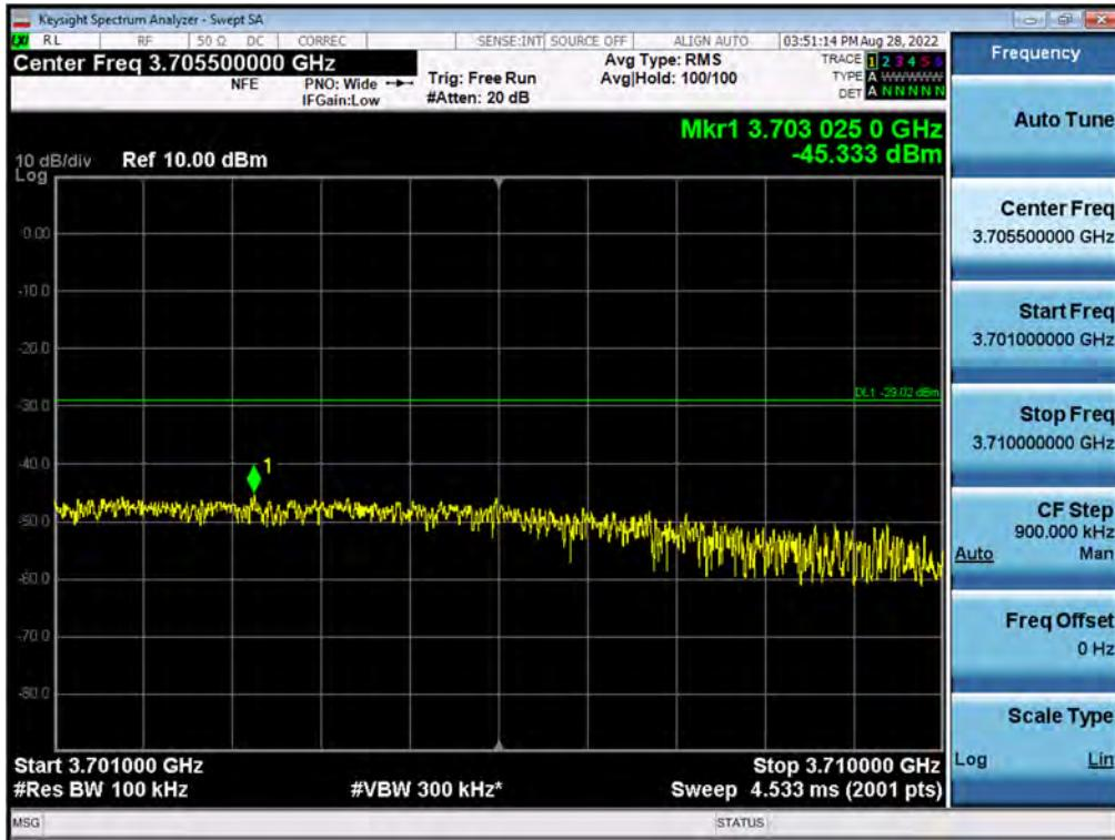
Antenna 0 / 2<sup>nd</sup> High Edge + 10 MHz ~ 3720 MHz / CBRS LTE[20 MHz 1C + (20 MHz 1C + 20 MHz 1C + 20 MHz 1C + 20 MHz 1C)][5C(1C+4C)] / Non-Contiguous / QPSK
