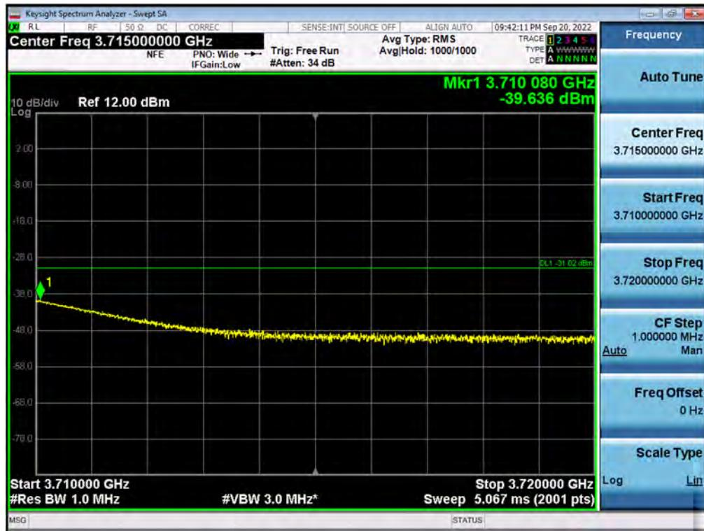
Antenna 3 / 3720 MHz ~ 6 GHz / CBRS NR 40 MHz 1C + (NR 20 MHz 1C + NR 20 MHz 1C + LTE 10 MHz 1C + LTE 10 MHz 1C)[5C(1C+4C)] / Non-Contiguous / 16QAM
