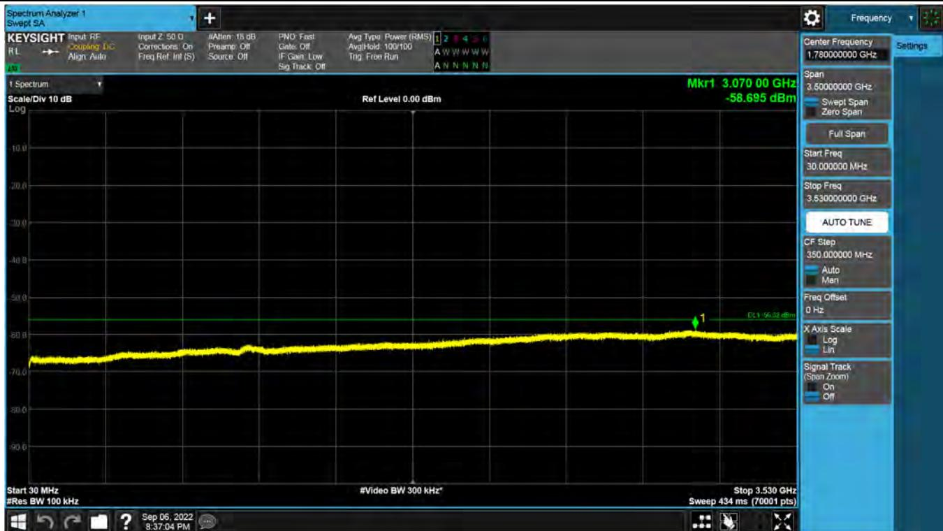
**Antenna 1 / 3530 MHz ~ 1<sup>st</sup> Low Edge - 10 MHz / CBRS LTE[(20 MHz 1C + 20 MHz 1C + 20 MHz 1C + 20 MHz 1C) + 20 MHz 1C][5C(4C+1C)] / Non-Contiguous / QPSK**
