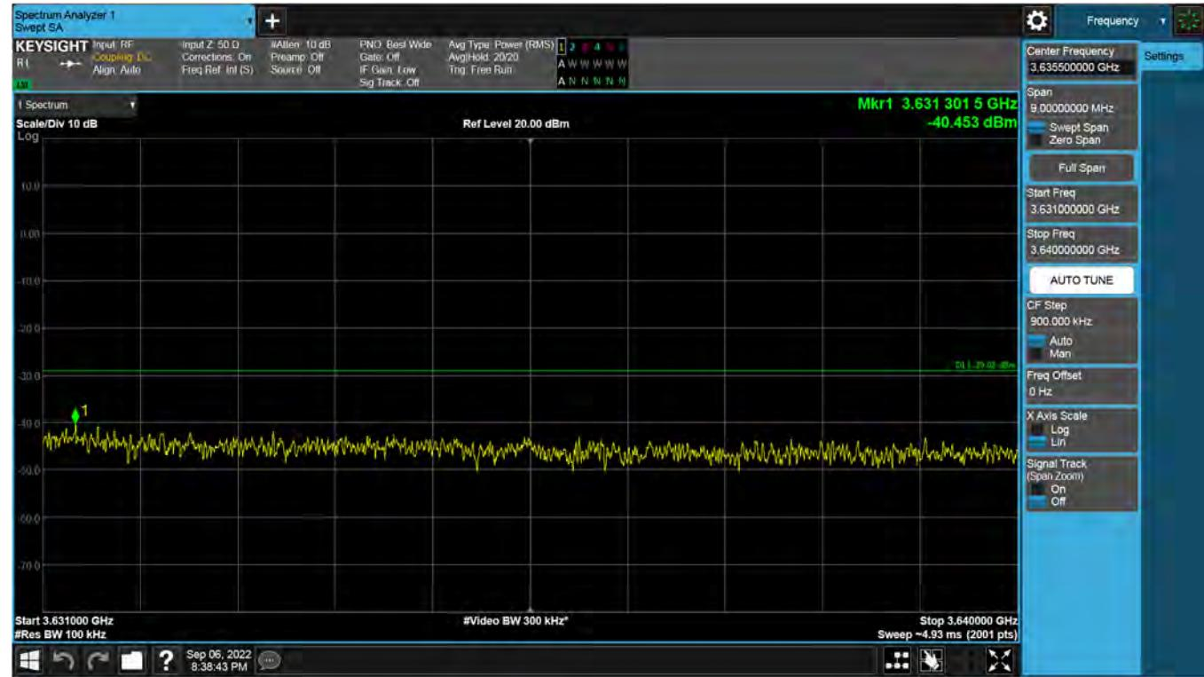
**Antenna 1 / 1<sup>st</sup> High Edge + 10 MHz ~ 2<sup>nd</sup> Low Edge - 10 MHz / CBRS LTE[(20 MHz 1C + 20 MHz 1C + 20 MHz 1C) + 20 MHz 1C][5C(4C+1C)] / Non-Contiguous / 16QAM**
