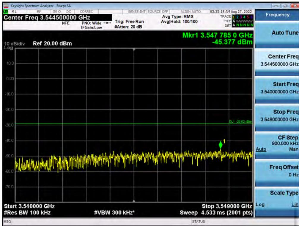
**Antenna 3 / 1<sup>st</sup> High Edge + 1 MHz ~ 1<sup>st</sup> High Edge + 10 MHz / CBRS LTE[20 MHz 1C + (20 MHz 1C + 20 MHz 1C + 20 MHz 1C + 10 MHz 1C)][5C(1C+4C)] / Non-Contiguous / QPSK**
