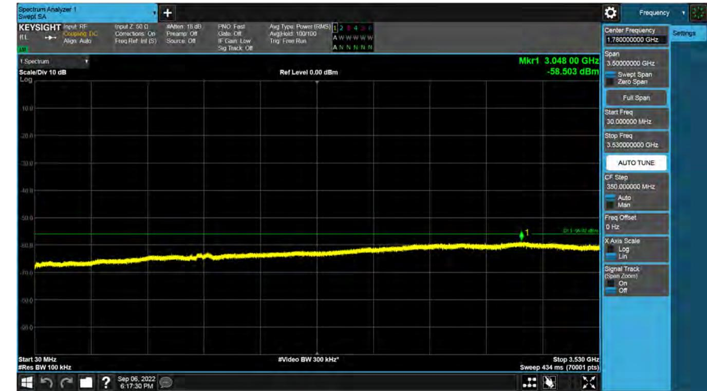
**Antenna 3 / 3530 MHz ~ 1<sup>st</sup> Low Edge - 10 MHz / CBRS LTE[20 MHz 1C + (20 MHz 1C + 20 MHz 1C + 20 MHz 1C + 10 MHz 1C)][5C(1C+4C)] / Non-Contiguous / QPSK**
