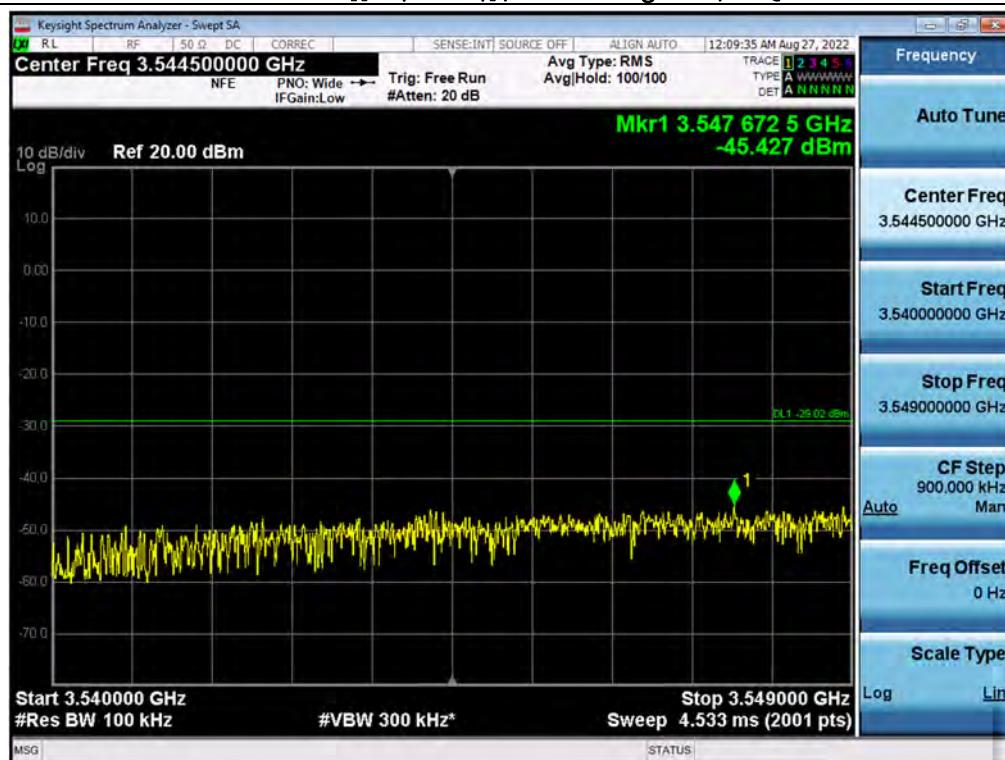
**Antenna 3 / 1<sup>st</sup> High Edge + 1 MHz ~ 1<sup>st</sup> High Edge + 10 MHz / CBRS LTE[(20 MHz 1C + 20 MHz 1C + 20 MHz 1C) + 10 MHz 1C][5C(4C+1C)] / Non-Contiguous / QPSK**
