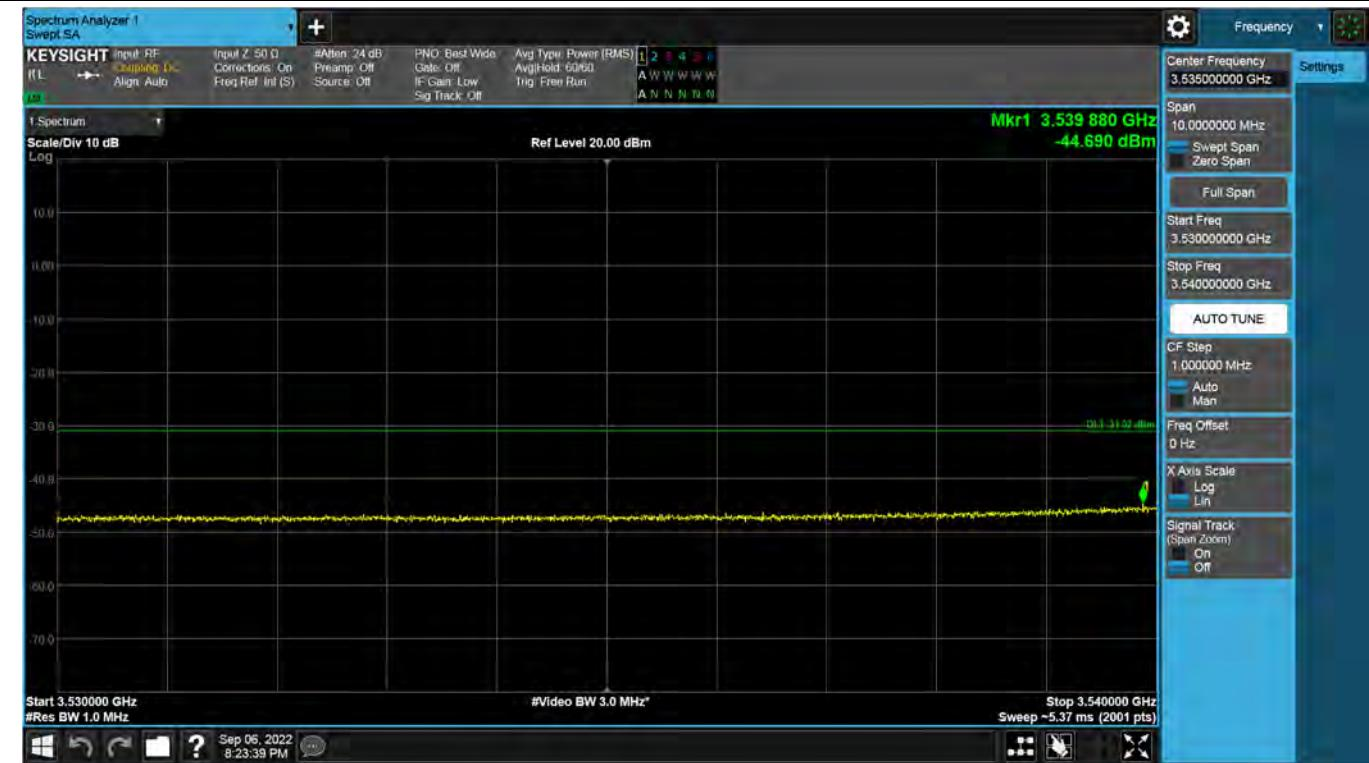
**Antenna 1 / 1<sup>st</sup> Low Edge - 10 MHz ~ 1<sup>st</sup> Low Edge - 1 MHz / CBRS LTE[(20 MHz 1C + 20 MHz 1C + 20 MHz 1C + 20 MHz 1C) + 20 MHz 1C][5C(4C+1C)] / Non-Contiguous / 16QAM**
