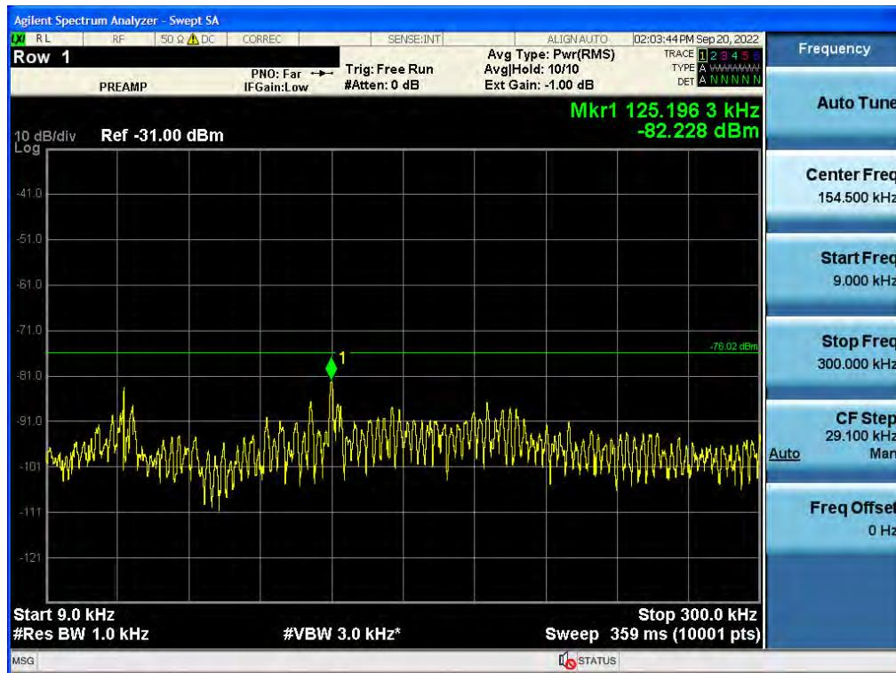
Antenna 0 / 300 kHz ~ 30 MHz / CBRS LTE[20 MHz 1C + (20 MHz 1C + 20 MHz 1C + 20 MHz 1C + 20 MHz 1C)][5C(1C+4C)] / Non-Contiguous / 16QAM
