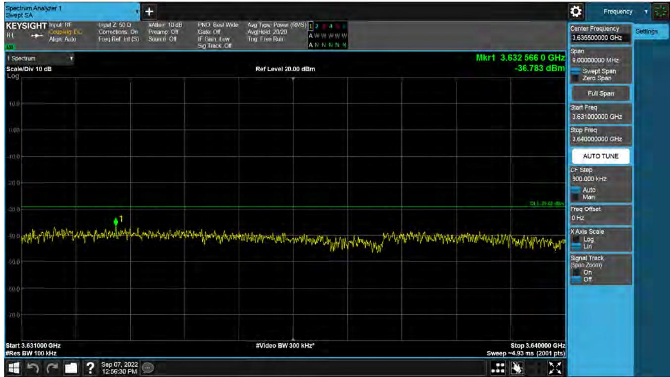
**Antenna 3 / 1<sup>st</sup> High Edge + 10 MHz ~ 2<sup>nd</sup> Low Edge - 10 MHz / CBRS LTE[(20 MHz 1C + 20 MHz 1C + 20 MHz 1C) + 10 MHz 1C][5C(4C+1C)] / Non-Contiguous / 256QAM**
