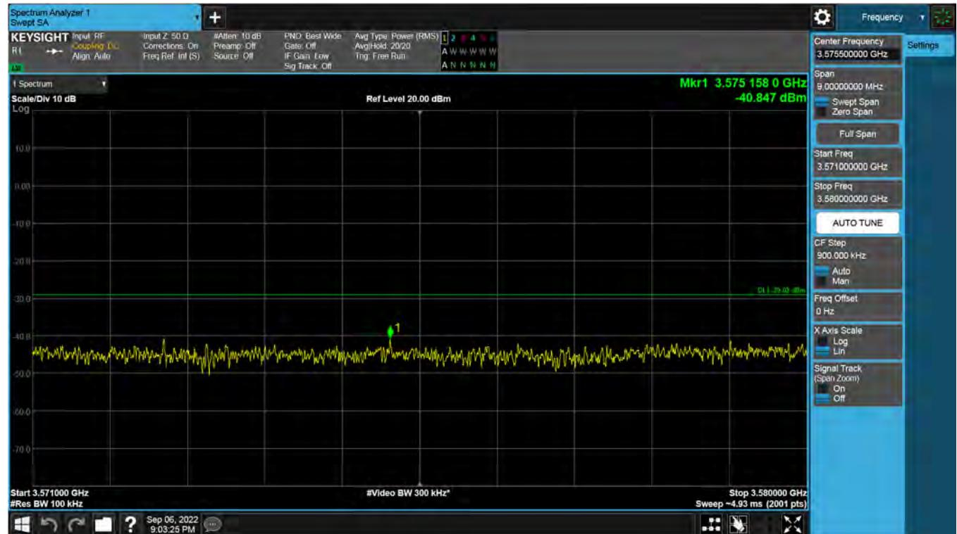
**Antenna 0 / 1<sup>st</sup> High Edge + 10 MHz ~ 2<sup>nd</sup> Low Edge - 10 MHz / CBRS LTE[20 MHz 1C + (20 MHz 1C + 20 MHz 1C + 20 MHz 1C + 20 MHz 1C)][5C(1C+4C)] / Non-Contiguous / 64QAM**
