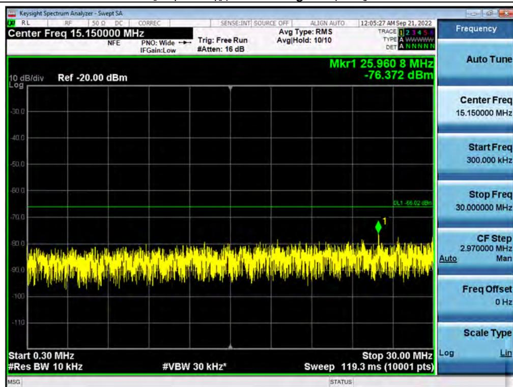
**Antenna 3 / 30 MHz ~ 3540 MHz / CBRS (NR 40 MHz 1C + NR 10 MHz 1C + LTE 20 MHz 1C + LTE 5 MHz 1C[5C(4C+1C)] / Non-Contiguous / QPSK**
