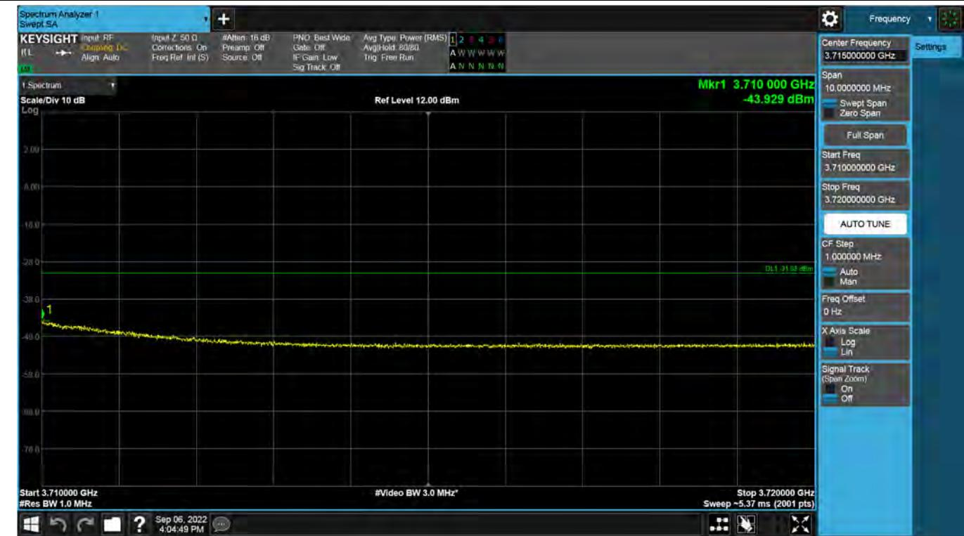
**Antenna 3 / 3720 MHz ~ 6 GHz / CBRS LTE[(15 MHz 1C + 15 MHz 1C + 15 MHz 1C + 15 MHz 1C) + 10 MHz 1C][5C(4C+1C)] / Non-Contiguous / 16QAM**
