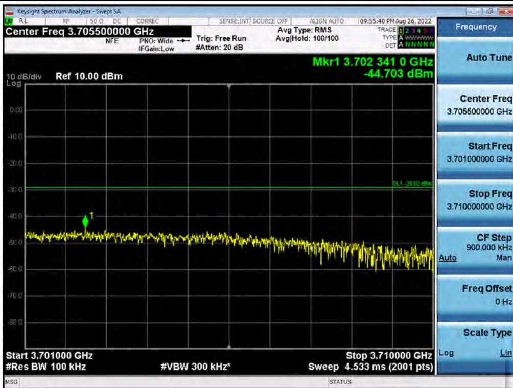
**Antenna 3 / 2<sup>nd</sup> High Edge + 10 MHz ~ 3720 MHz / CBRS LTE[(20 MHz 1C + 20 MHz 1C + 20 MHz 1C + 20 MHz 1C) + 10 MHz 1C][5C(4C+1C)] / Non-Contiguous / QPSK**
