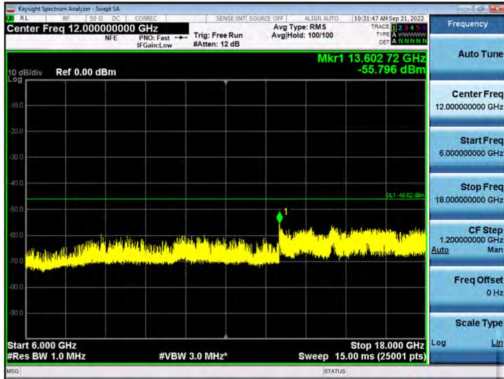
**Antenna 3 / 18 GHz ~ 40 GHz / CBRS (NR 40 MHz 1C + NR 20 MHz 1C + NR 20 MHz 1C + LTE 10 MHz 1C) + LTE 10 MHz 1C[5C(4C+1C)] / Non-Contiguous / 256QAM**
