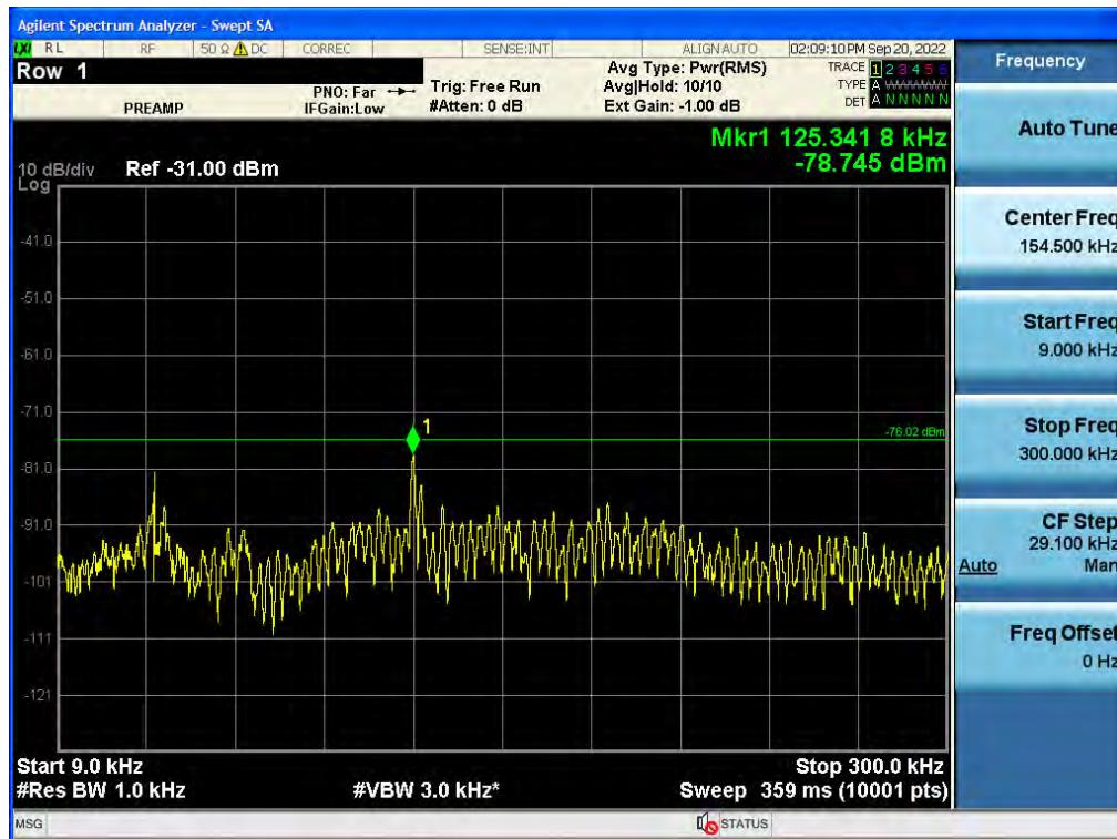
**Antenna 3 / 300 kHz ~ 30 MHz / CBRS LTE[20 MHz 1C + (20 MHz 1C + 20 MHz 1C + 20 MHz 1C + 10 MHz 1C)][5C(1C+4C)] / Non-Contiguous / QPSK**
