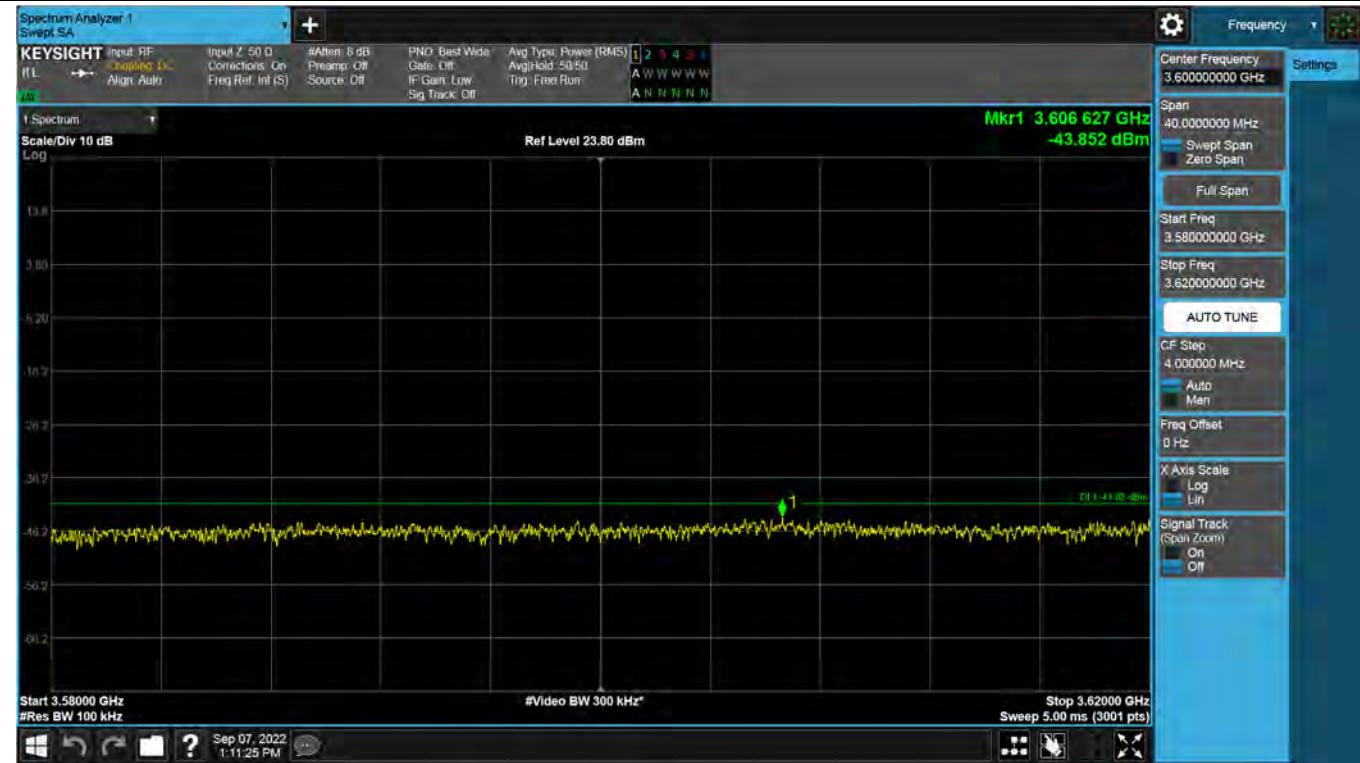
**Antenna 3 / 2<sup>nd</sup> High Edge - 10 MHz ~ 2<sup>nd</sup> High Edge - 1 MHz / CBRS LTE[20 MHz 1C + (20 MHz 1C + 20 MHz 1C + 20 MHz 1C + 10 MHz 1C)][5C(1C+4C)] / Non-Contiguous / QPSK**
