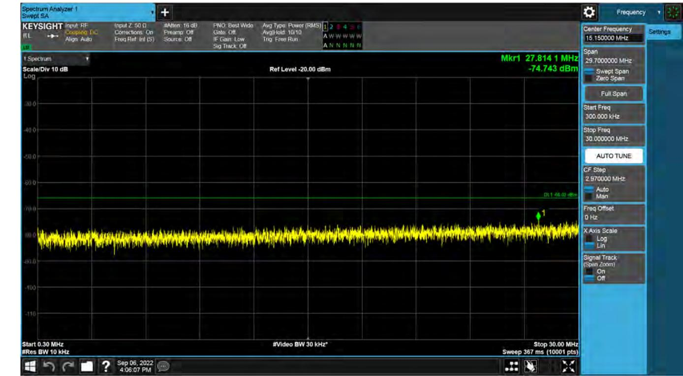
**Antenna 3 / 30 MHz ~ 3530 MHz / CBRS LTE[(15 MHz 1C + 15 MHz 1C + 15 MHz 1C + 15 MHz 1C) + 10 MHz 1C][5C(4C+1C)] / Non-Contiguous / QPSK**
