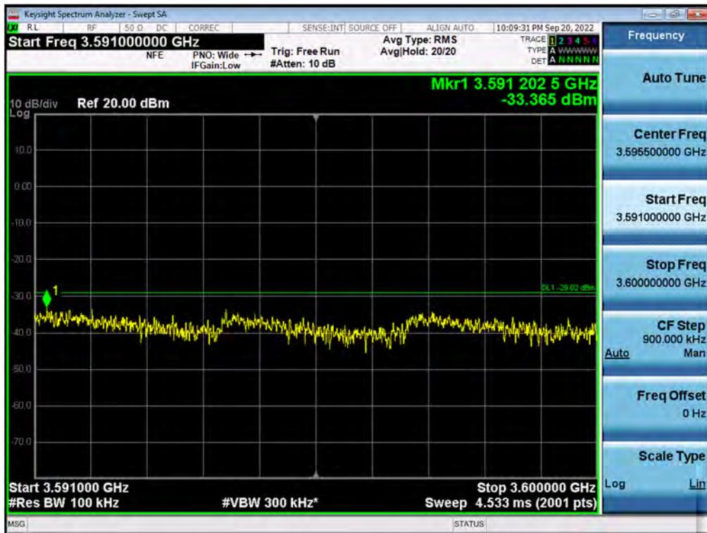
**Antenna 3 / 1<sup>st</sup> High Edge + 10 MHz ~ 2<sup>nd</sup> Low Edge - 10 MHz / CBRS NR 40 MHz 1C + (NR 20 MHz 1C + NR 20 MHz 1C + LTE 10 MHz 1C + LTE 10 MHz 1C)[5C(1C+4C)] / Non-Contiguous / QPSK**
