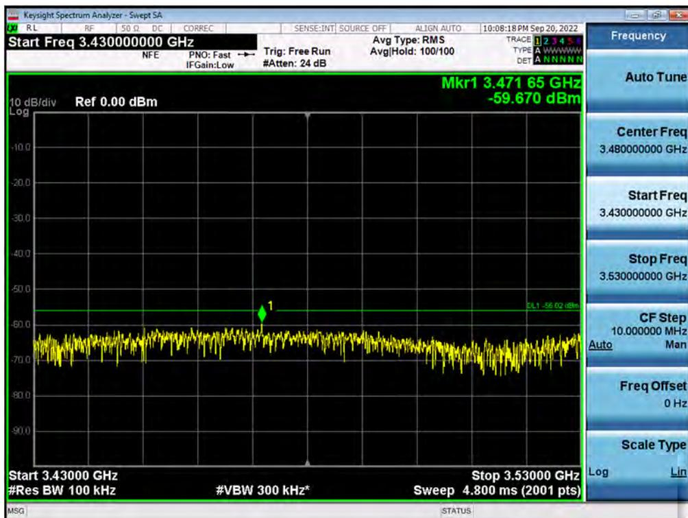
Antenna 3 / 3530 MHz ~ 1<sup>st</sup> Low Edge - 10 MHz / CBRS NR 40 MHz 1C + (NR 20 MHz 1C + NR 20 MHz 1C + LTE 10 MHz 1C + LTE 10 MHz 1C)[5C(1C+4C)] / Non-Contiguous / QPSK
