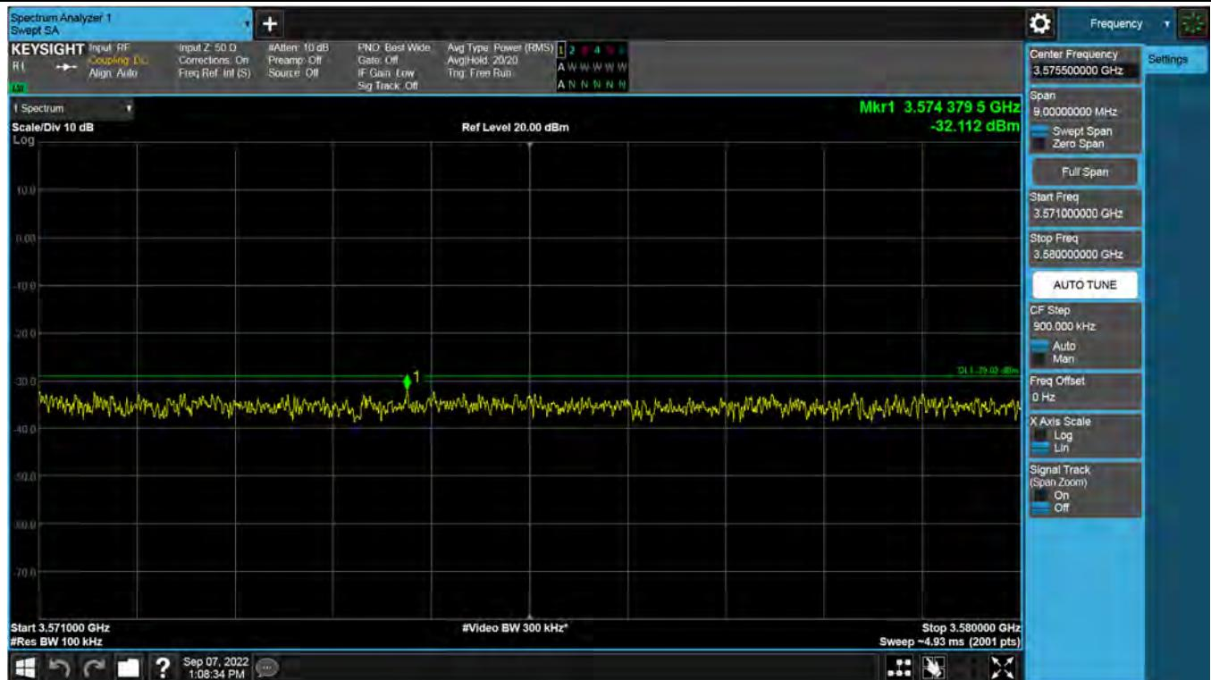
**Antenna 3 / 1<sup>st</sup> High Edge + 10 MHz ~ 2<sup>nd</sup> Low Edge - 10 MHz / CBRS LTE[20 MHz 1C + (20 MHz 1C + 20 MHz 1C + 20 MHz 1C + 10 MHz 1C)][5C(1C+4C)] / Non-Contiguous / QPSK**
