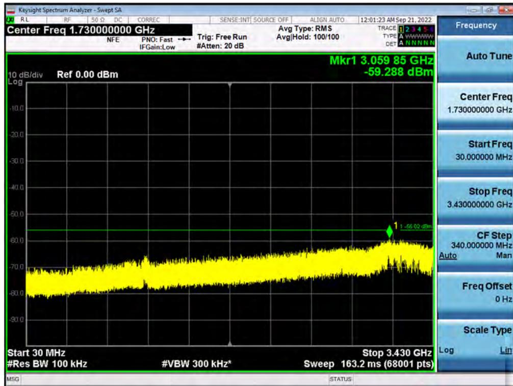
**Antenna 3 / 3540 MHz ~ 3530 MHz / CBRS (NR 40 MHz 1C + NR 10 MHz 1C + LTE 20 MHz 1C + LTE 5 MHz 1C) + LTE 5 MHz 1C[5C(4C+1C)] / Non-Contiguous / 64QAM**
