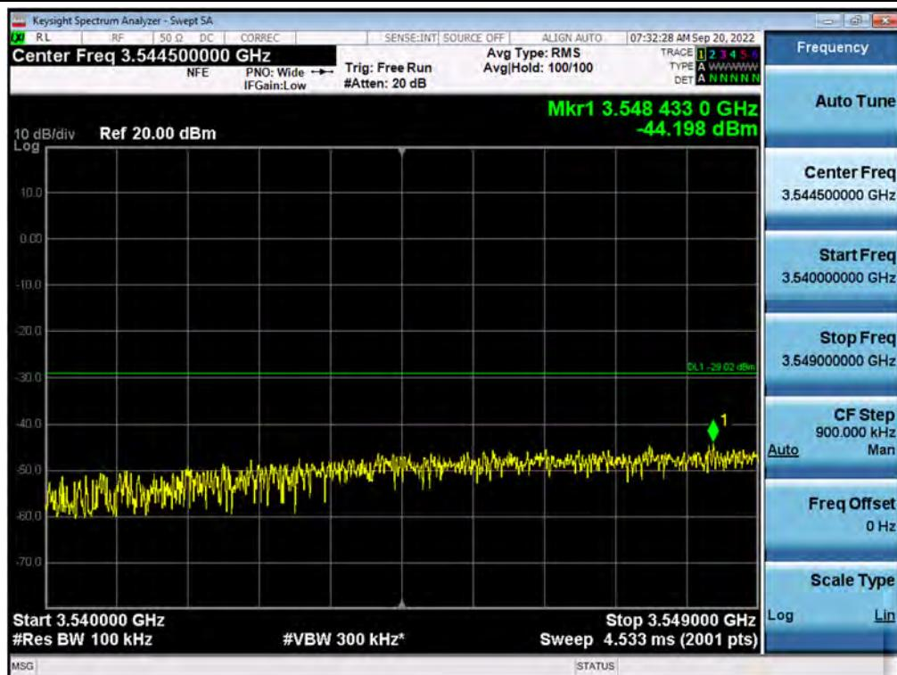
**Antenna 3 / 1<sup>st</sup> High Edge + 1 MHz ~ 1<sup>st</sup> High Edge + 10 MHz / CBRS (NR 40 MHz 1C + NR 10 MHz 1C + LTE 20 MHz 1C + LTE 5 MHz 1C) + LTE 5 MHz 1C[5C(4C+1C)] / Non-Contiguous / 16QAM**
