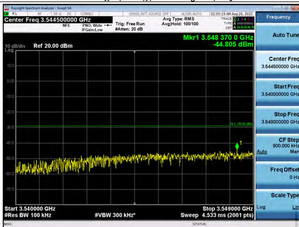
**Antenna 3 / 1<sup>st</sup> High Edge + 1 MHz ~ 1<sup>st</sup> High Edge + 10 MHz / CBRS LTE[(15 MHz 1C + 15 MHz 1C + 15 MHz 1C) + 10 MHz 1C][5C(4C+1C)] / Non-Contiguous / QPSK**
