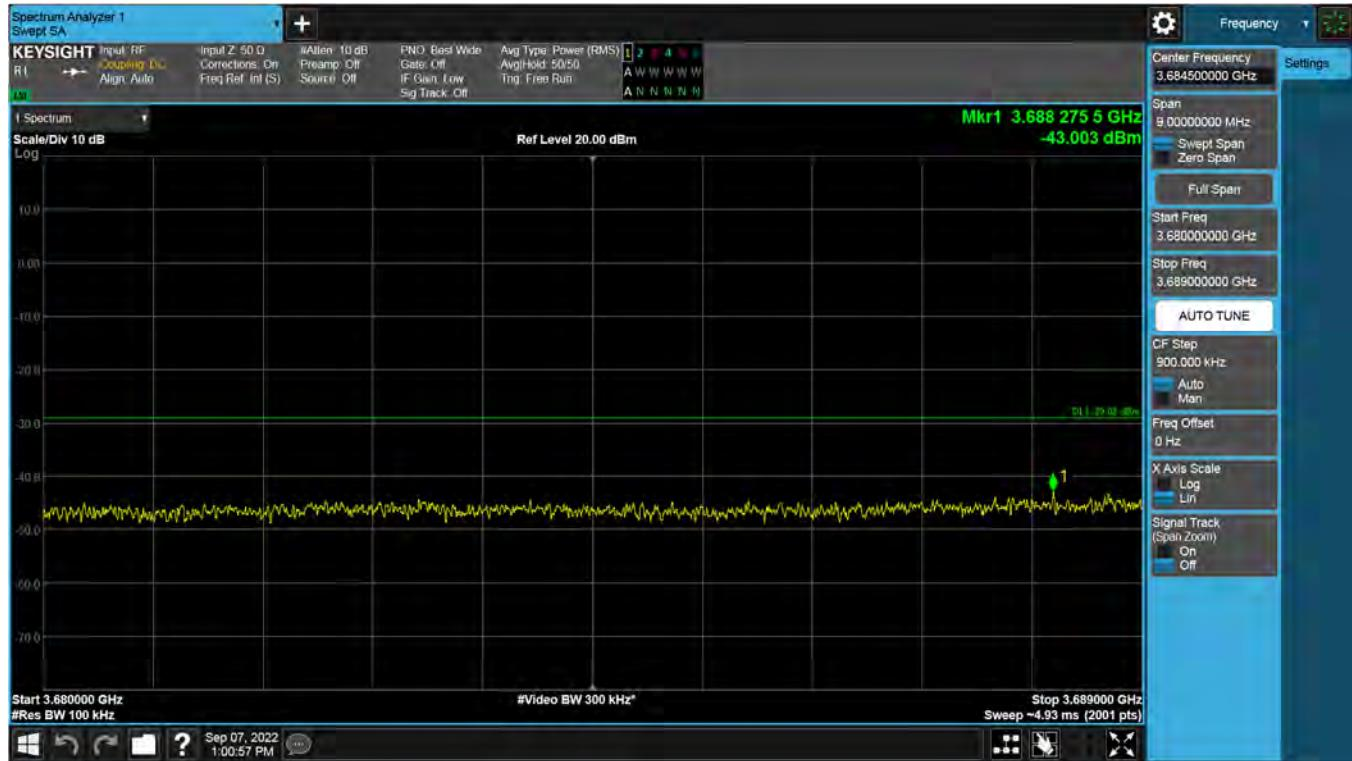
**Antenna 3 / 2<sup>nd</sup> High Edge + 1 MHz ~ 2<sup>nd</sup> High Edge + 10 MHz / CBRS LTE[(20 MHz 1C + 20 MHz 1C + 20 MHz 1C) + 10 MHz 1C][5C(4C+1C)] / Non-Contiguous / 16QAM**
