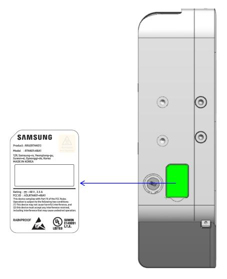
The FCC Identifier Label will be displayed on the rear side of the DU (Digital Unit) shelf in accordance with the following format, displaying FCC ID: A3LRT4401-48A1. The adhesive label shall be permanently affixed at a conspicuous location on the device.
