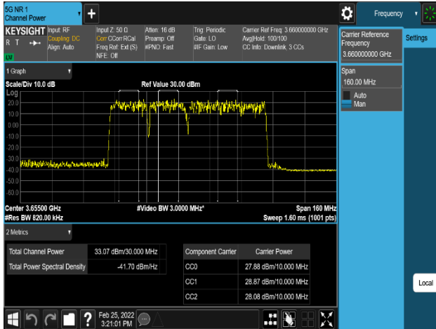
Plot 11-16. Equivalent Isotropic Radiated Power Plot (LTE_2C+NR_1C_20M+20M+40M_256QAM-High Channel, Port2)
