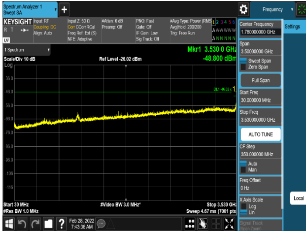
Plot 11-28. Conducted Spurious Emission Plot 30 MHz to 3.53 GHz (LTE_2C+NR_1C_20M+20M+40M_QPSK - low Channel, Port 0)
