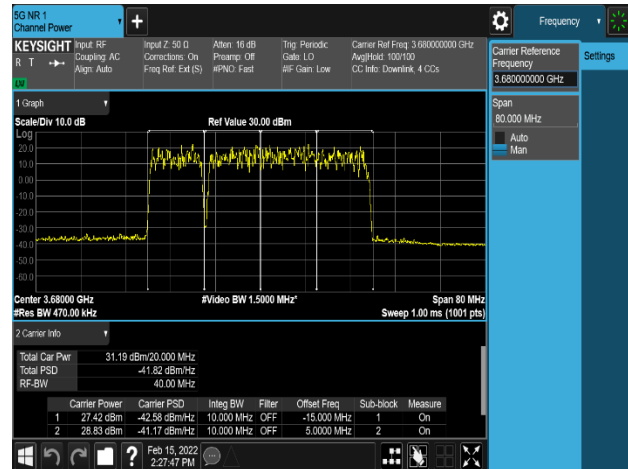
Plot 11-13. Equivalent Isotropic Radiated Power Plot (NR_n48_2C_10M+30M_QPSK - High Channel, Port 3)
