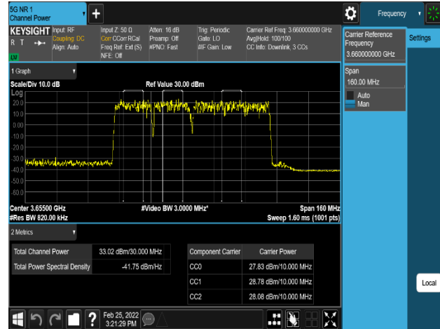
Plot 11-20. Equivalent Isotropic Radiated Power Plot (LTE_2C+NR_1C_20M+20M+40M_256QAM-High Channel, Port3)
