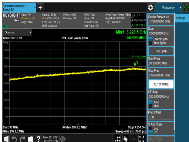
Plot 8-484. Conducted Spurious Emission Plot 30 MHz to 3.53 GHz (NR_n48_2C_40M+40M_QPSK - Mid Channel, Port 0)
