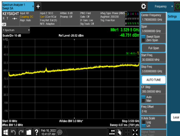
Plot 8-488. Conducted Spurious Emission Plot 30 MHz to 3.53 GHz (LTE_2C+NR_1C_20M+20M+40M_QPSK - low Channel, Port 0)
