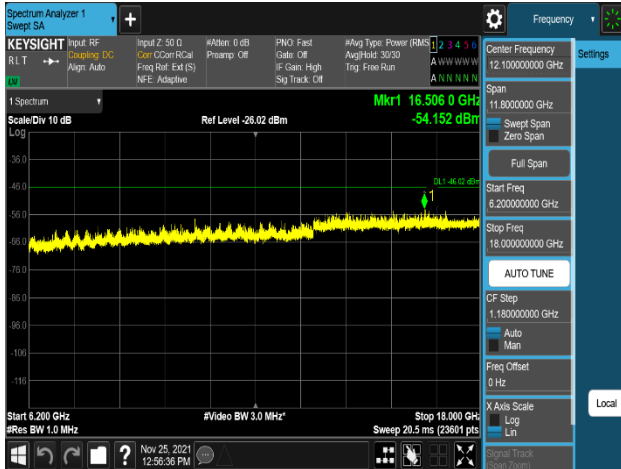
Plot 8-474. Conducted Spurious Emission Plot 6.2 GHz to 18 GHz (NR_n48_1C_40M_QPSK - Low Channel, Port 3)
