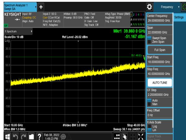
Plot 8-483. Conducted Spurious Emission Plot 18 GHz to 40 GHz (LTE_B48_4C_20M+20M+20M+20M_QPSK - High Channel, Port 0)
