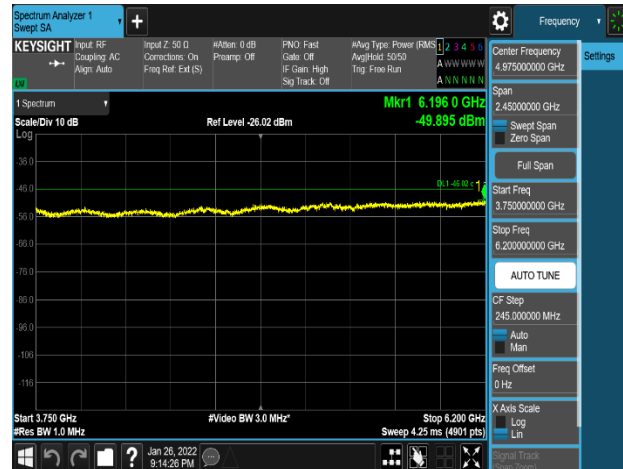
Plot 8-481. Conducted Spurious Emission Plot 3.75 GHz to 6.2 GHz (LTE_B48_4C_20M+20M+20M+20M_QPSK - High Channel, Port 0)
