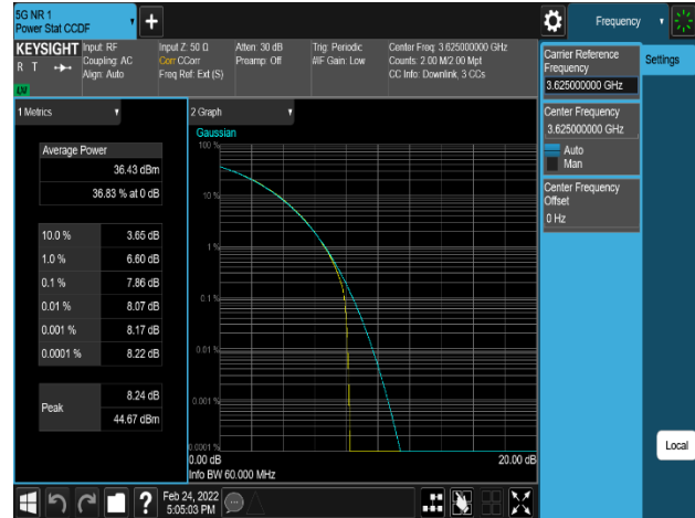
Plot 8-358. Peak To Average Power Ratio Plot (LTE_B48_3C_20M+20M+20M_QPSK - Mid Channel, Port 0)
