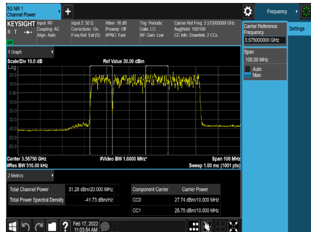
Plot 8-310. Equivalent Isotropic Radiated Power Plot (NR_n48_2C_10M+40M_256QAM - Low Channel, Port 3)
