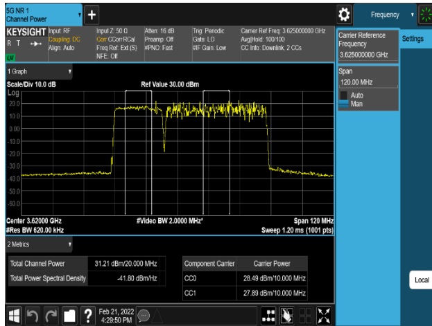
Plot 8-327. Equivalent Isotropic Radiated Power Plot (LTE_1C+NR_1C_20M+40M_16QAM-Mid Channel, Port 0)
