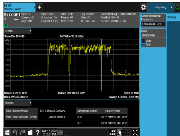
Plot 8-300. Equivalent Isotropic Radiated Power Plot (NR_n48_2C_10M+20M_64QAM - Low Channel, Port 1)
