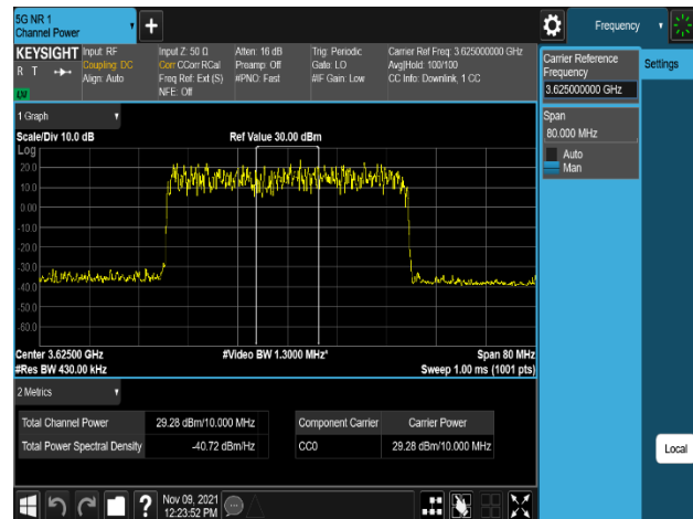
Plot 8-294. Equivalent Isotropic Radiated Power Plot (NR_n48_1C_40M_64QAM - Mid Channel, Port 3)
