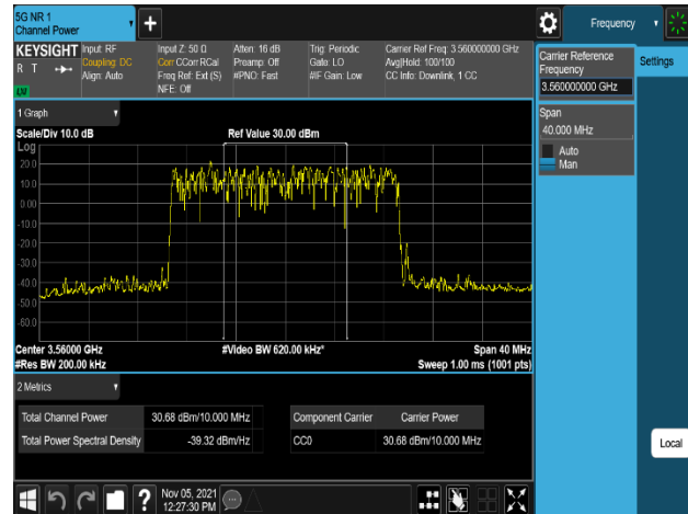
Plot 8-286. Equivalent Isotropic Radiated Power Plot (NR_n48_1C_20M_QPSK - Low Channel, Port 3)
