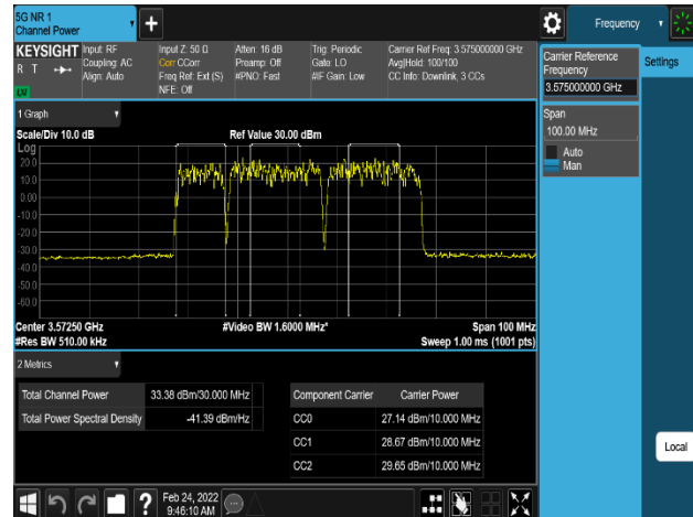
Plot 8-248. Equivalent Isotropic Radiated Power Plot (LTE_B48_3C_10M+20M+20M_64QAM - High Channel, Port 1)
