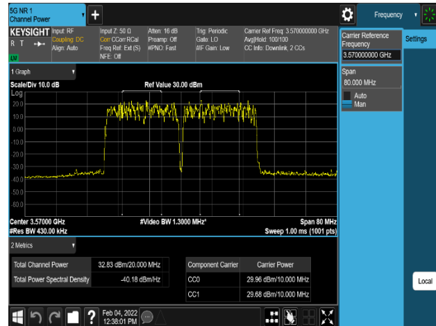
Plot 8-238. Equivalent Isotropic Radiated Power Plot (LTE_B48_2C_20M+20M_QPSK - Low Channel, Port 3)
