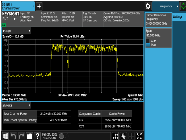
Plot 8-303. Equivalent Isotropic Radiated Power Plot (NR_n48_2C_10M+30M_16QAM - Mid Channel, Port 0)
