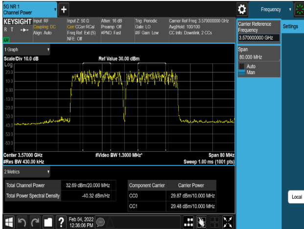
Plot 8-235. Equivalent Isotropic Radiated Power Plot (LTE_B48_2C_20M+20M_QPSK - Low Channel, Port 0)
