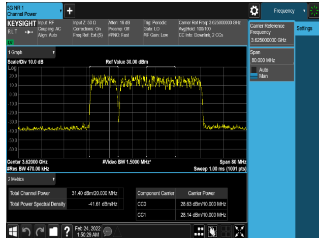
Plot 8-304. Equivalent Isotropic Radiated Power Plot (NR_n48_2C_10M+30M_16QAM - Mid Channel, Port 1)
