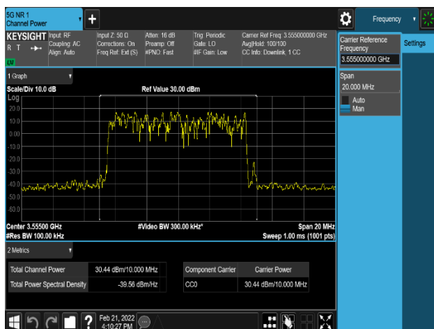
Plot 8-281. Equivalent Isotropic Radiated Power Plot (NR_n48_1C_10M_64QAM - Low Channel, Port 2)
