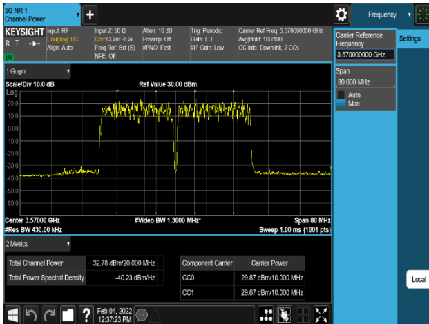
Plot 8-237. Equivalent Isotropic Radiated Power Plot (LTE_B48_2C_20M+20M_QPSK - Low Channel, Port 2)
