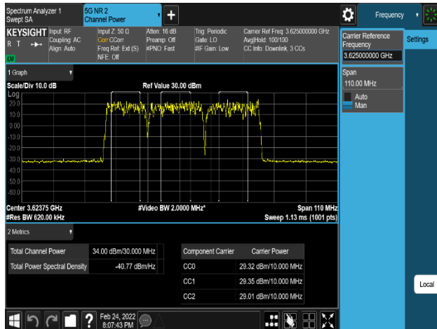
Plot 8-253. Equivalent Isotropic Radiated Power Plot (LTE_B48_3C_15M+20M+20M_QPSK - Mid Channel, Port 2)
