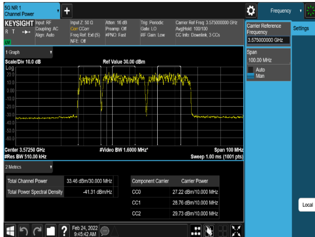
Plot 8-247. Equivalent Isotropic Radiated Power Plot (LTE_B48_3C_10M+20M+20M_64QAM - High Channel, Port 0)
