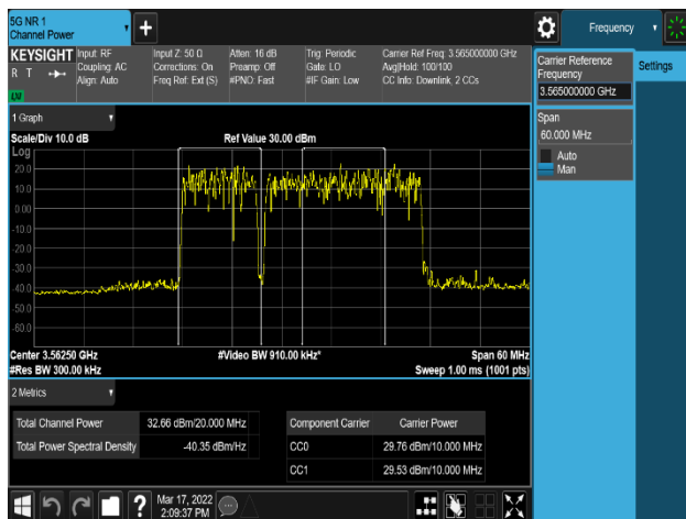
Plot 8-299. Equivalent Isotropic Radiated Power Plot (NR_n48_2C_10M+20M_64QAM - Low Channel, Port 0)
