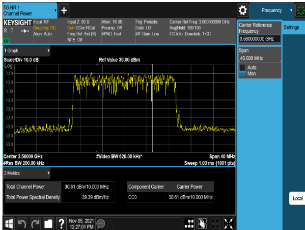
Plot 8-285. Equivalent Isotropic Radiated Power Plot (NR_n48_1C_20M_QPSK - Low Channel, Port 2)
