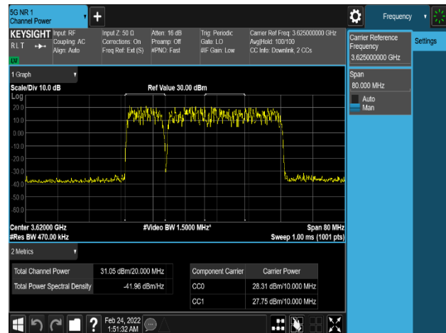
Plot 8-306. Equivalent Isotropic Radiated Power Plot (NR_n48_2C_10M+30M_16QAM - Mid Channel, Port 3)
