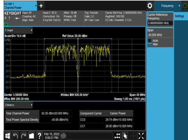
Plot 8-296. Equivalent Isotropic Radiated Power Plot (NR_n48_2C_10M+10M_256QAM - Low Channel, Port 1)
