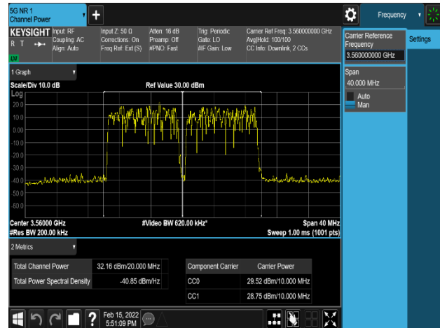
Plot 8-298. Equivalent Isotropic Radiated Power Plot (NR_n48_2C_10M+10M_256QAM - Low Channel, Port 3)
