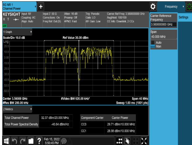
Plot 8-297. Equivalent Isotropic Radiated Power Plot (NR_n48_2C_10M+10M_256QAM - Low Channel, Port 2)
