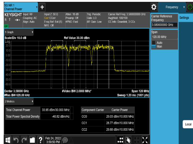
Plot 8-256. Equivalent Isotropic Radiated Power Plot (LTE_B48_3C_20M+20M+20M_QPSK - Low Channel, Port 1)
