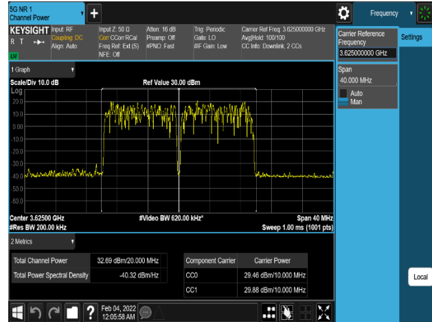
Plot 8-224. Equivalent Isotropic Radiated Power Plot (LTE_B48_2C_10M+10M_64QAM - Mid Channel, Port 1)
