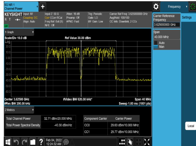
Plot 8-226. Equivalent Isotropic Radiated Power Plot (LTE_B48_2C_10M+10M_64QAM - Mid Channel, Port 3)
