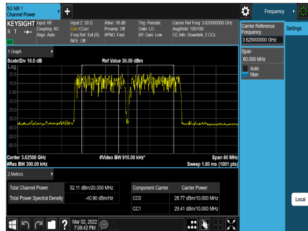
Plot 8-232. Equivalent Isotropic Radiated Power Plot (LTE_B48_2C_15M+15M_256QAM - Mid Channel, Port 1)
