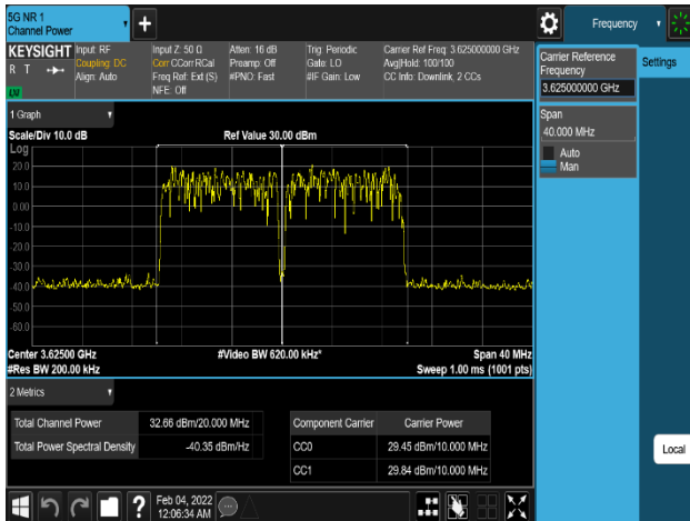
Plot 8-225. Equivalent Isotropic Radiated Power Plot (LTE_B48_2C_10M+10M_64QAM - Mid Channel, Port 2)
