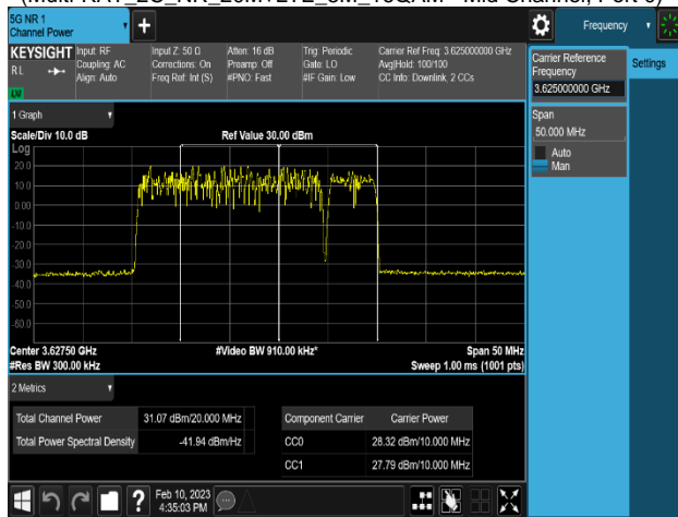
Plot 8-27. Equivalent Isotropic Radiated Power Plot (Multi-RAT_2C_NR_20M+LTE_5M_16QAM - Mid Channel, Port 2)
