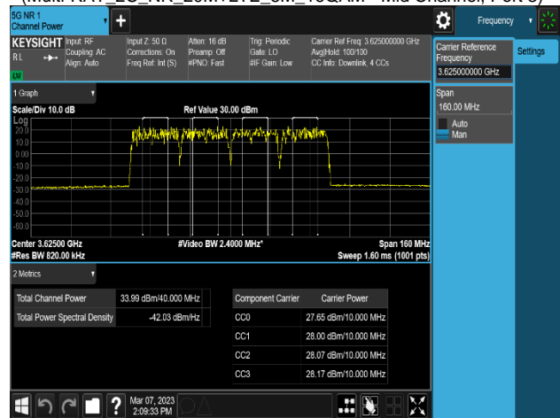
Plot 8-30. Equivalent Isotropic Radiated Power Plot (Multi-RAT_4C_NR_20M+20M+LTE_20M+20M_16QAM - Mid Channel, Port 1)
