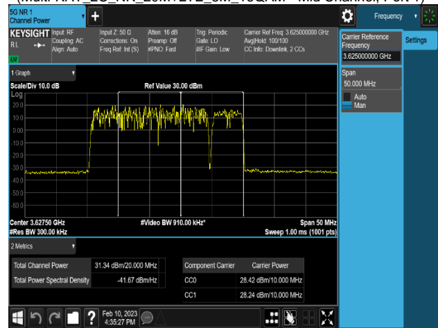
Plot 8-28. Equivalent Isotropic Radiated Power Plot (Multi-RAT_2C_NR_20M+LTE_5M_16QAM - Mid Channel, Port 3)
