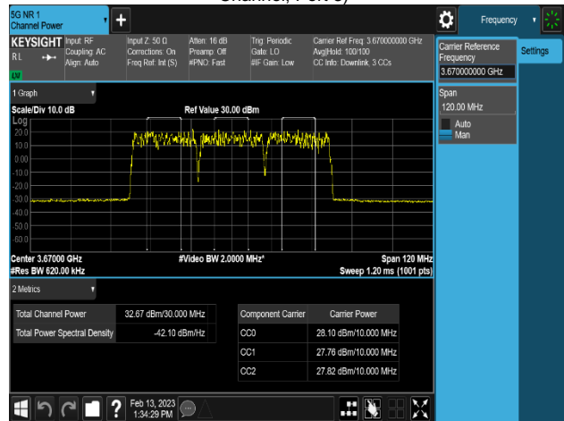
Plot 8-34. Equivalent Isotropic Radiated Power Plot (NR_3C_20M+20M_QPSK - High Channel, Port 1)
