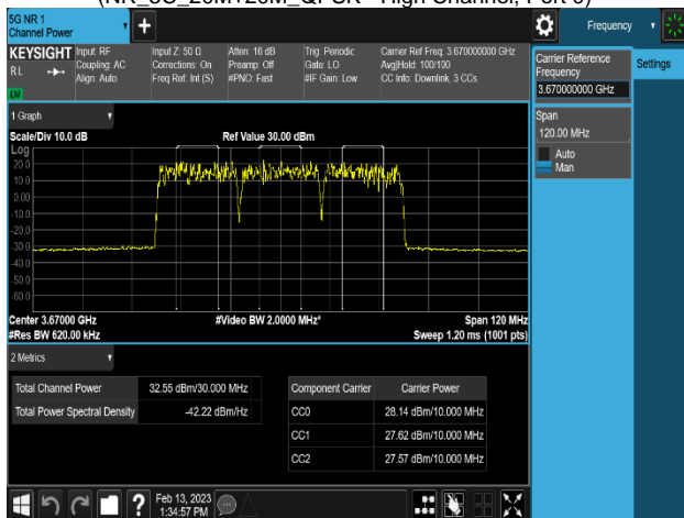
Plot 8-35. Equivalent Isotropic Radiated Power Plot (NR_3C_20M+20M+20M_QPSK - High Channel, Port 2)
