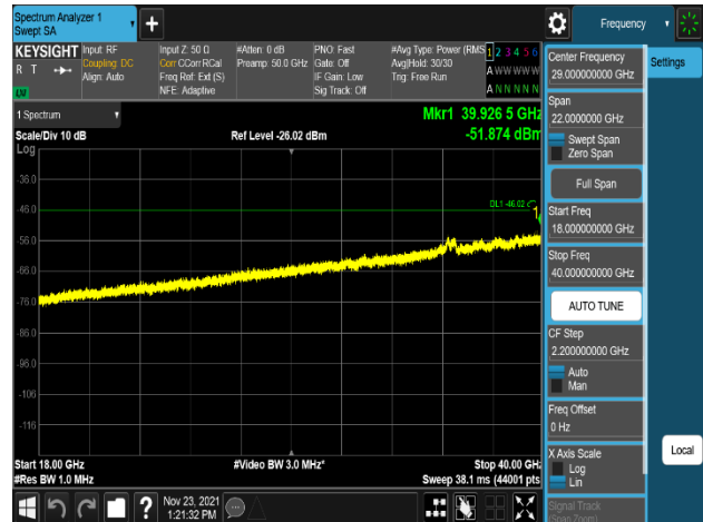
Plot 8-283. Conducted Spurious Emission Plot 18 GHz to 40 GHz (NR_n48_2C_40M+40M_Non-Contiguous_16QAM- Mid Channel, Port 0)
