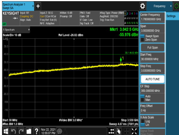
Plot 8-276. Conducted Spurious Emission Plot 30 MHz to 3530 MHz (NR_n48_2C_40M+40M_64QAM - Mid Channel, Port 0)
