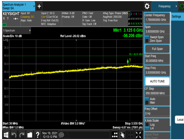
Plot 8-256. Conducted Spurious Emission Plot 30 MHz to 3530 MHz (NR_n48_1C_10M_16QAM - High Channel, Port 2)
