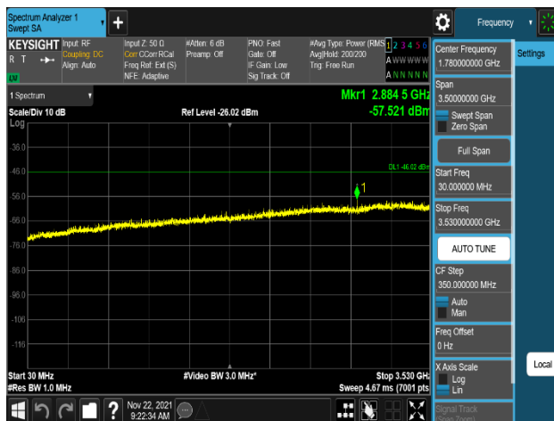
Plot 8-260. Conducted Spurious Emission Plot 30 MHz to 3530 MHz (NR_n48_1C_20M_16QAM - Low Channel, Port 3)
