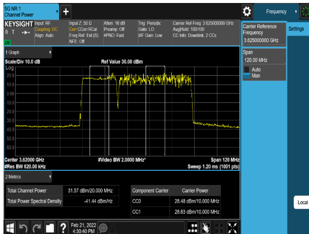
Plot 8-173. Equivalent Isotropic Radiated Power Plot (LTE_1C+NR_1C_20M+40M_QPSK - High Channel, Port 2)
