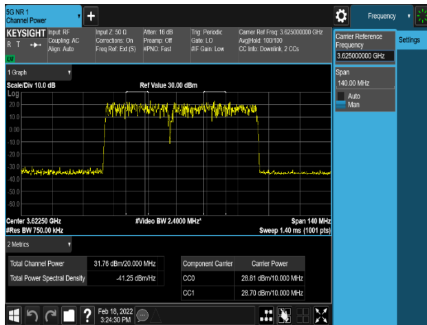
Plot 8-161. Equivalent Isotropic Radiated Power Plot (NR_n48_2C_30M+40M_QPSK – Mid Channel, Port 2)
