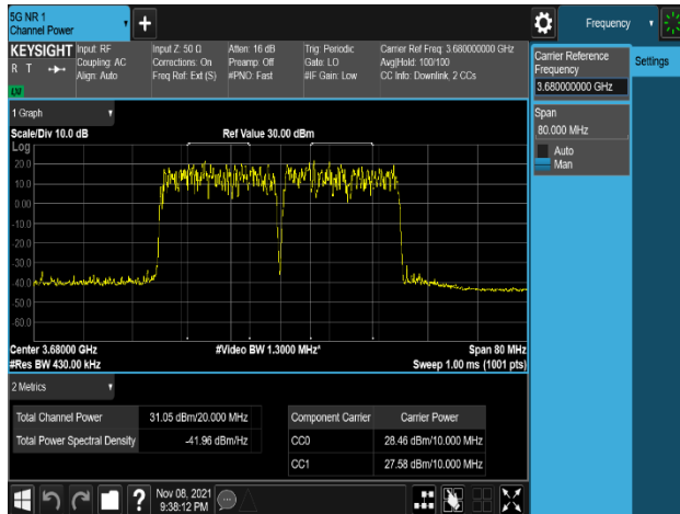
Plot 8-147. Equivalent Isotropic Radiated Power Plot (NR_n48_2C_20M+20M_64QAM – High Channel, Port 0)
