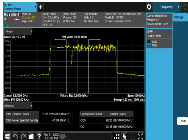
Plot 8-174. Equivalent Isotropic Radiated Power Plot (LTE_1C+NR_1C_20M+40M_QPSK - High Channel, Port 3)
