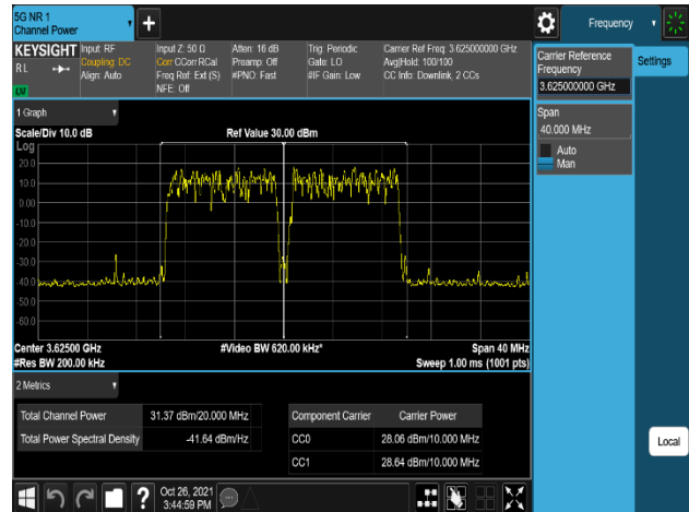
Plot 8-136. Equivalent Isotropic Radiated Power Plot (NR_n48_2C_10M+10M_QPSK – Mid Channel, Port 1)
