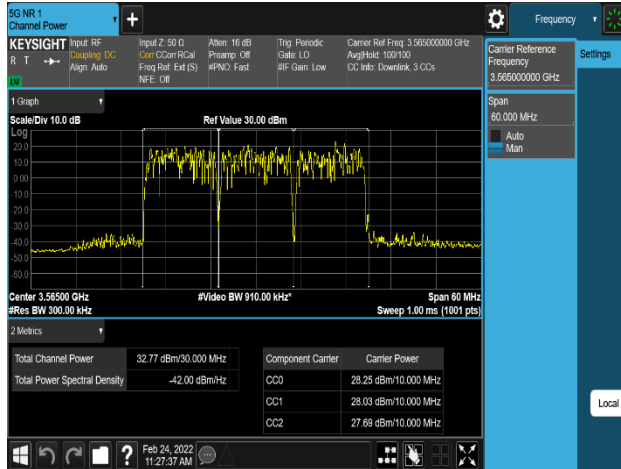
Plot 8-175. Equivalent Isotropic Radiated Power Plot (LTE_2C+NR_1C_10M+10M+10M_64QAM-Low Channel, Port 0)
