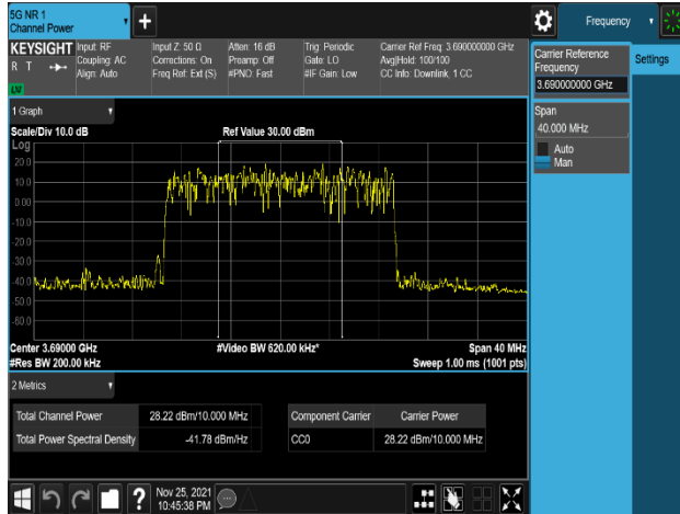
Plot 8-121. Equivalent Isotropic Radiated Power Plot (NR_n48_1C_20M_16QAM – High Channel, Port 2)
