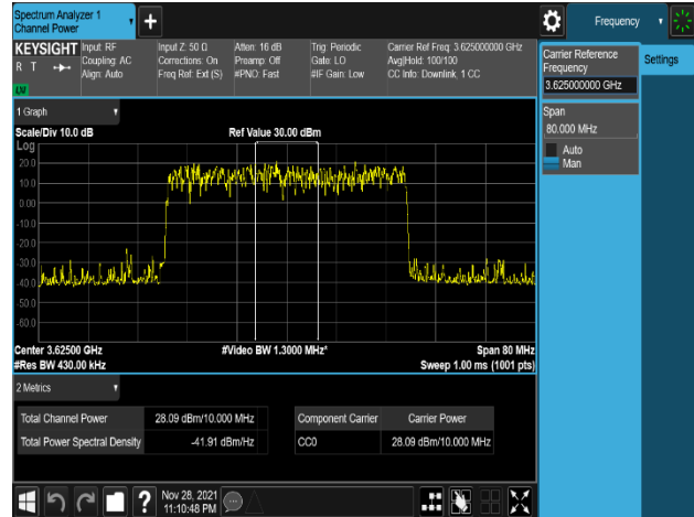
Plot 8-128. Equivalent Isotropic Radiated Power Plot (NR_n48_1C_40M_16QAM – Mid Channel, Port 1)
