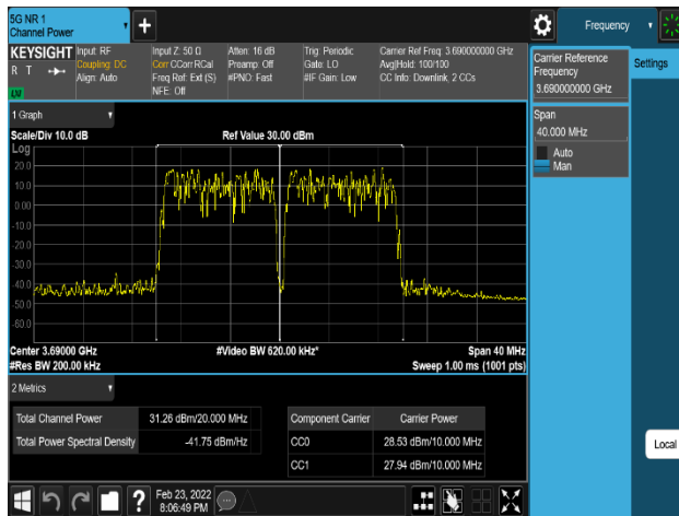
Plot 8-167. Equivalent Isotropic Radiated Power Plot (LTE_1C+NR_1C_10M+10M_QPSK - High Channel, Port 0)
