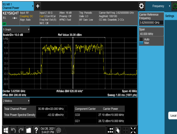
Plot 8-135. Equivalent Isotropic Radiated Power Plot (NR_n48_2C_10M+10M_QPSK – Mid Channel, Port 0)
