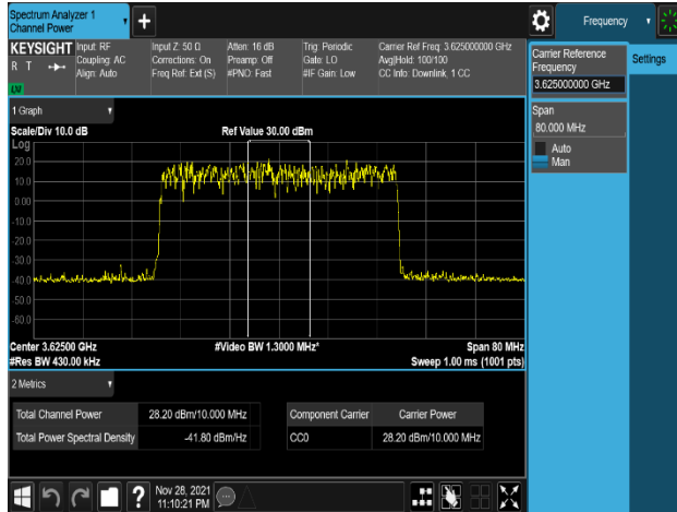
Plot 8-127. Equivalent Isotropic Radiated Power Plot (NR_n48_1C_40M_16QAM – Mid Channel, Port 0)
