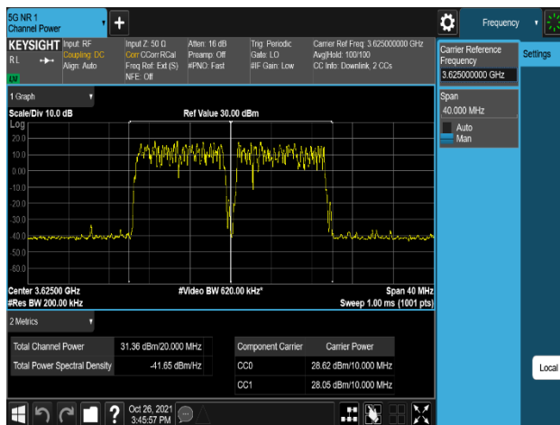
Plot 8-137. Equivalent Isotropic Radiated Power Plot (NR_n48_2C_10M+10M_QPSK – Mid Channel, Port 2)
