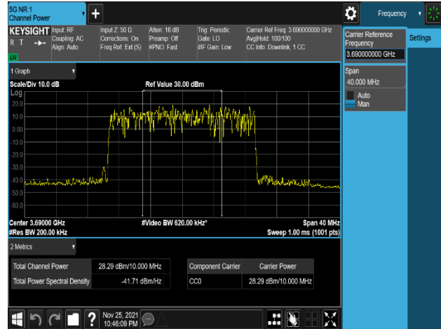
Plot 8-122. Equivalent Isotropic Radiated Power Plot (NR_n48_1C_20M_16QAM – High Channel, Port 3)
