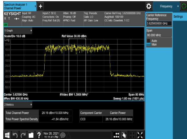
Plot 8-130. Equivalent Isotropic Radiated Power Plot (NR_n48_1C_40M_16QAM – Mid Channel, Port 3)
