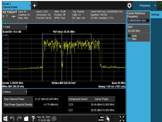
Plot 8-141. Equivalent Isotropic Radiated Power Plot (NR_n48_2C_10M+20M_16QAM – Low Channel, Port 2)
